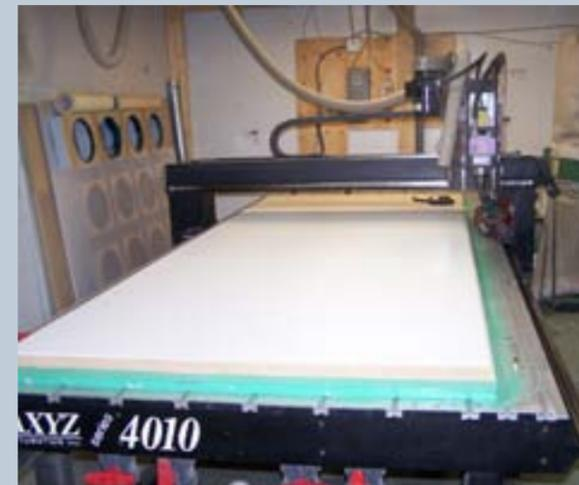
Figure 64: XYZ Programmable Router.
