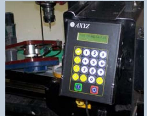
Figure 65: Router programming terminal.
