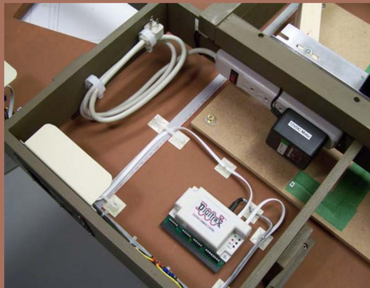
Figure 9: Electrical, DCC and electronic parts.
