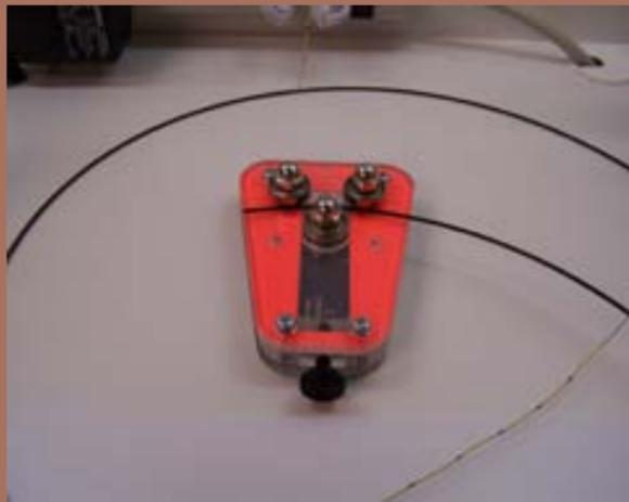
Figure 43: Fast Tracks Rail Bender.
