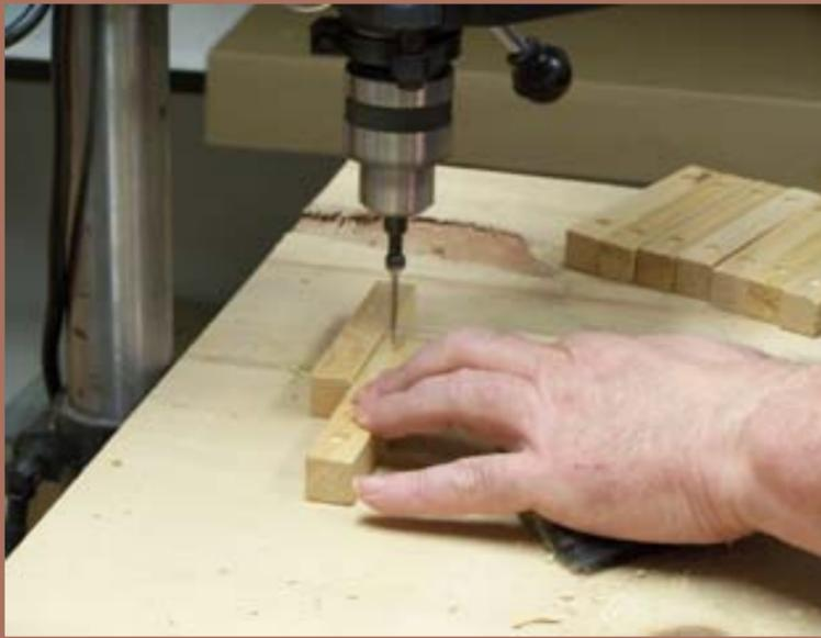
Figure 21: Pre-drilling the cleats.
