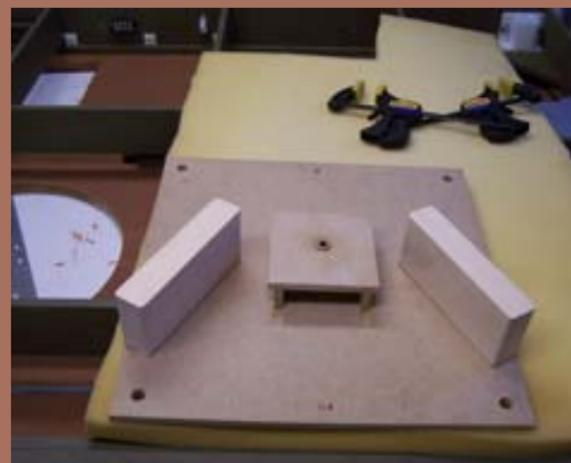
Figure 76: Pit bottom with mounting blocks.
