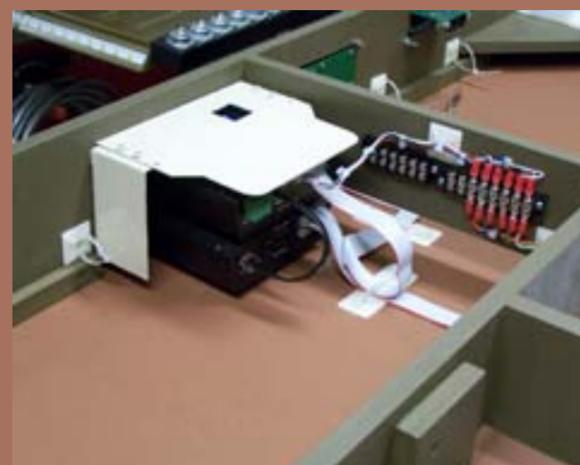
Figure 93: PTC III and APR mounted with Velcro inverted view with protective cover installed.
