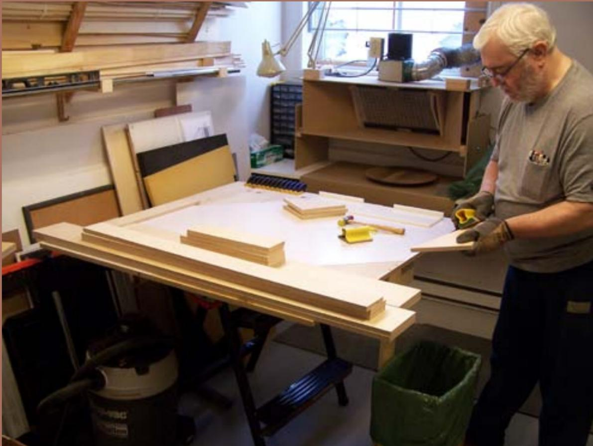
Figure 11: Preparing / Sanding rough edges.
