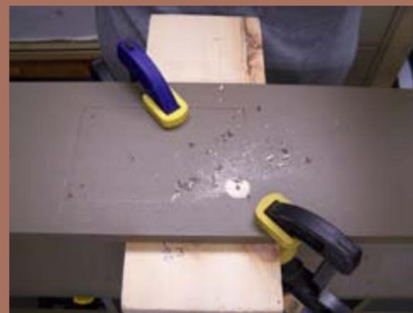
Figure 34: Used a backplate to help get a clean cut.
