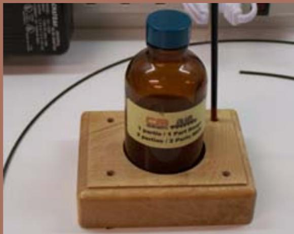
Figure 47: Barge cement and MEK mixture
