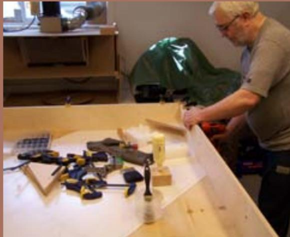
Figure 13: Assembling sideframe and gusset.
