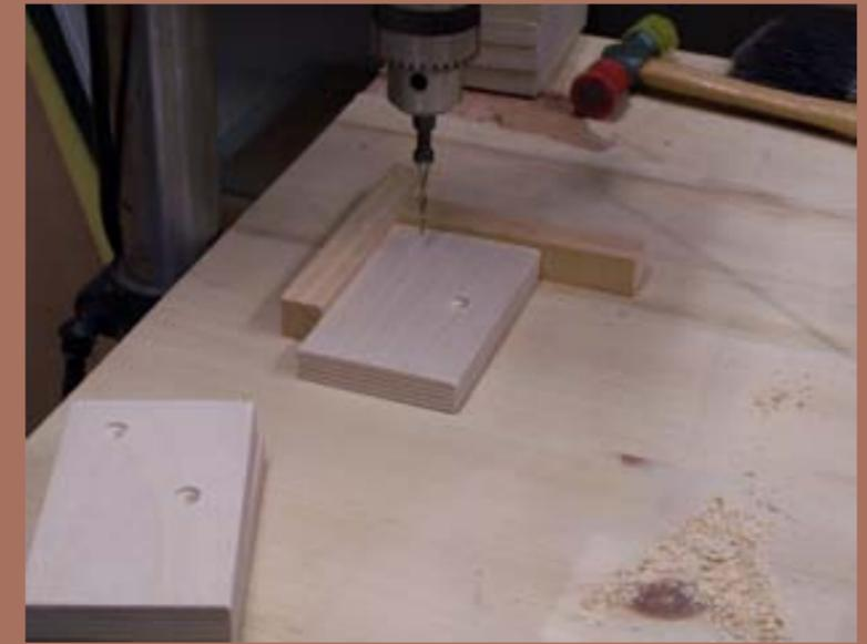
Figure 23: Pre-drilling the risers.
