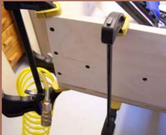
Figure 15: Sideframe and gusset screw positions.
