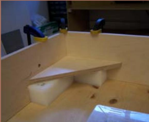
Figure 14: Gussets glued and screwed.
