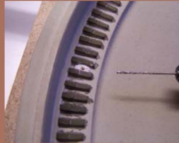
Figure 45: Drill hole in pit for wire.
