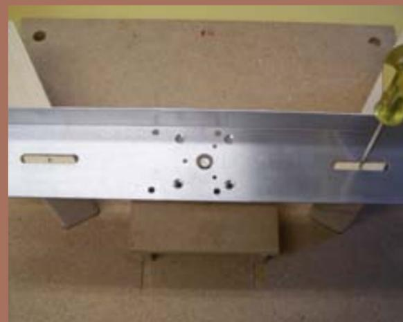
Figure 78: Centering mounting bracket.
