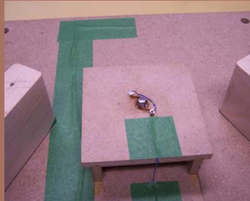
Figure 61: Dual wipers on shaft for better continuity.
