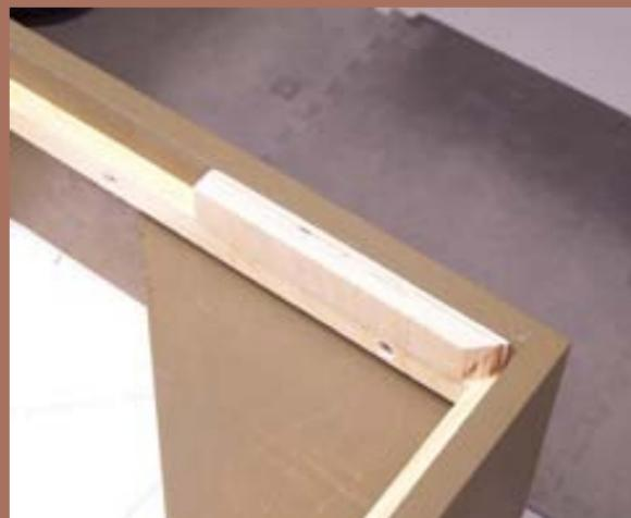
Figure 27: Sideframe cleats installed.
