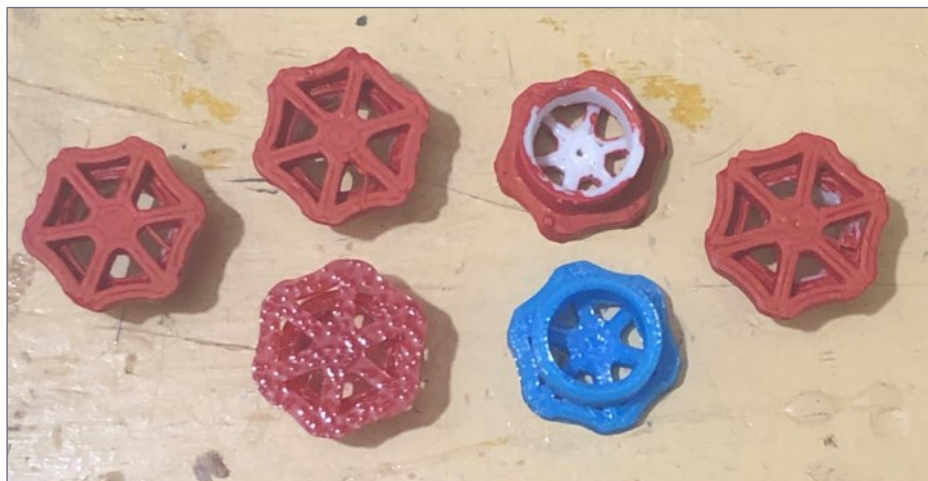
2. Pushbutton Tops/Appliques. The top four are printed with PLA, and painted. The bottom two are PETG.
