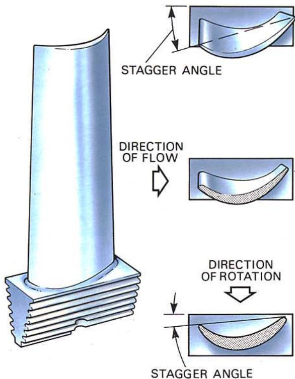
**Fig. 5-6 A typical turbine blade showing twisted contour.**
