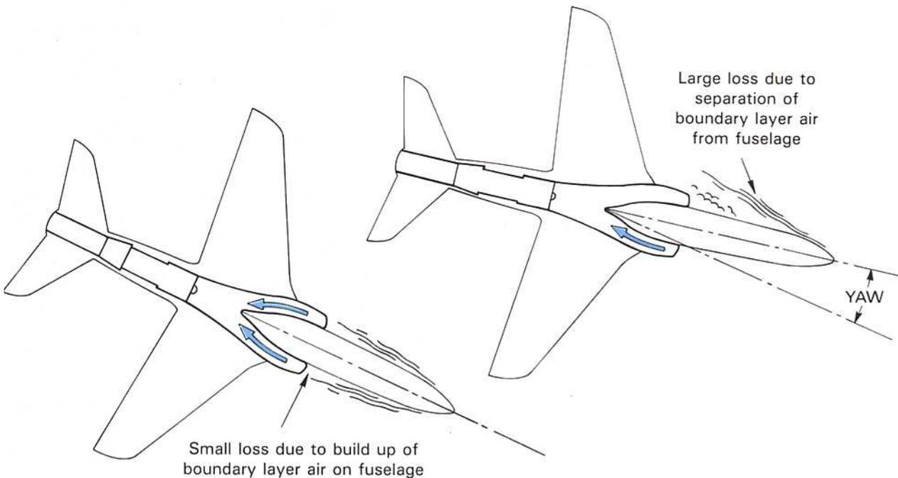
**Fig. 23-7 Loss of ram pressure in divided intakes.**
