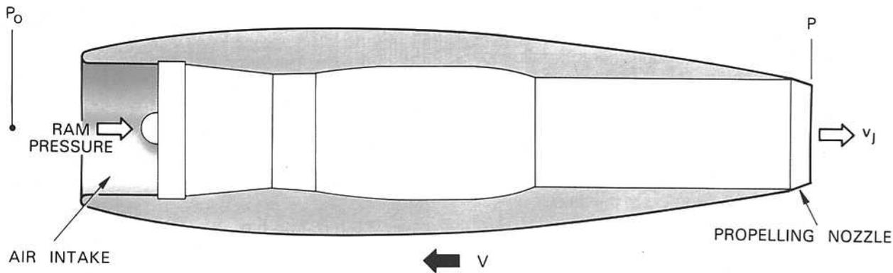
All pressures are total pressures except P which is the static pressure at the propelling nozzle
