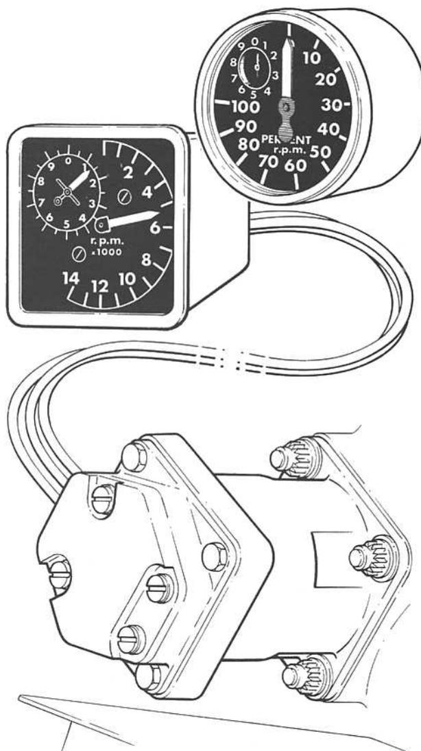
**Fig. 12-5 Engine speed indicators and generator.**
