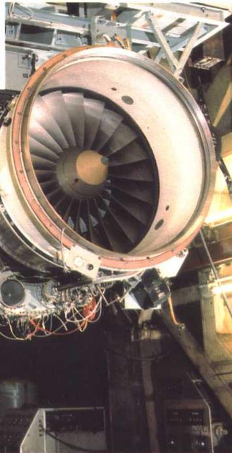
Fig. 25-14 A sea-level test cell.
