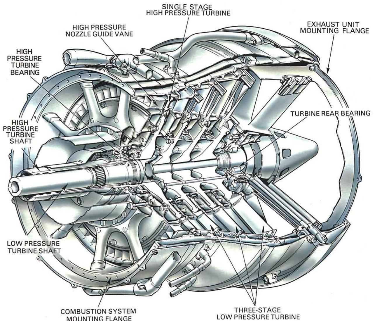
Fig. 5-2 A twin turbine and shaft arrangement.
