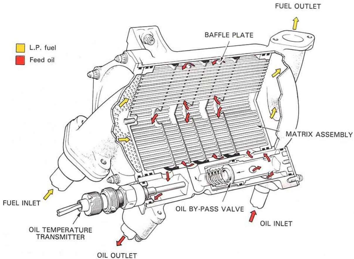
**Fig. 8-7** A low pressure fuel-cooled oil cooler.
