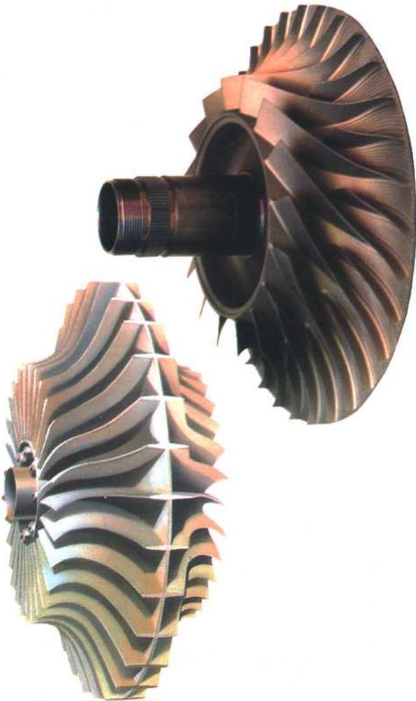
**Fig. 3-5 Typical impellers for centrifugal compressors.**
