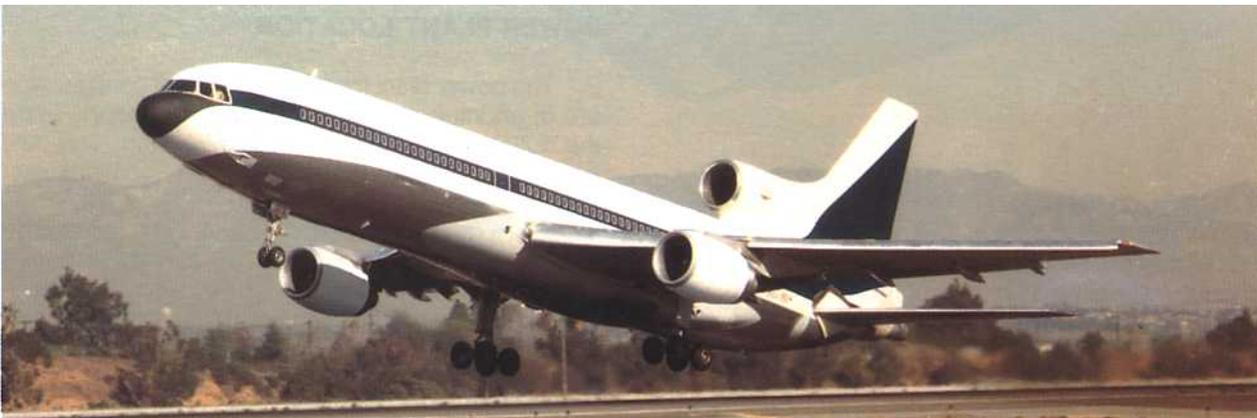
**Fig. 23-3** Tail and wing-mounted pod installation.
