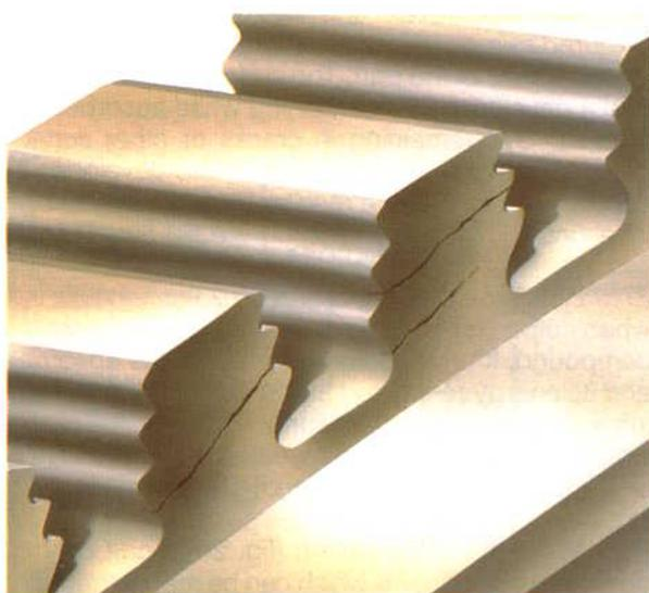
**Fig. 25-4 Cracks revealed by magnetic crack detection.**
