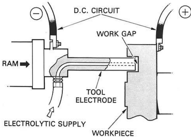
1. Electrolytic solution passes under pressure through tool electrode
