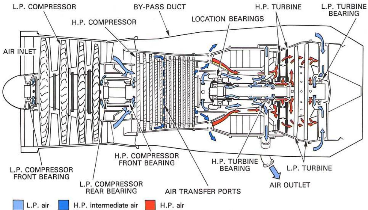
Fig. 9-1 General internal airflow pattern.
