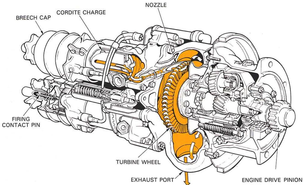
**Fig. 11-4 A triple-breech cartridge starter.**
