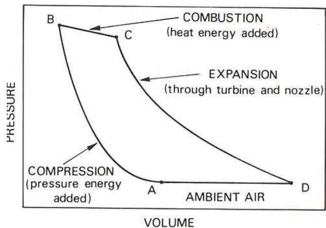
**Fig. 2-2 The working cycle on a pressure-volume diagram.**
