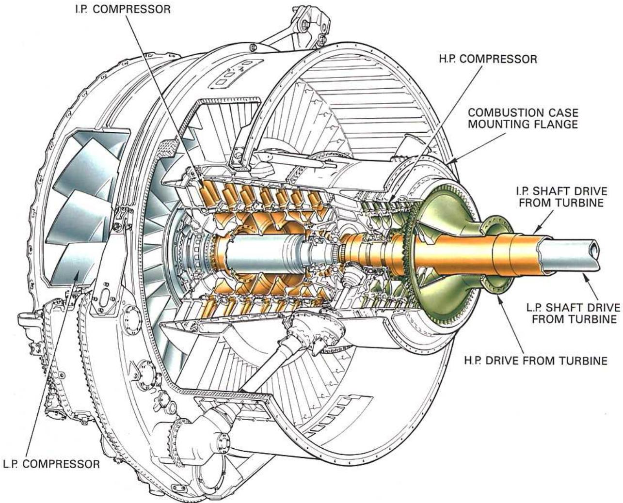
**Fig. 3-8 Typical triple spool compressor.**
