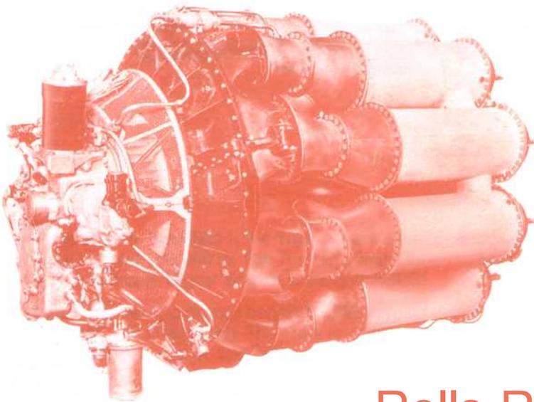
On 1 April, 1943, Rolls-Royce assumed responsibility for the Power Jets W2B which, a month earlier, had made its first flight in the Gloster E28/39 at 1200lb thrust. Later known as the B23 Welland it was, during April, put through a 100 hr test at the design rating of 1600 lb thrust. In June, 1943, it flew in a Gloster Meteor at 1400lb thrust. Production Welland-Meteors were in action against V-1 flying bombs in August 1944.
