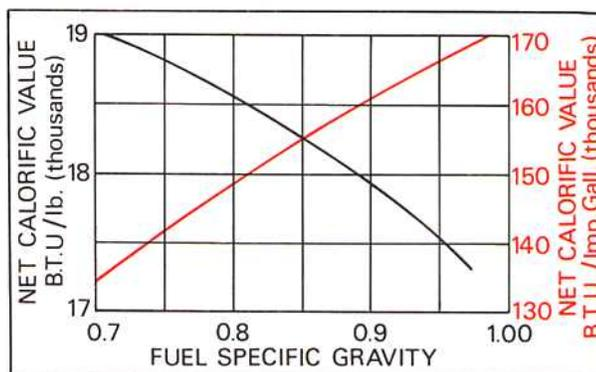
**Fig. 10-21 Relationship between calorific value and specific gravity.**
