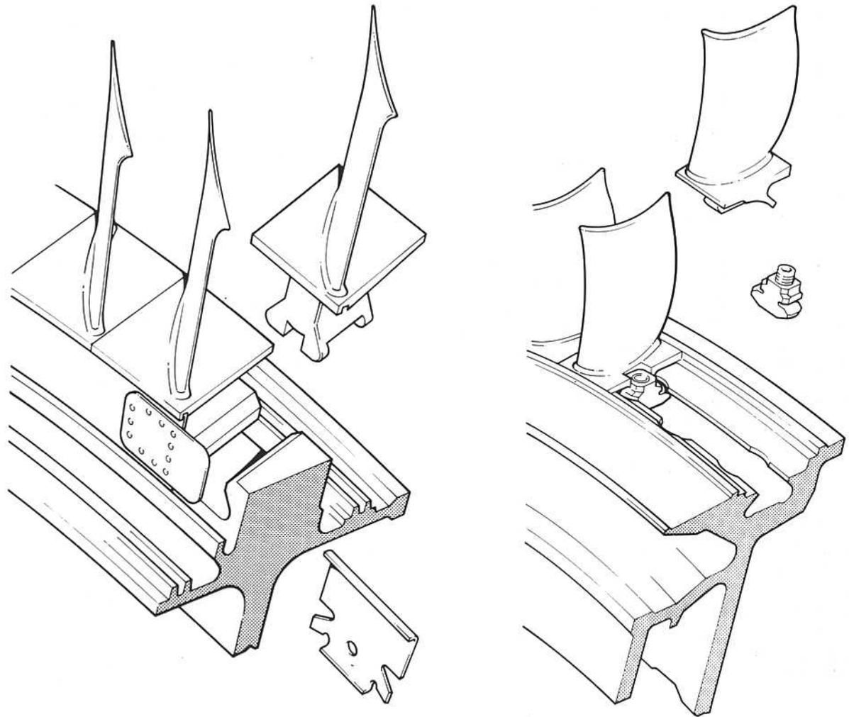
**Fig. 3-11 Methods of securing blades to disc.**
