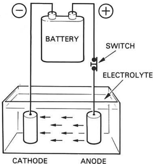
Fig. 22-11 Electro-chemical machining.
