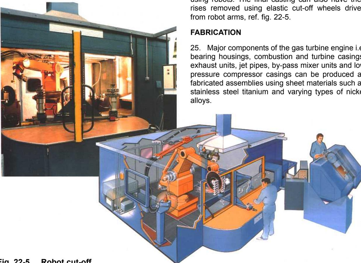
Fig. 22-5 Robot cut-off
