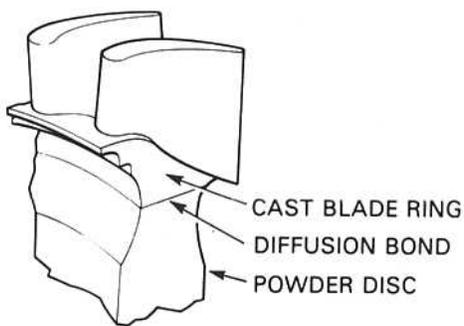
**Fig. 5-11 Section through a dual alloy disc.**
