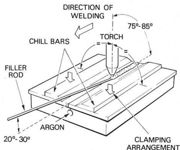
**Fig. 22-7** Typical tungsten inert gas welding details.
