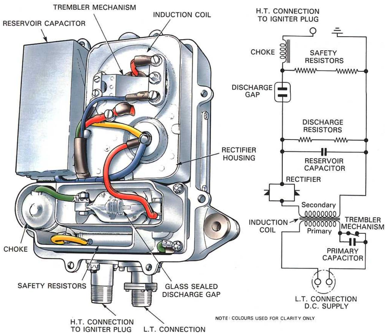
Fig. 11-10 A D.C. trembler-operated ignition unit.
