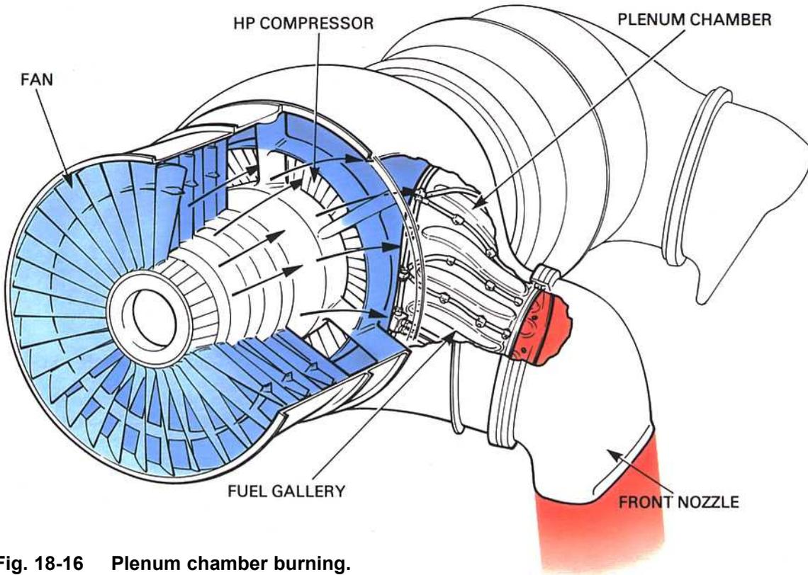
Fig. 18-16 Plenum chamber burning.
