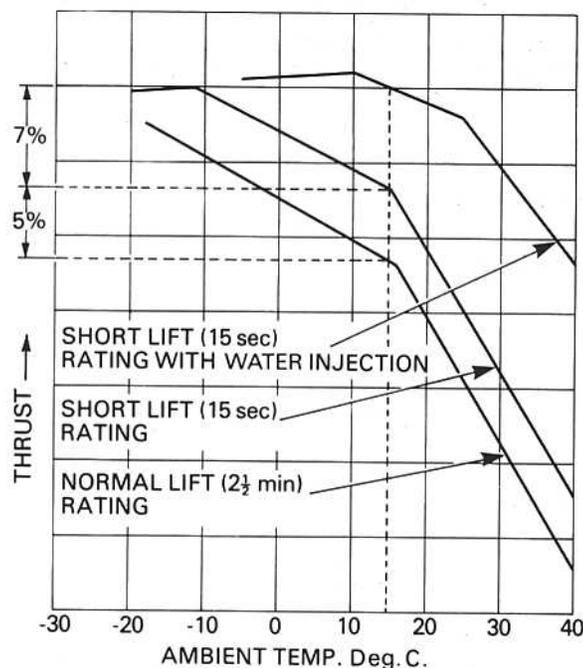
**Fig. 18-15 Thrust increases with short lift ratings.**
