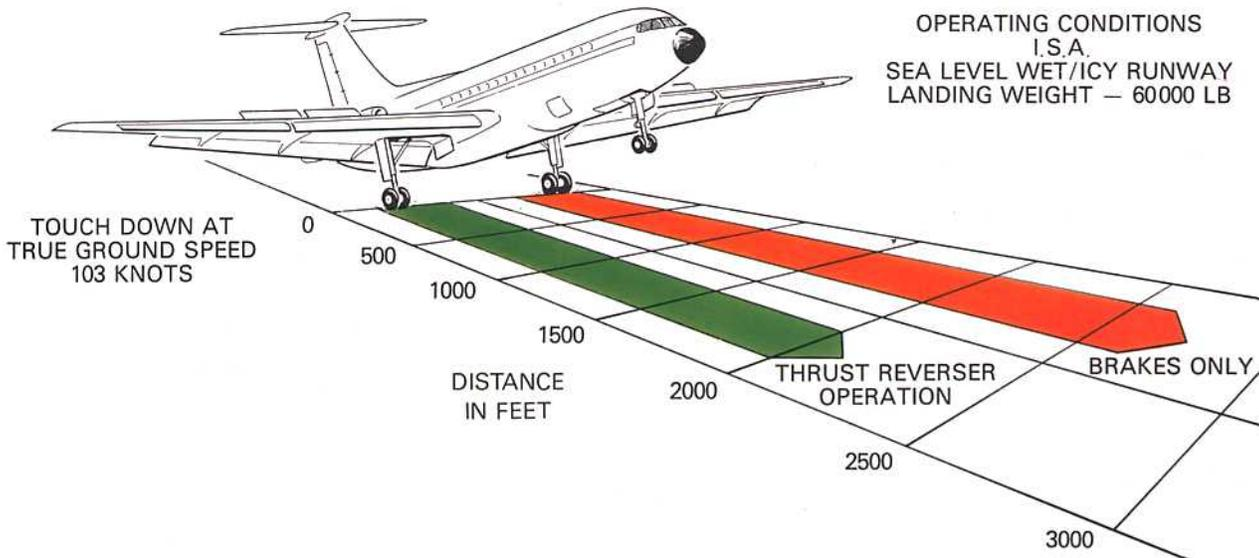
**Fig. 15-1 Comparative landing runs with and without thrust reversal.**
