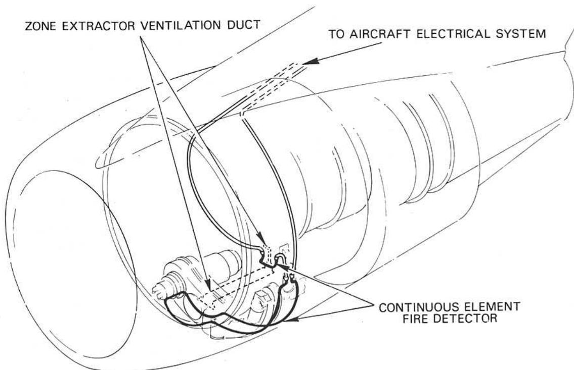
**Fig. 14-3** A continuous element fire detecting system.
