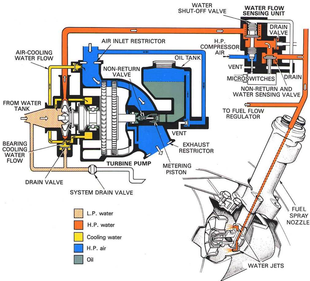
**Fig. 17-4 A typical combustion chamber injection system.**
