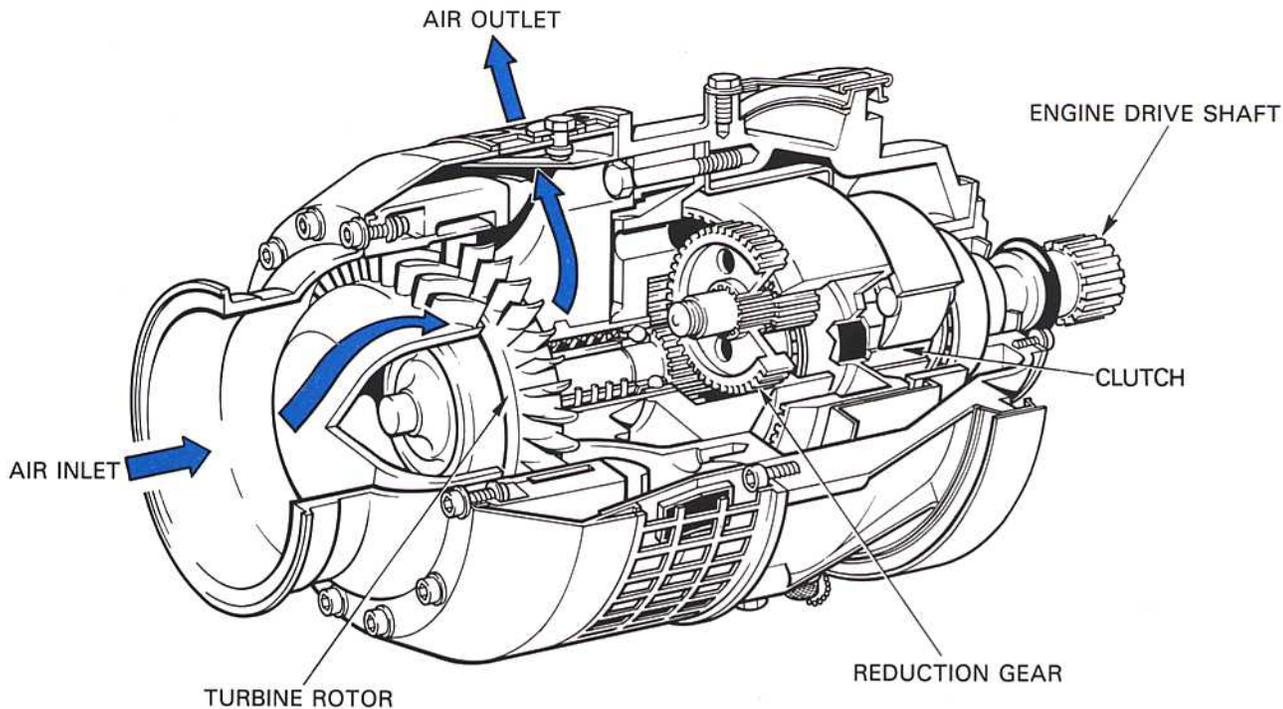
**Fig. 11-6 An air starter motor.**
