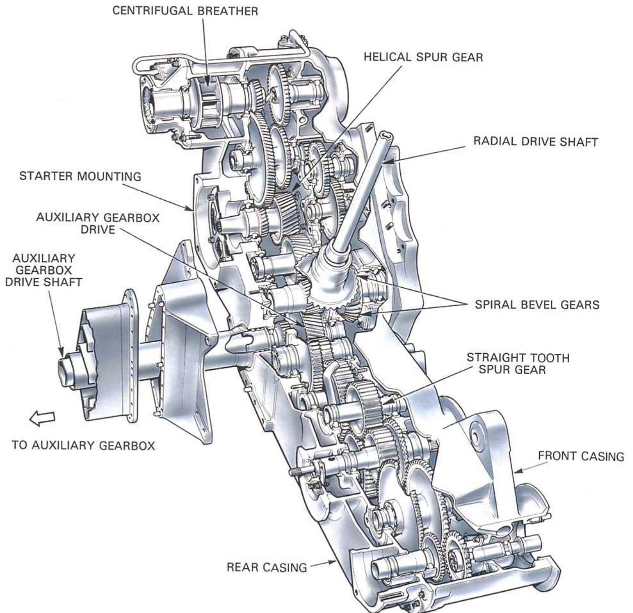
**Fig. 7-5 An external gearbox with auxiliary gearbox drive.**
