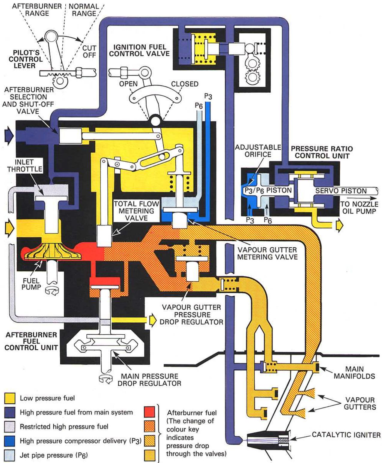
Fig. 16-6 A simplified typical afterburner fuel control system.
