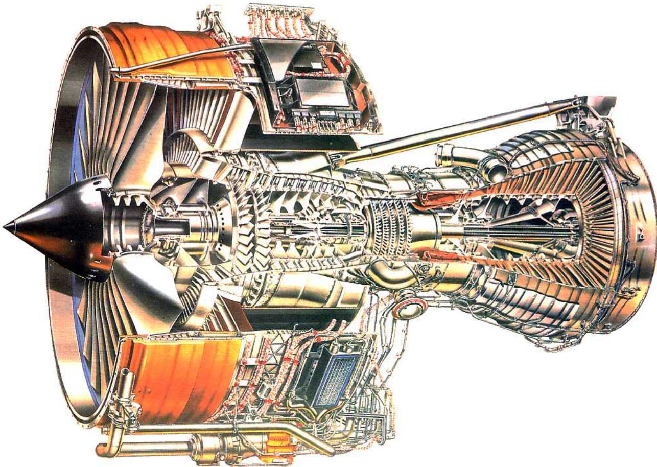
Developed from the RB211, the Trent covers a thrust range of 71,000 lb to 92,000 lb thrust, with the capability to grow beyond 100,000 lb. The Trent 800 features a 110 inch diameter wide-chord fan, high flow compressors and Full Authority Digital Engine Control (FADEC).
