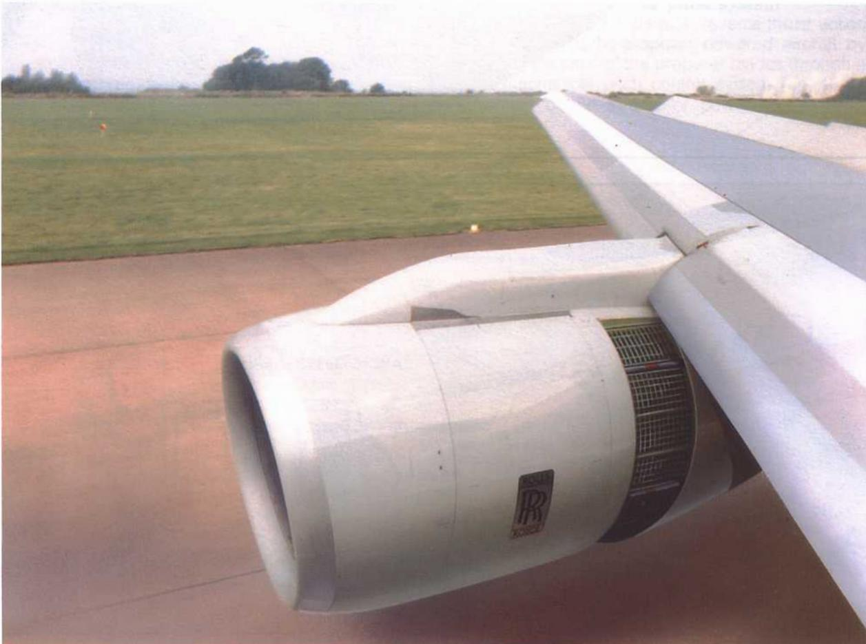
**Fig. 15-7 A cold stream thrust reverser installation.**
