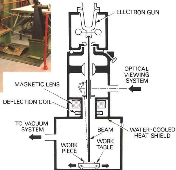
**Fig. 22-9 Electron beam welding.**
