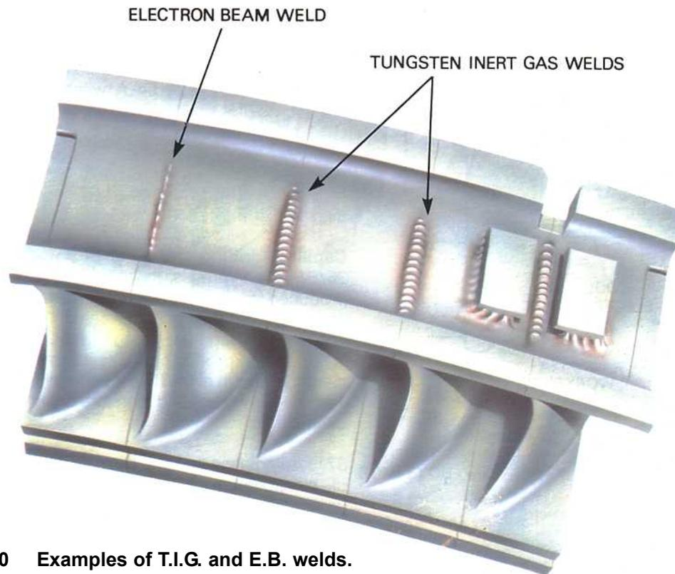
**Fig. 22-10 Examples of T.I.G. and E.B. welds.**
