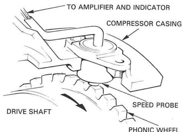
**Fig. 12-6 Variable-reluctance speed probe and phonic wheel.**
