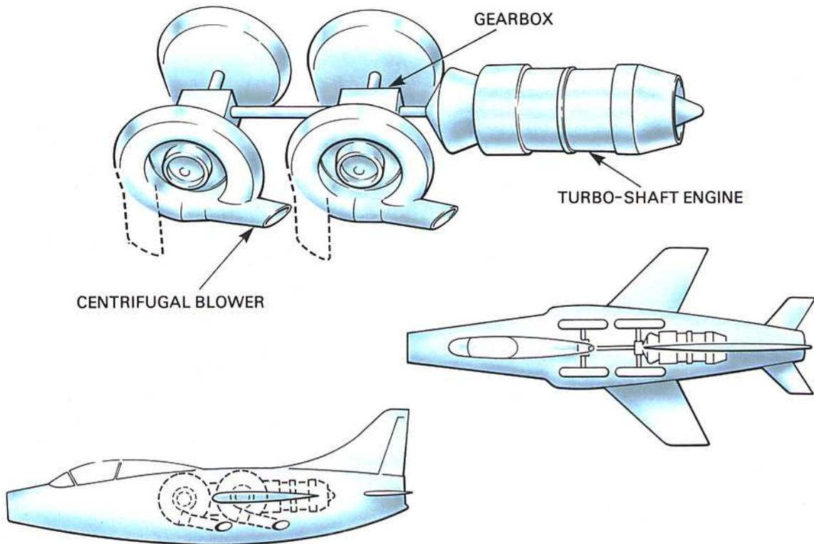
**Fig. 18-1 Michel Wibault's ground attack gyropter (concept) 1956**
