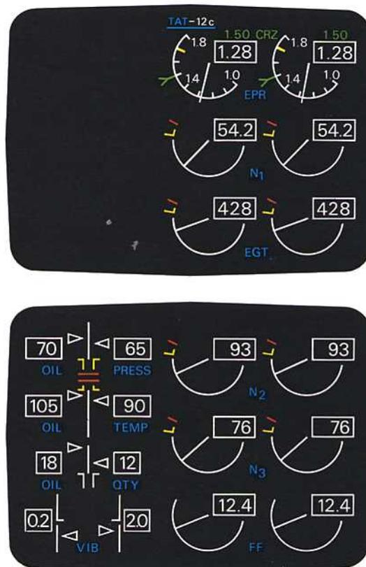
**Fig. 12-12** Typical electronic indicating display.
