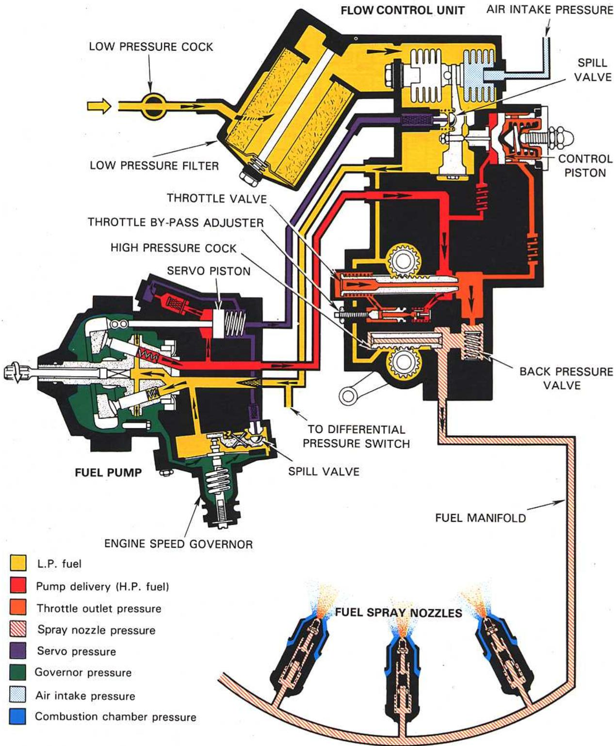
Fig. 10-4 A pressure control system (turbo-propeller engine).
