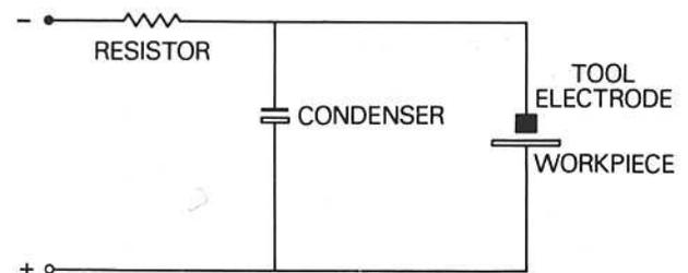
**Fig. 22-13 Electro-discharge machining circuit.**
