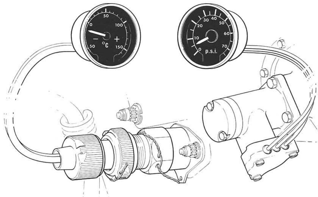
**Fig. 12-9 Oil temperature and pressure transmitters and indicators.**
