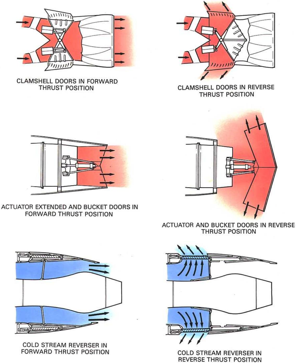
Fig. 15-2 Methods of thrust reversal.
