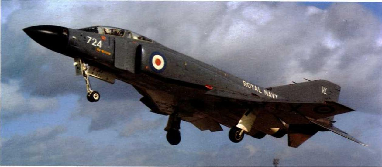
Fig. 23-10 Fuselage intakes.
