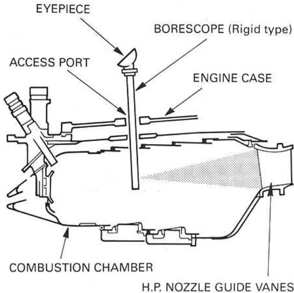
**Fig. 24-2 Inspection of H.P. nozzle guide vanes.**
