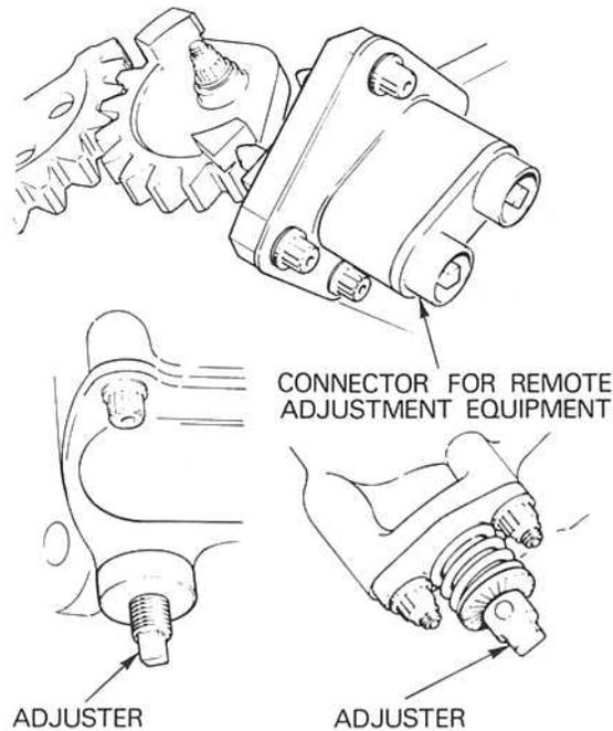
**Fig. 24-5 Typical friction locked adjusters.**
