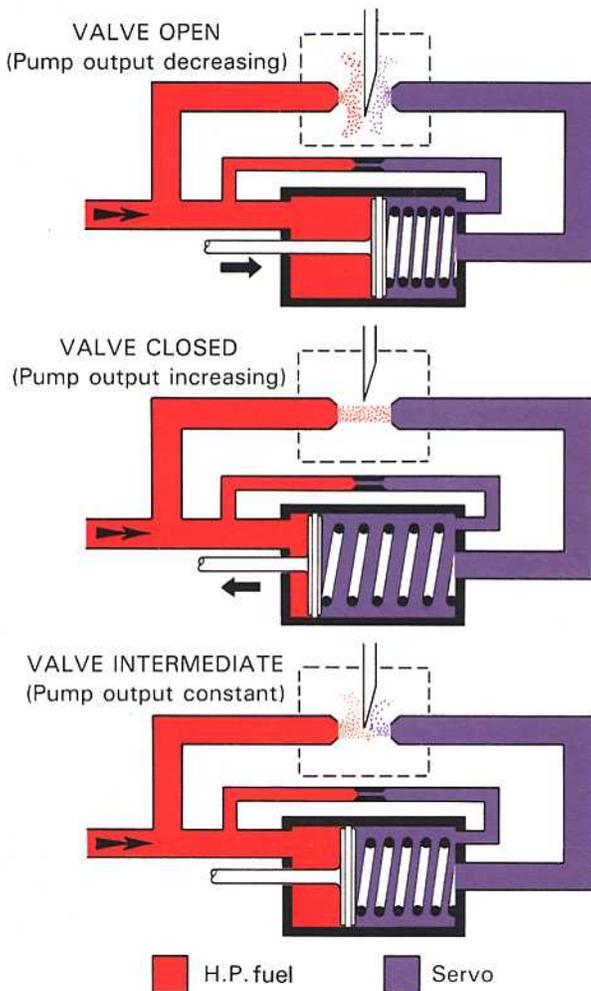
**Fig. 10-8 Servo pressure control by kinetic valve.**
