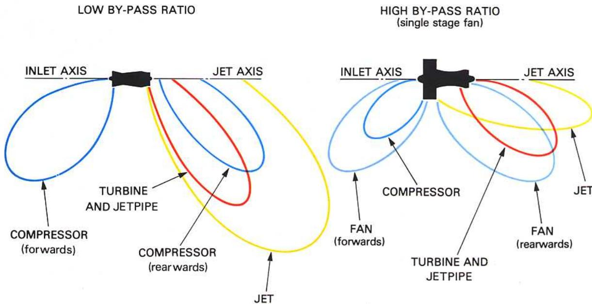
Fig. 19-4 Comparative noise sources of low and high by-pass engines.
