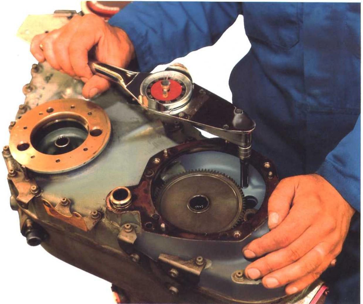
**Fig. 25-12 Torque tightening.**
