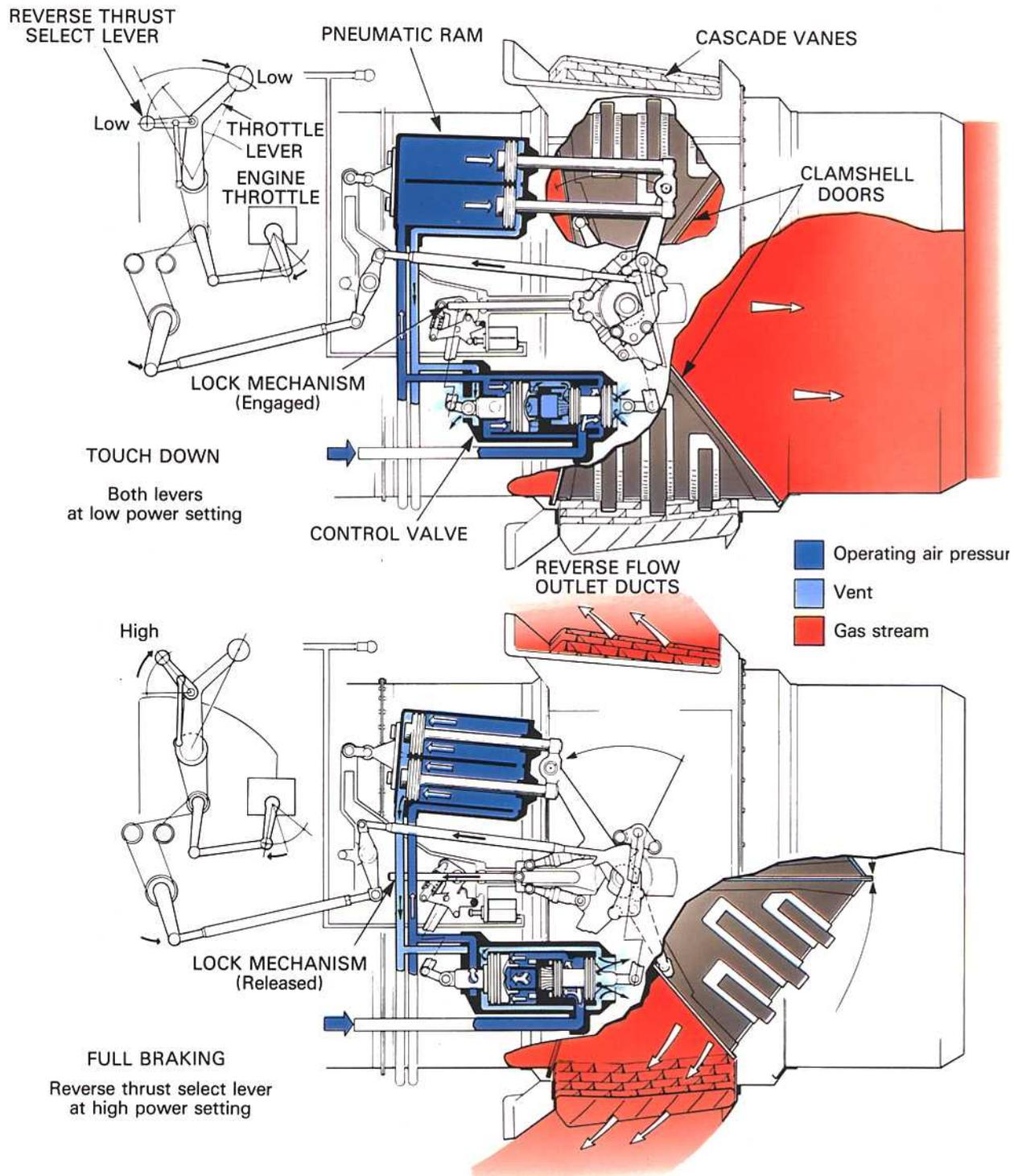
Fig. 15-3 A typical thrust reverser system using clamshell doors.
