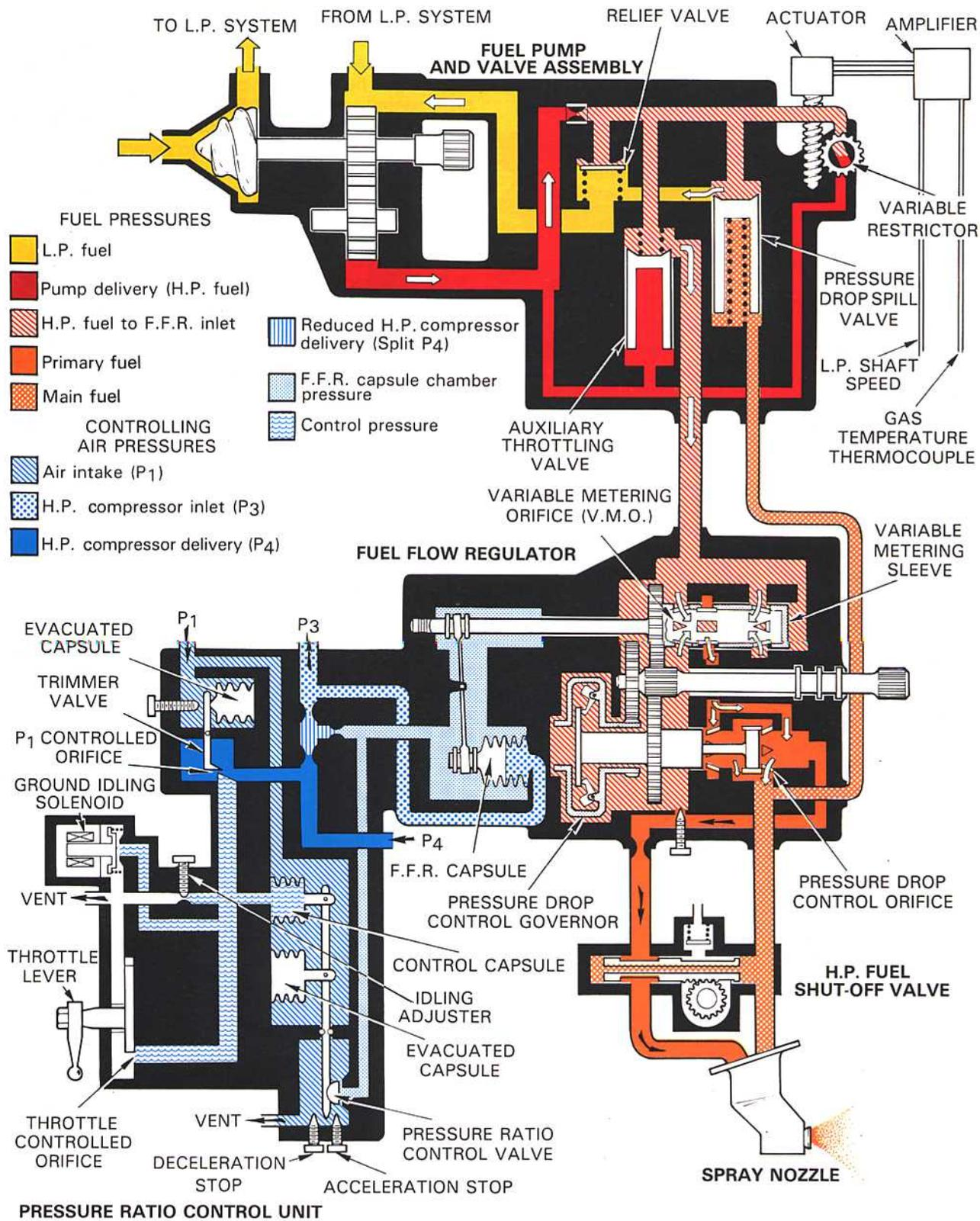
Fig. 10-12 A pressure ratio control system.
