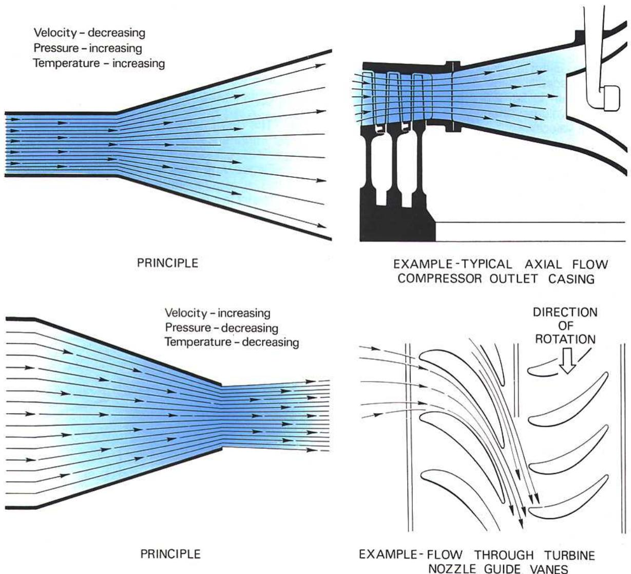
Fig. 2-3 An airflow through divergent and convergent ducts.
