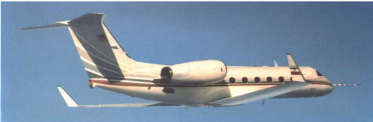
**Fig. 23-2** Fuselage - mounted pod installation.
