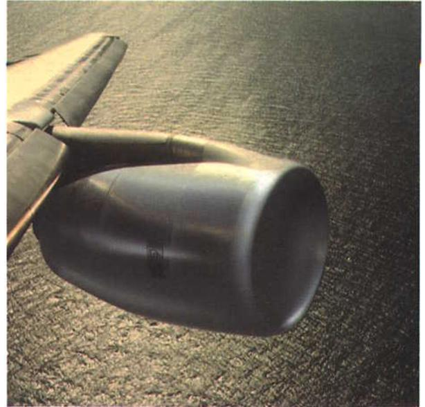
**Fig. 23-4 Pitot-type intake.**
