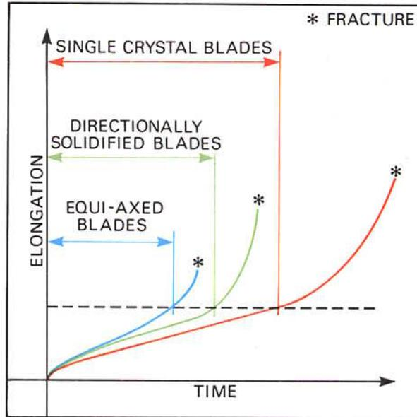
**Fig. 5-13 Comparison of turbine blade life properties.**
