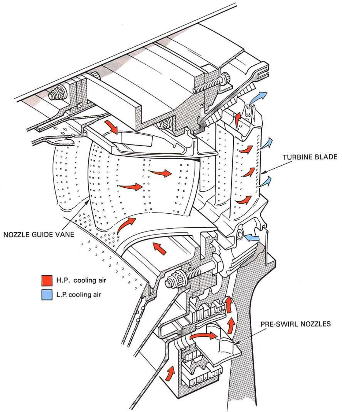
Fig. 9-2 Nozzle guide vane and turbine blade cooling arrangement.
