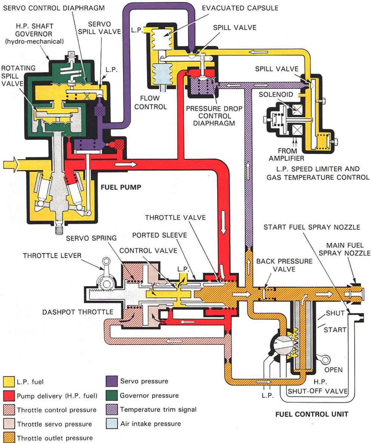
Fig. 10-5 A pressure control system (turbo-jet engine).
