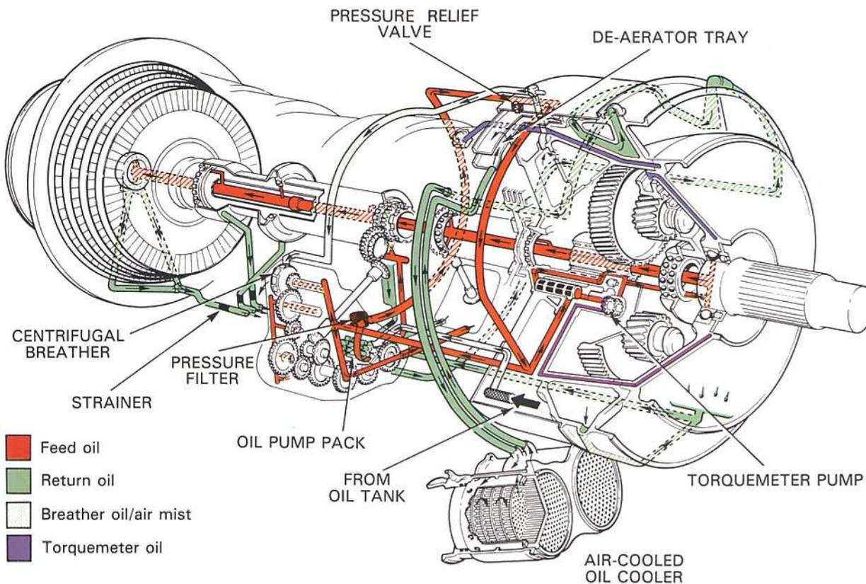
Fig. 8-1 A pressure relief valve type oil system.
