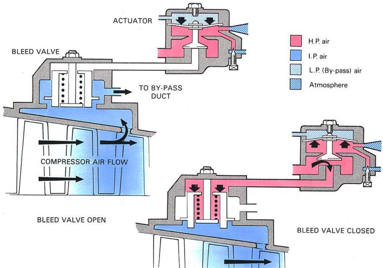
**Fig. 3-17 A pneumatically operated bleed valve system.**
