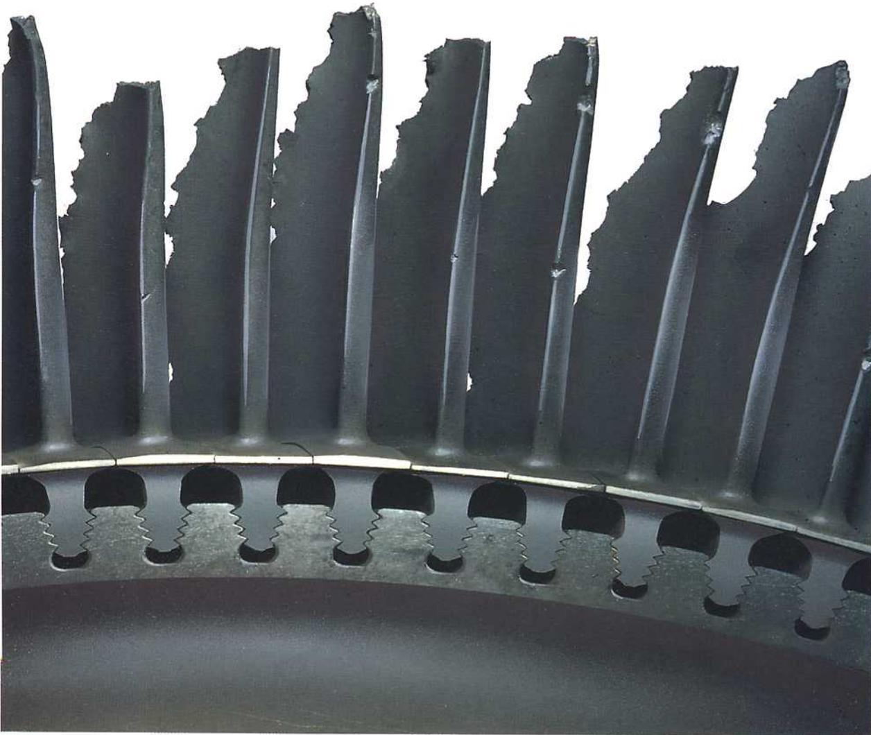
**Fig. 24-9** Overheated turbine blades.
