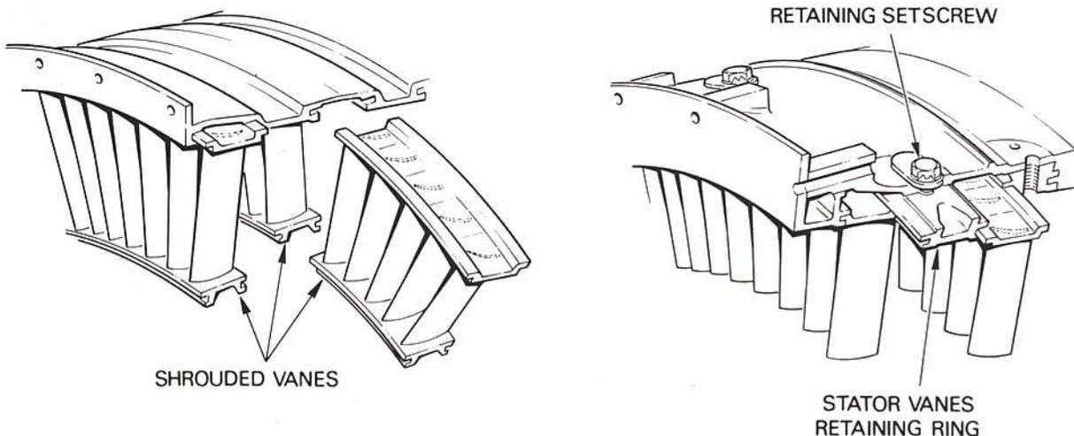
**Fig. 3-13 Methods of securing vanes to compressor casing.**
