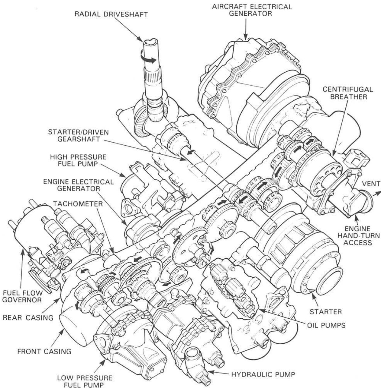
**Fig. 7-4 An external gearbox and accessory units.**
