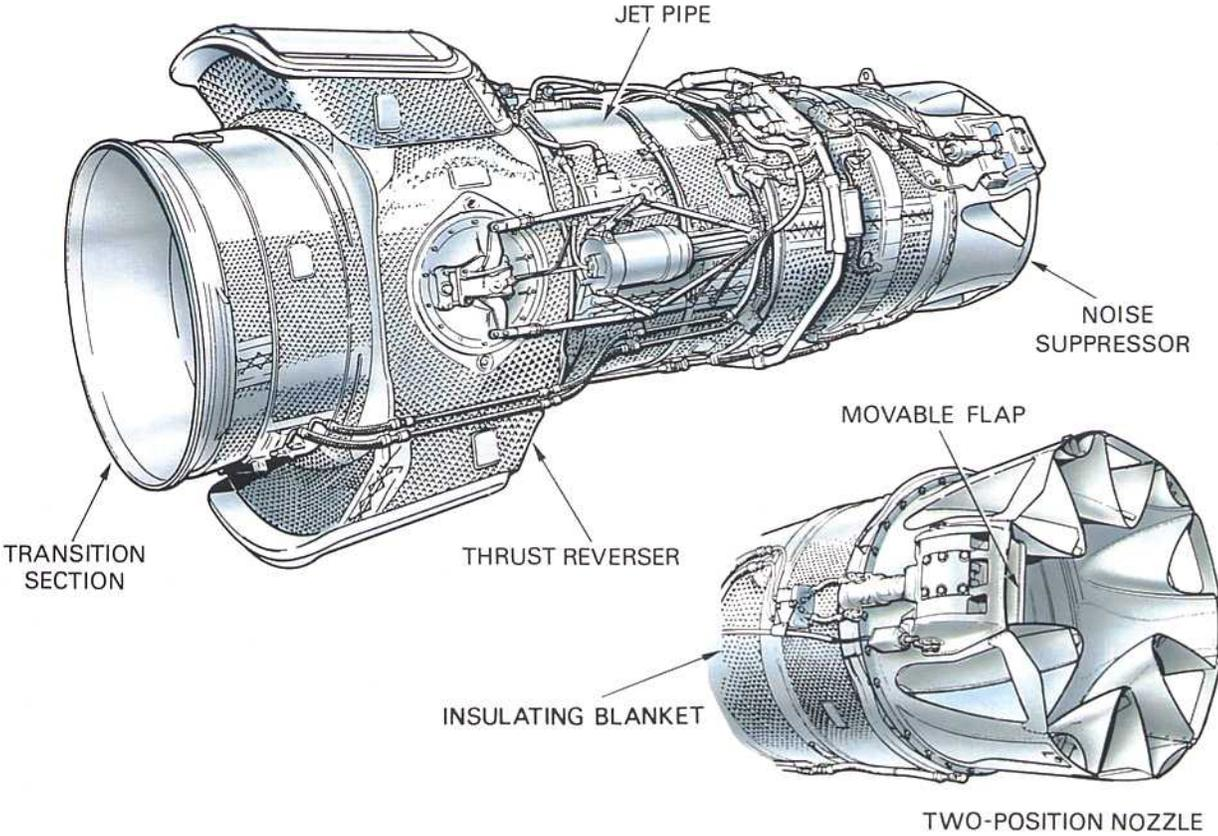
Fig. 6-2 Exhaust system with thrust reverser, noise suppressor and two position propelling nozzle.
