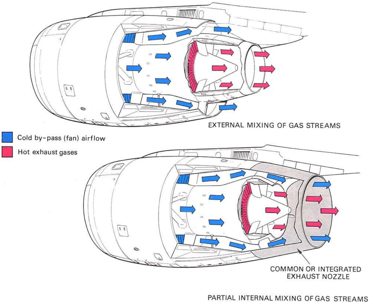
Fig. 6-5 High by-pass ratio engine exhaust systems.
