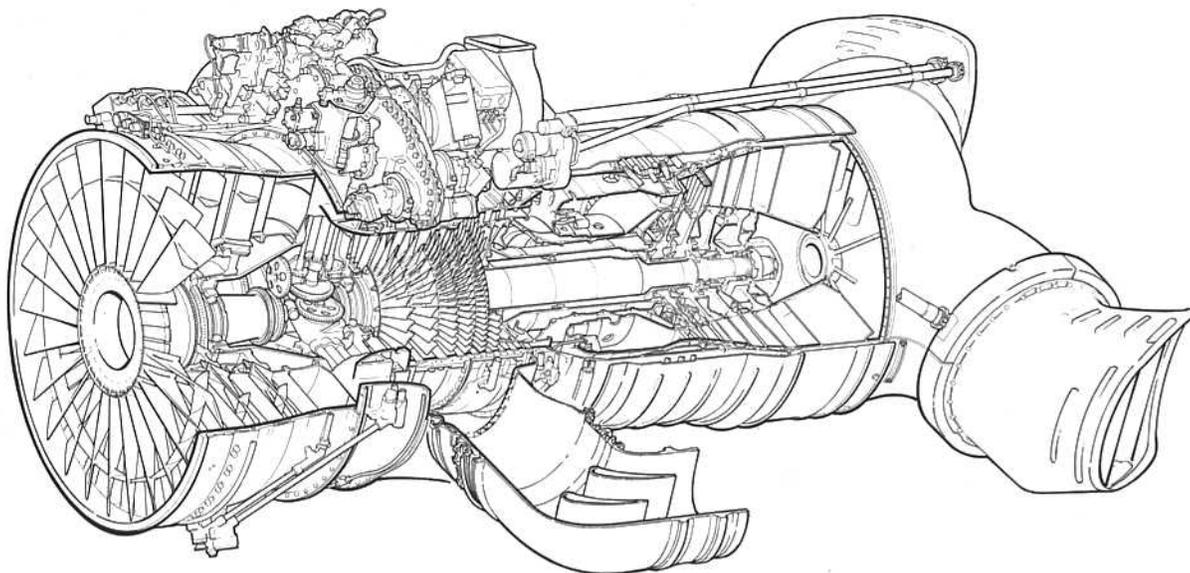
**Fig. 18-2 Lift/Propulsion engine.**
