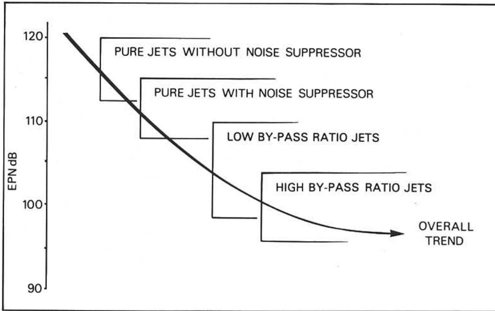
Fig. 19-1 Comparative noise levels of various engine types.
