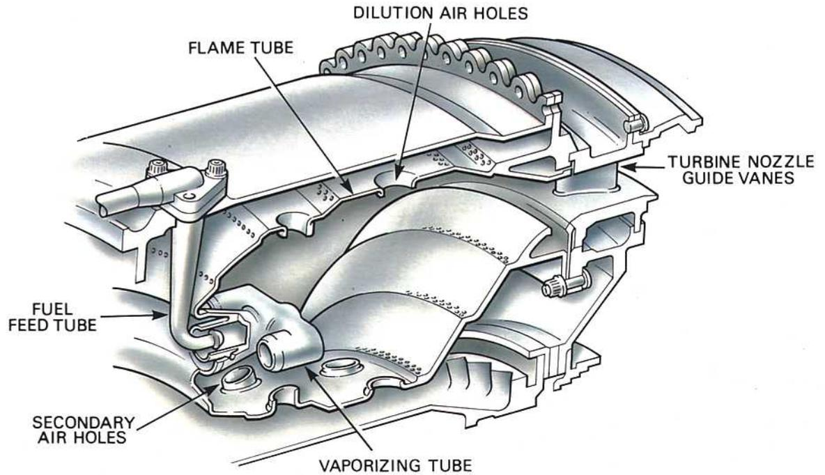
**Fig. 4-5 A vaporizer combustion chamber.**
