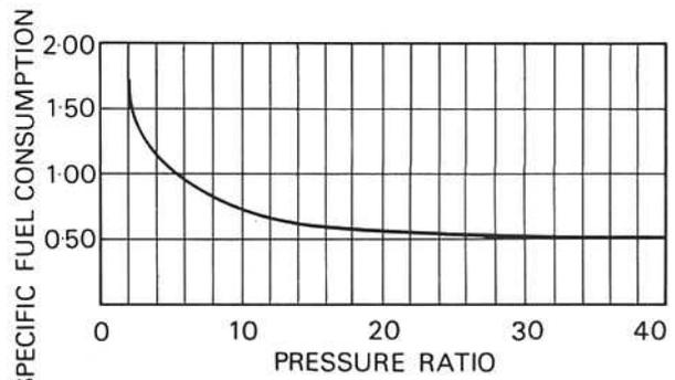
**Fig. 3-2 Specific fuel consumption and pressure ratio.**
