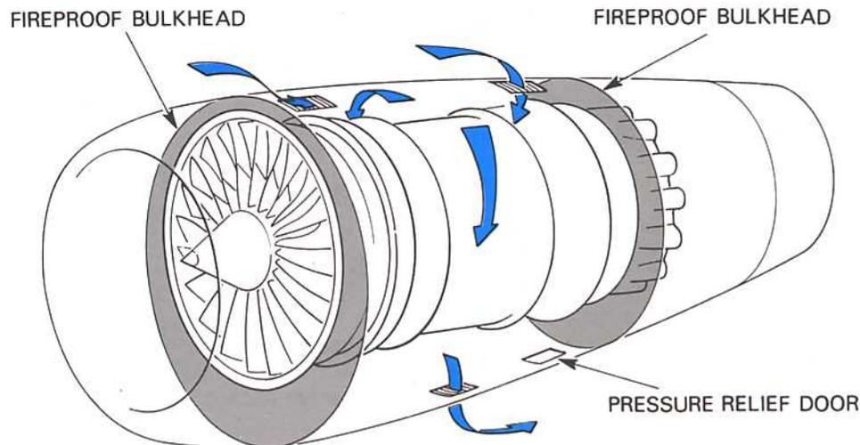
**Fig. 14-1** A typical cooling and ventilation system.
