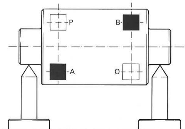
**Fig. 25-5 Unbalance couples due to centrifugal force.**
