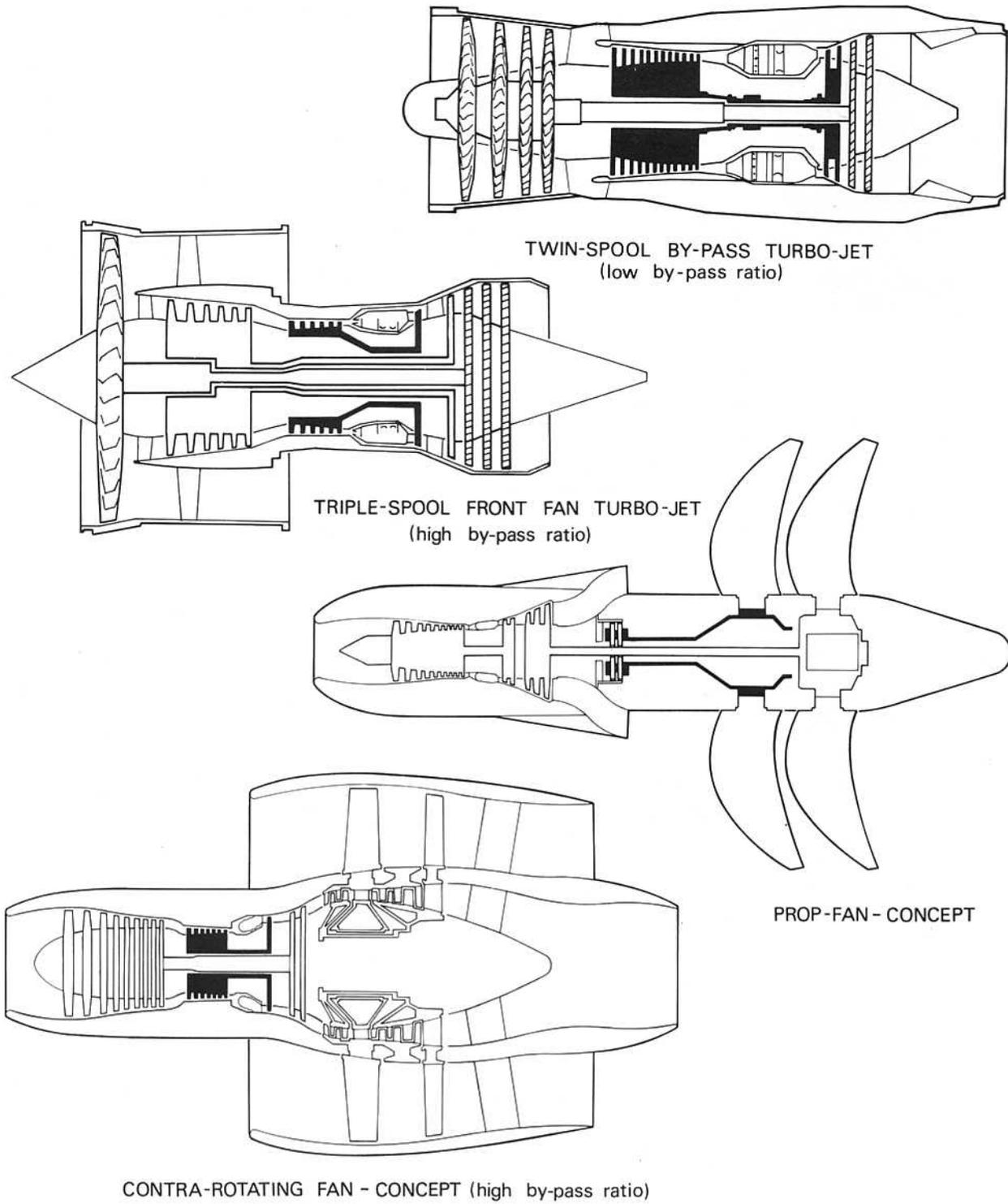
Fig. 1-9-2 Mechanical arrangement of gas turbine engines.
