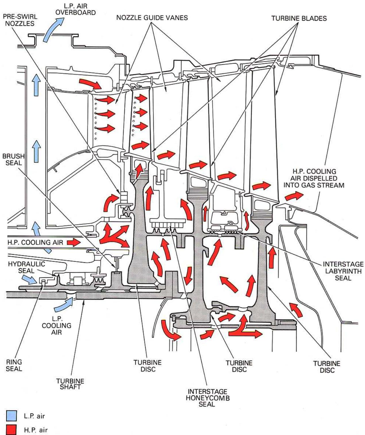
Fig. 9-5 A hypothetical turbine cooling and sealing arrangement.
