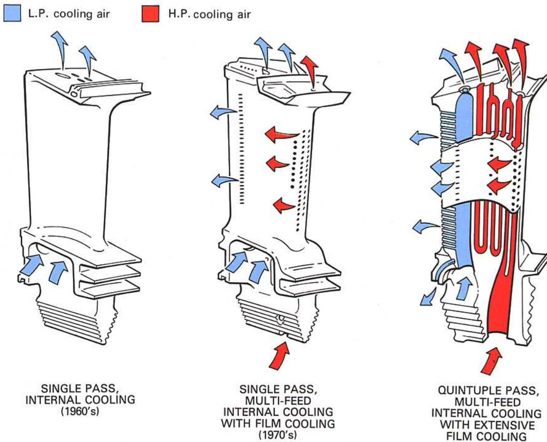
Fig. 9-3 Development of high pressure turbine blade cooling.
