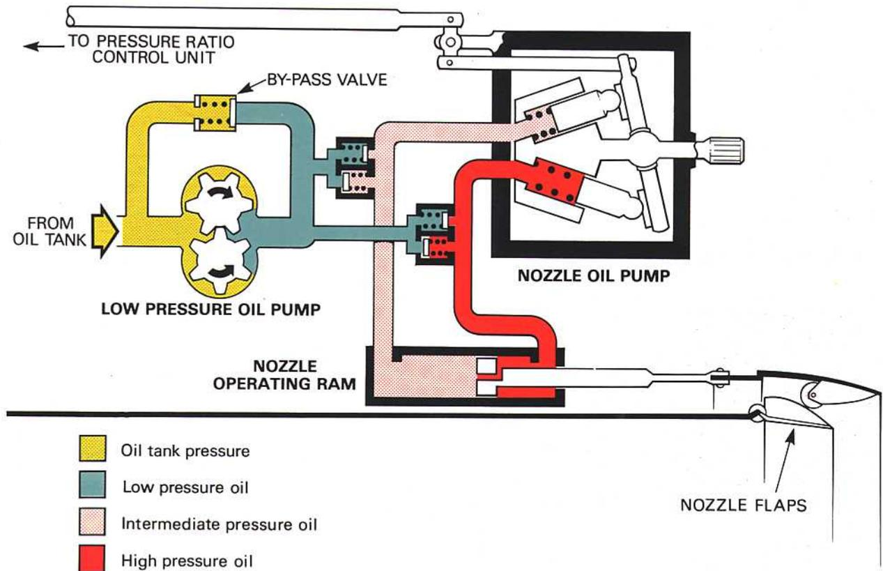
**Fig. 16-7 A simplified typical afterburner nozzle control system.**
