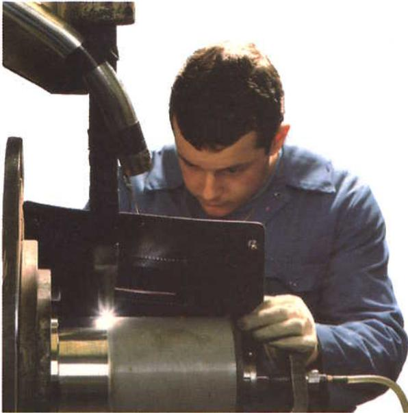
**Fig. 22-8 Tungsten inert gas welding.**
