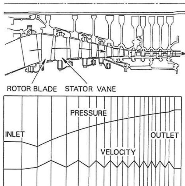
**Fig. 3-9 Pressure and velocity changes through an axial compressor.**
