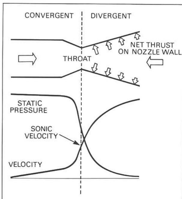
**Fig. 6-3 Gas flow through a convergent-divergent nozzle.**
