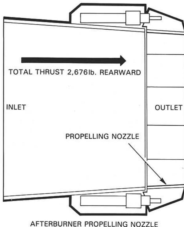
system are reheated to provide additional thrust. The effect of afterburning is to increase the volume of the exhaust gases, thus producing a higher exit velocity at the propelling nozzle.
