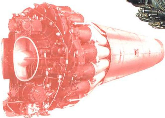
Development of the de Havilland Goblin began in 1941 with the Halford H1 with a design thrust of 3000 lb. The engine passed a 25 hr special category test in September 1942 and was cleared for flight at 2000 lb thrust. This took place in a Gloster Meteor on 5 March 1943 and was also the first flight of that aircraft type. In September 1943 the first flight of a de Havilland DH100 Vampire was made with a Goblin of 2300 lb thrust.
