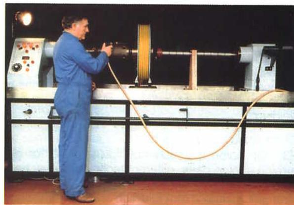
**Fig. 25-3 Magnetic crack testing.**
