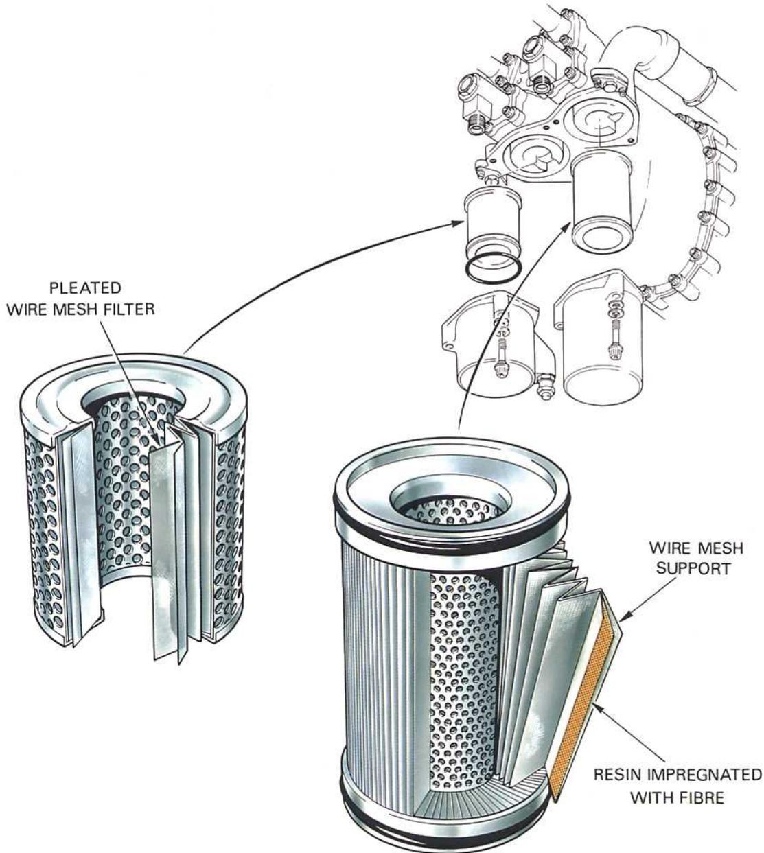
**Fig. 8-12 A typical pressure and scavenge filter.**
