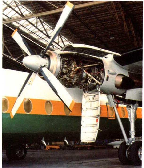
**Fig. 23-13 Engine accessibility, turbo-propeller engine.**
