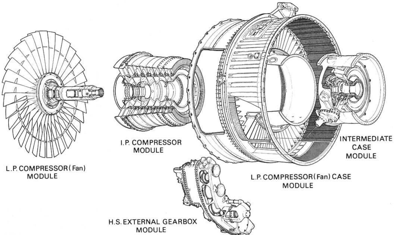
**Fig. 22-1 Arrangements of a triple-spool turbo-jet engine.**
