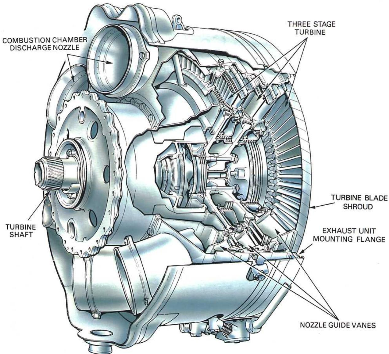
**Fig. 5-1 A triple-stage turbine with single shaft system.**
