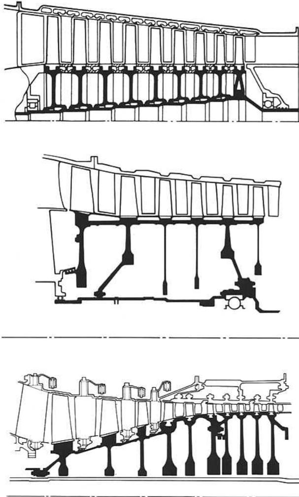
**Fig. 3-10 Rotors of drum and disc construction.**
