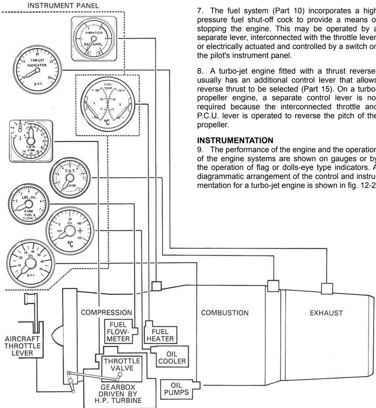
Fig. 12-2 Diagrammatic arrangement of engine control and instrumentation.
