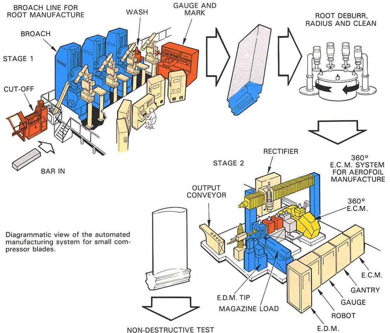
**Fig. 22-12 Typical automated manufacture of compressor blades.**
