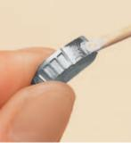
35 To shape pieces no. 5 and no. 6, proceed as indicated in the previous steps, slightly smoothing the flat part with the metal file and then with sandpaper. For the most inaccessible points use the craft knife and, in case of imperfections, proceed as in step 34.
