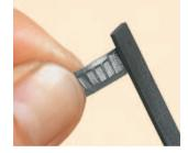
32 After removing the projections, smooth pieces no. 7 and no. 8 with no. 800 grain sandpaper, taking care not to damage the original reliefs. To smooth the hollows, fold the sandpaper in two as shown in the photo.
