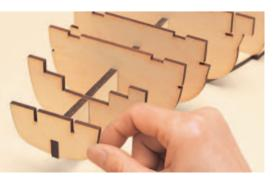
70 After applying glue in the relevant notches on the upper edge of frames nos. 12 and 16, fit the two reinforcements (4). The right edge of the reinforcements reaches the middle of the upper edge of frame no 12 (red circles in the photo).
