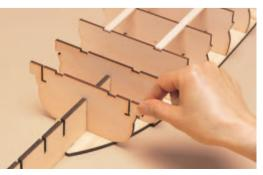
55 Proceed in the same way with the next notches of the keel, and insert frame no. 15 (2). Make sure the frames are set square to the base.
