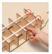
33 In the places where it is difficult to reach with sandpaper, use a craft knife, which can also be used to correct the edges if they are not well modelled. It is easier to deal with such details if you hold the tip of the blade between your fingers.
