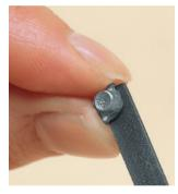
Paint pieces from nos.  $10_{6}$  to  $10_{0}$ . First, spray them evenly with the metal mordant from a distance of 30cm. To avoid the pieces moving, fix them in advance onto adhesive tape.
