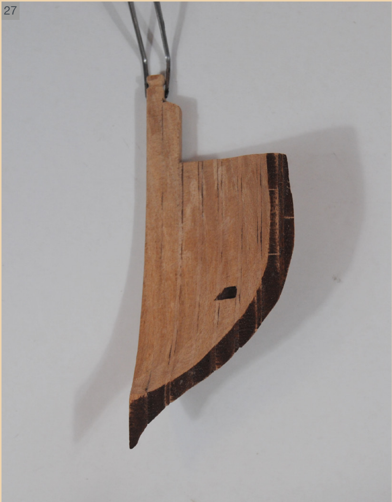
27 Completed hawse piece - rear view.
