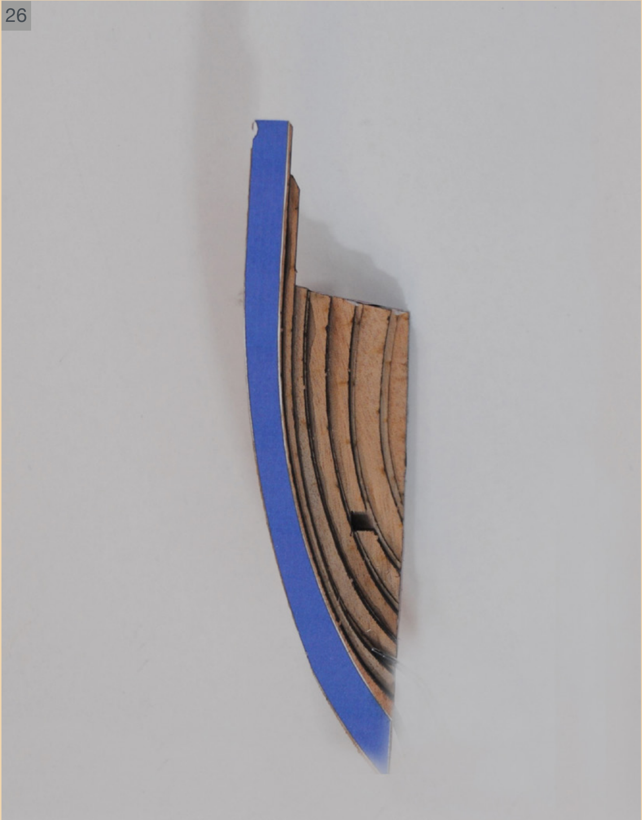
26 Hawse piece with template - keel side.
