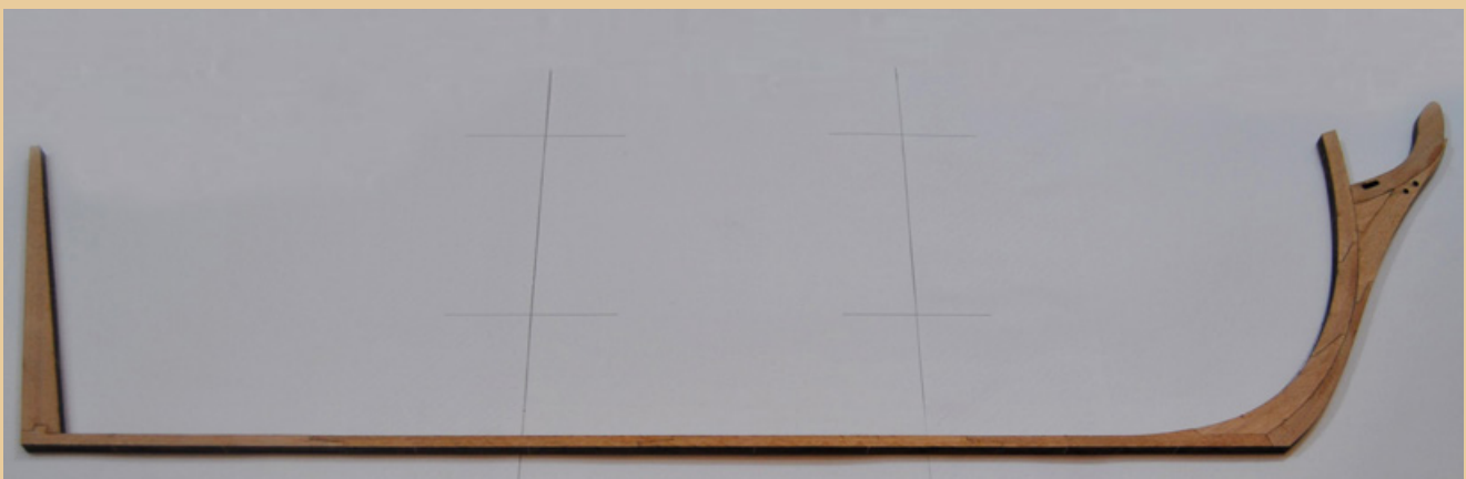
The keel of our HMS Bounty model, built with admiralty techniques.
