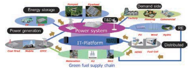
Fig. 16 Smart energy supply chain hydrogen GT
