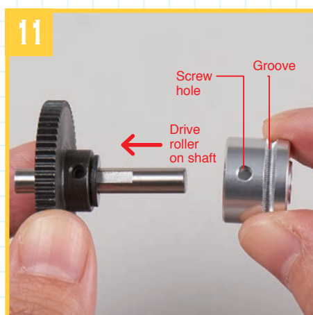
Put the drive roller on the shaft, with the screw hole on the left and groove on the right.
