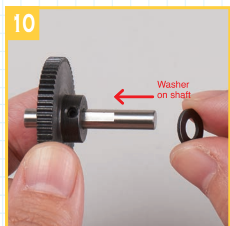
Put the M5 washer you have just removed onto the opposite end of the drive shaft.
