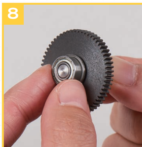
Remove the bearing from the drive shaft.
