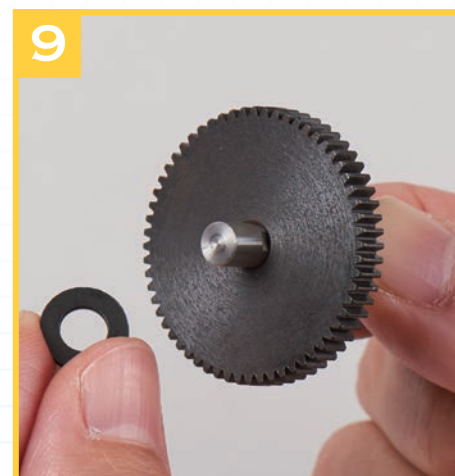
Remove the washer from the drive shaft.
