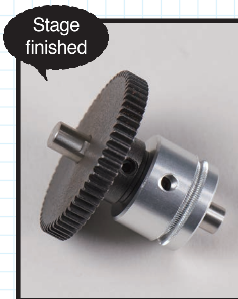
The extruder's large gear has been assembled. Check that your components look like those in the photo above.
