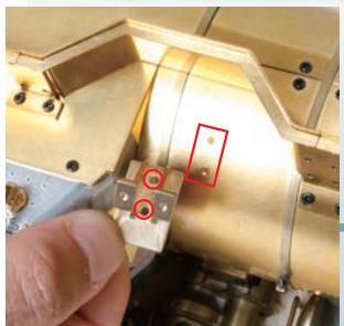
Place the water pump support onto the right side of the boiler, aligning the holes of both.
