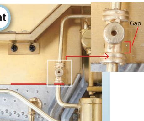
Place the fire hydrant over the water pipe, positioned as shown in the inset and with the bottom edge in line with the bottom of the firebox.
