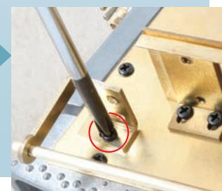
Tighten a 2 x 4mm screw into the hole to secure.
