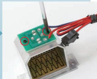
Tighten a 2 x 5mm screw into each hole.
