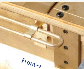
The pipe should be held in the bracket, as shown.
