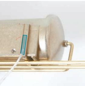
Glue one of the A brackets to the top of the reservoir, positioning it over the tube to hold it in place.
