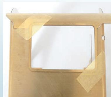
When the glue is dry, remove the tape holding the frame in place.
