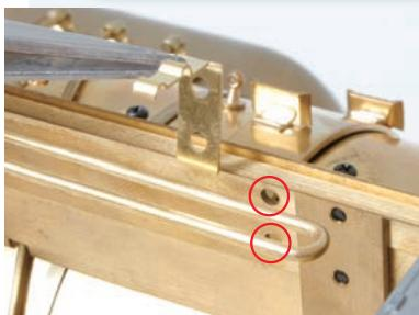
Locate the circled holes in the running board near the looped end of the tube, and place bracket B there, between the board and the tube.
