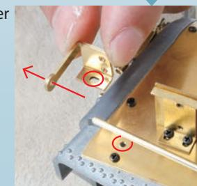
Slide the water pipe support over the end of the water supply pipe until you can align the two circled holes.
