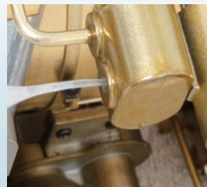
Place a small amount of instant adhesive into the lowest hole on the water pump.
