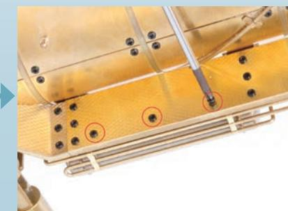
Tighten a 2 x 3mm screw into each of the holes (circled).
