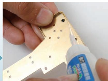
Holding the edging in place, apply instant adhesive to the join between it and the floor.
