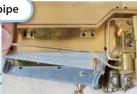
Insert the water supply pipe into the hole in the pump. Make sure the angled area in the pipe doesn't lean in or out.
