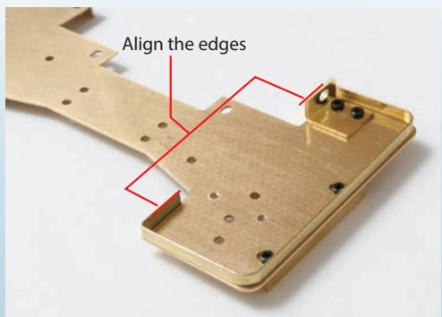
Turn the cab floor over so the underside is facing up. Place the edging on the left side, as shown, and align the inner edge with the edge of the floor.
