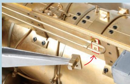
Tighten a 2 x 3mm screw into the circled holes, securing the two brackets.
