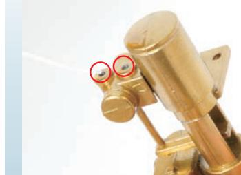
Locate the two circled holes at the top of the water pump. Place a small amount of instant adhesive in each.
