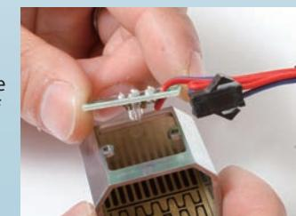
Place the LED board over the hole at the top of the firebox, aligning the holes of both.
