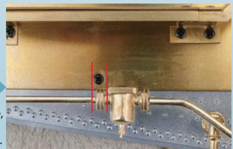
Glue the filter onto the water supply pipe, aligning the left side with the screw above.
