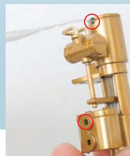
Insert the shorter side of the water pipe into the lower hole and the long side into the hole at the top.
