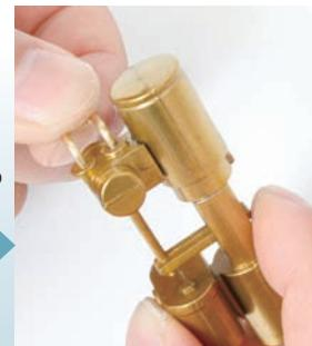
Apply glue to the hole at the top of the pump and the upper hole of the pair at the bottom, both circled.
