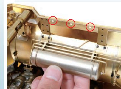
Locate the three circled holes along the right running board in front of the water pump. Align the three holes at the top of the reservoir with them.
