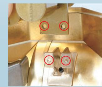
Place the projection of the water pump with two holes in it below the support, aligning the holes of both.
