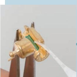
Apply glue to the shaded area at the back of the filter.
