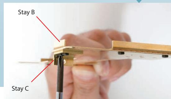
Place stay B (left) on top of the floor, aligning the holes with those highlighted in the previous step. Tighten a 2 x 3mm screw into each hole.
