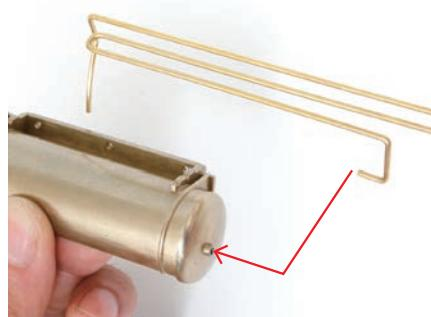
Hold the right air reservoir and insert the end of the cooling tube, following the direction of the arrow.
