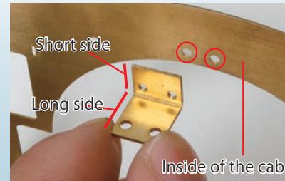
Align the holes on the short side of the stay with those at the front of the cab.
