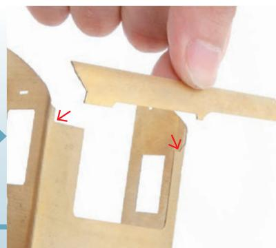
Temporarily hold the top left cab in position at the front with tape.
