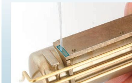
Holding the tube in place, apply some instant adhesive to the highlighted point at the top of the reservoir.
