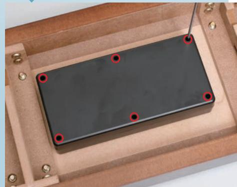
Tighten a self-tapping screw into each of the six circled holes in the speaker cover.
