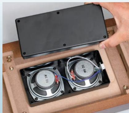
Place the speaker cover onto the back of the speakers, making sure that the socket doesn't come loose from its mount.
