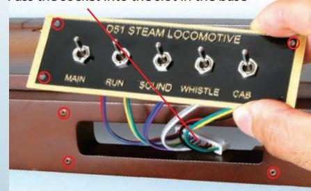
Half-tighten a 2.3 x 8mm self-tapping screw into one of the holes to hold the board in place.
