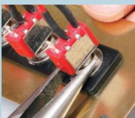
Tighten the nuts on the back of the switchboard to secure the switches in place.
