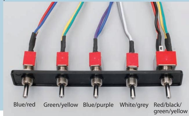
Fit a hex nut onto each of the remaining four switches, then fit them into the switchboard, in the order shown in the photo.
