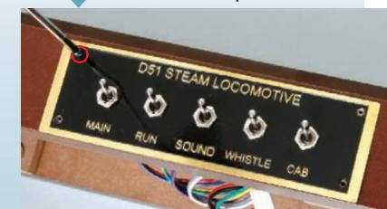
Place the switchboard over the slot in the side of the base, aligning the circled holes.
