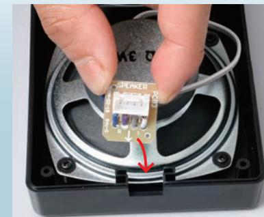
Insert the speaker socket (attached to the speaker) into the mount at the side of the speaker.
