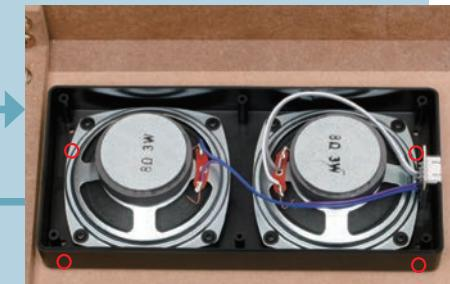
Adjust the position of the speaker so that the four circled holes align with those in the top plate.
