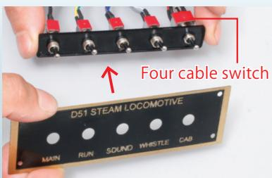
Place the switch plate over the switches and up against the switchboard. Make sure the four-cable switch goes through the 'CAB' hole.
