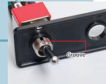
Insert the end of the switch into the first hole on the switchboard, aligning the groove with the projection on the washer.
