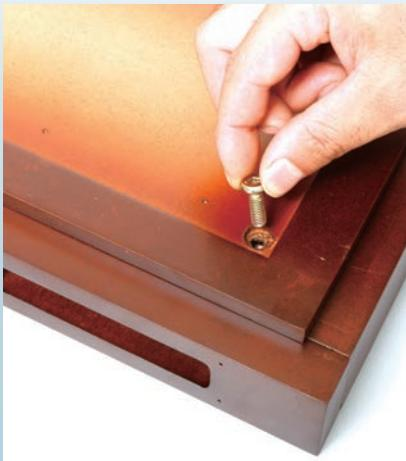
Insert a cap bolt into each of the 16 holes and screw into place by hand.
