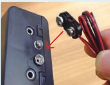
Push the connector on the end of the battery cable onto the one on the battery box.
