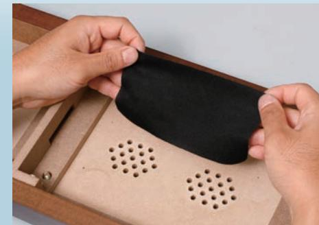
Turn the base assembly over and place the speaker protection cloth over the holes on the underside of top plate C.
