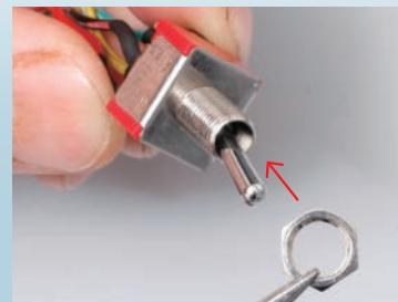
Place a hex nut onto the threaded part of one of the switches.
