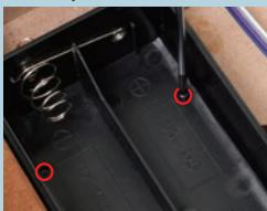
Tighten a 2.6 x 8mm self-tapping screw into each of the four holes in the battery box.
