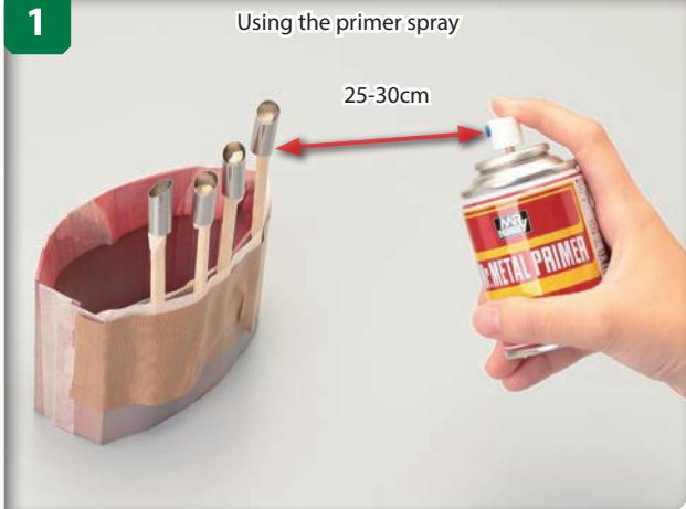
Fix four wooden pencils or disposable chopsticks to a base, so that they are upright, and place the four tailpipes on the ends of them. If the tailpipes slip down, wrap some masking tape below them to keep them in place. Wipe off any dirt, dust or fingerprints on the pipes and, with the can held 25-30cm away, spray them with clear primer. Leave them to dry fully.
