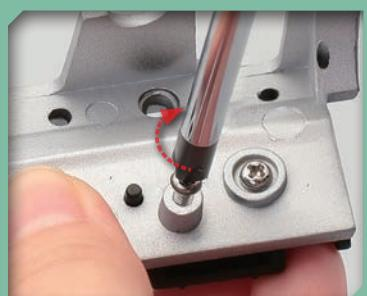
To thread a hole using a spare screw, select one that is the same size as the one you want to screw into the hole. Hold the spare screw to make sure it will go in straight, then turn it clockwise with a screwdriver – you might need to apply a little pressure to get it started. Stop when the screw is two-thirds of the way in, and turn it anti-clockwise to remove it.
