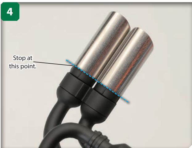
The tailpipes should come to rest just above the ridges on the silencers, as indicated by the blue dotted line.
