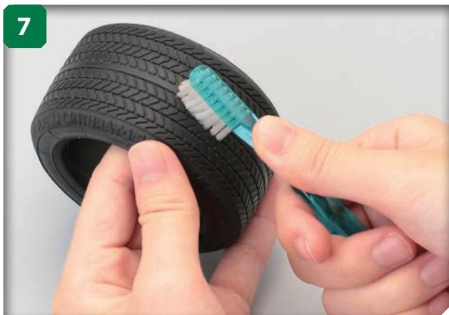
Use an old toothbrush to clean off any debris left over from the moulding process.
