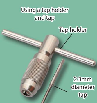
A tap holder has chuck jaws that tighten around a tap, such as the 2.3mm tap shown above, which is for threading holes for 2.3mm-diameter screws. Taps and tap holders are available from hobby or tool shops, and online.
