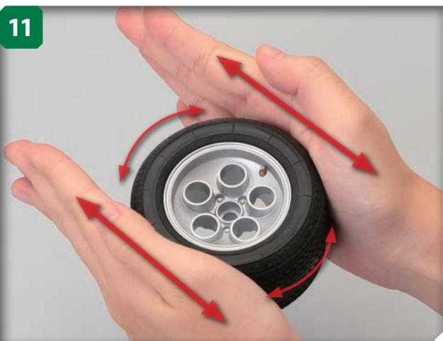
When the tyre is on the wheel, hold the assembly between your hands and roll it back and forth to ensure that the tyre walls are fully seated in the rims.
