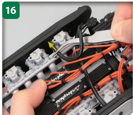
Now press the straight tip of blow-by gas hose A into the right air filter casing adjacent to the oil separator, as shown.
