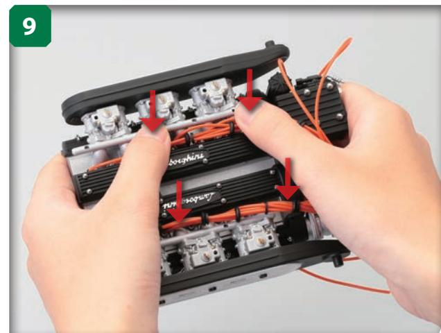
Press down lightly on the two sets of leads so that the ends slip neatly through the holes in the body of the cylinder head, and the tied parts of the leads run flat along the top of it.
