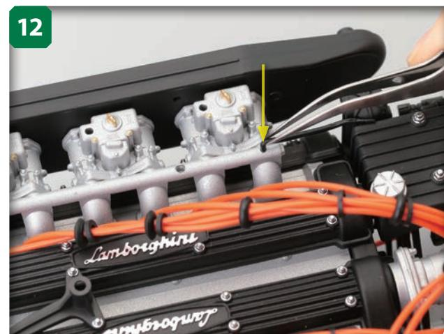
Use tweezers to push the hose fully into the hole, with the free end pointing towards the oil casing.
