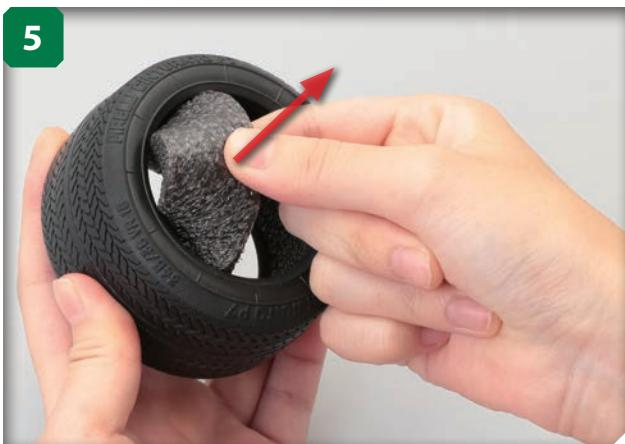
Next, remove the foam insert from the rear tyre, making sure not to damage it.
