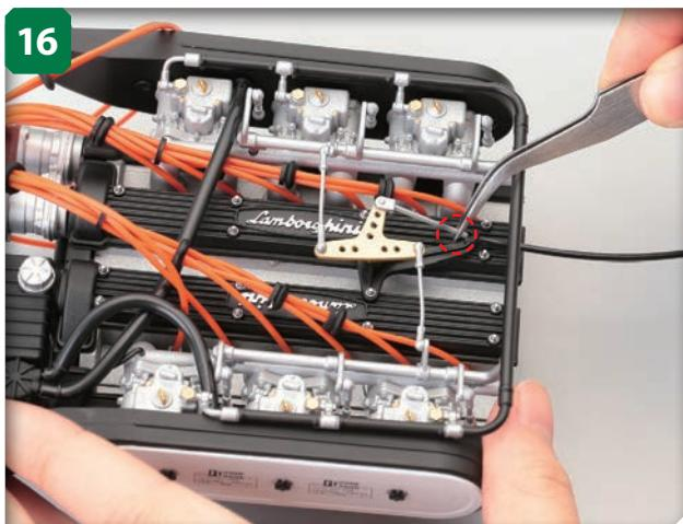
Next, very carefully use tweezers to fit the crank's free rod into the recess on the throttle crank base, as shown. These parts are very thin, so be especially careful when moving them.
