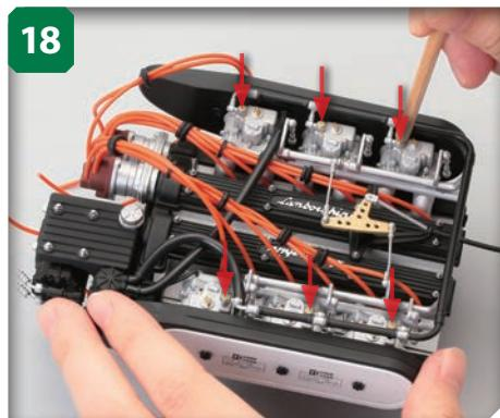
Finally, use the end of a wooden pencil or similar relatively soft object to press the outermost rows of pins into the carburetors, one by one. Do this gently to avoid scratching the gold paint off the parts. Work from the middle outwards as you do this (see Tip box, left).
