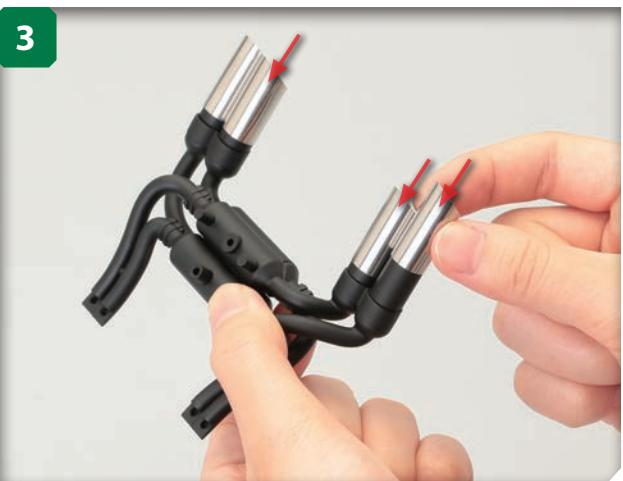
Slide the remaining three tailpipes over the ends of the other silencers, again with their angled ends uppermost. Don't push them all the way on at this point (see Step 4).
