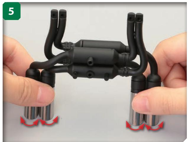
Holding the tailpipes in place, turn the assembly over and place the ends of the tailpipes against your work surface. Turn the tailpipes so that their angled ends are all approximately aligned.
