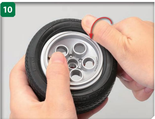
Pull the sidewall of the tyre over the outer rim of the wheel, then repeat for the inner rim.
