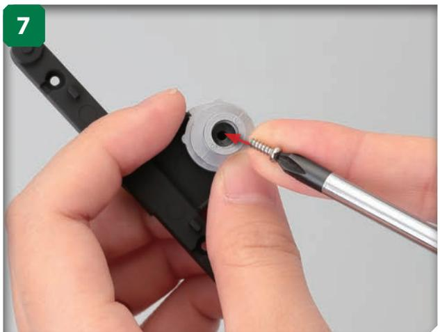
Holding the parts assembled together, place an M2.3 x 6mm self-tapping screw into the indicated hole in the alternator fan.
