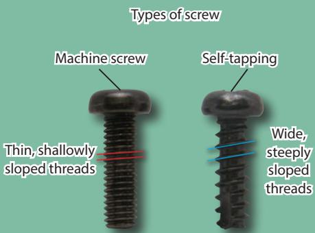
This series uses both machine screws and self-tapping screws. The main differences between them are in their threads, as shown above, and in the way they are used. Machine screws are screwed into holes that have their own internal threads, while self-tapping screws have to cut the internal threads themselves.
