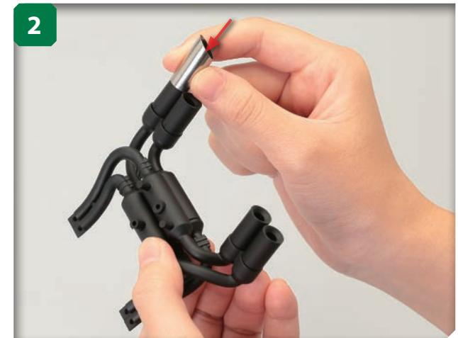
When the primer is fully dry, slide a tailpipe over the end of one of the outer silencers, as shown, with its angled end (arrowed) uppermost.
