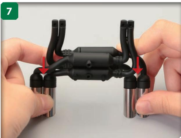
Holding the tailpipes in position, press down evenly on the silencers to push the pipes fully into place.
