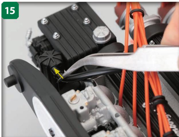
Fit the other end of hose C into the indicated hole on the oil separator, again using the diagram in Step 13 to make sure you have selected the correct hole.
