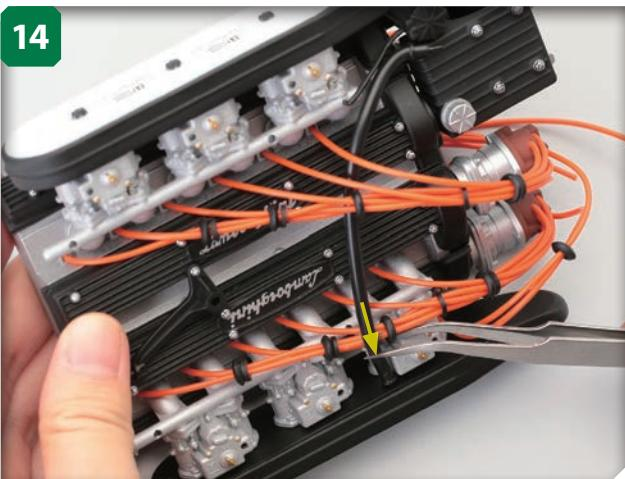
Next, use tweezers to fit the straight end of the blow-by gas hose C into the indicated hole on the left air filter casing, and pass the hose across the cylinder head, as shown.
