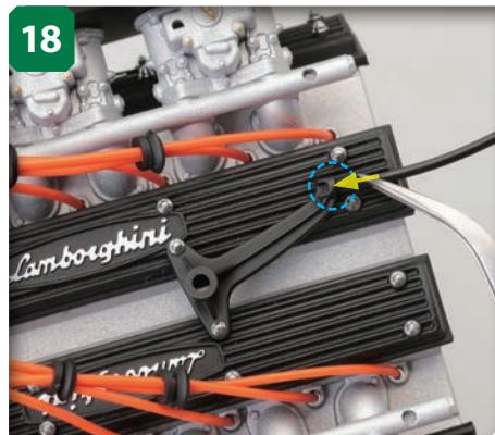
Lastly, push the end of the throttle cable over the pin at the end of the throttle crank base at the far end of the cylinder head assembly, as shown.
