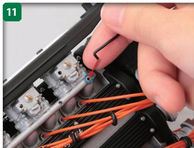
Back on the top of the cylinder head, locate the hole marked by the blue circle and place the L-shaped tip of the blow-by gas hose B into it (red arrow).
