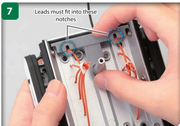
You do not need to fasten the part into place at this stage, but make sure the circled high-tension leads are sitting in the notches of the spacer.
