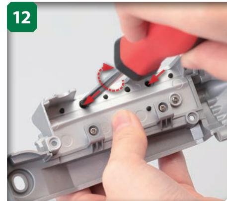
Partly tighten the screw, then insert a second M2 x 5mm countersunk screw into the indicated hole to the left. Now tighten both screws so that the exhaust pipe cannot move.
