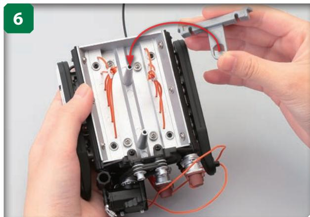
Take the cylinder head assembly and place it upside down on your work surface. Fit the cylinder head spacer over the indicated post, the one that is furthest away from the belts and distributors, as shown.
