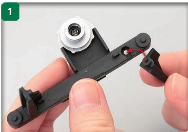
As you did for the right-hand bracket, line up the alternator bracket L with the indicated hole on the alternator assembly.
