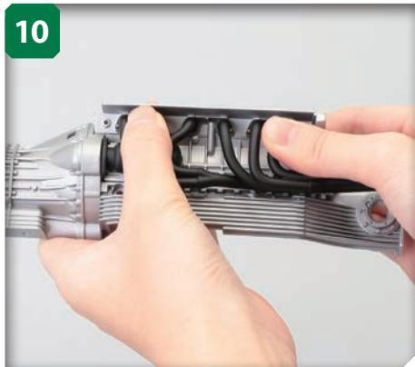
Press the exhaust pipe's pins into the holes to attach it to the block.
