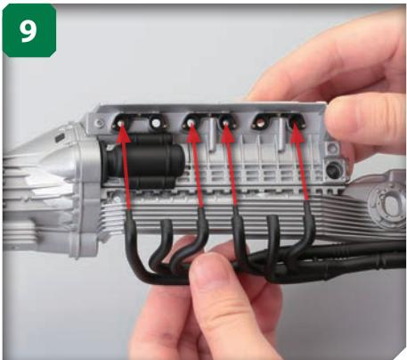
Take the exhaust pipe L from Stage 13 and line it up with the holes in the side of the engine block. The pins at the tips of the four pipes will fit into the arrowed holes.
