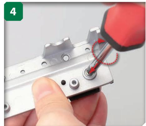
Tighten the screw just enough to prevent the starter from moving.
