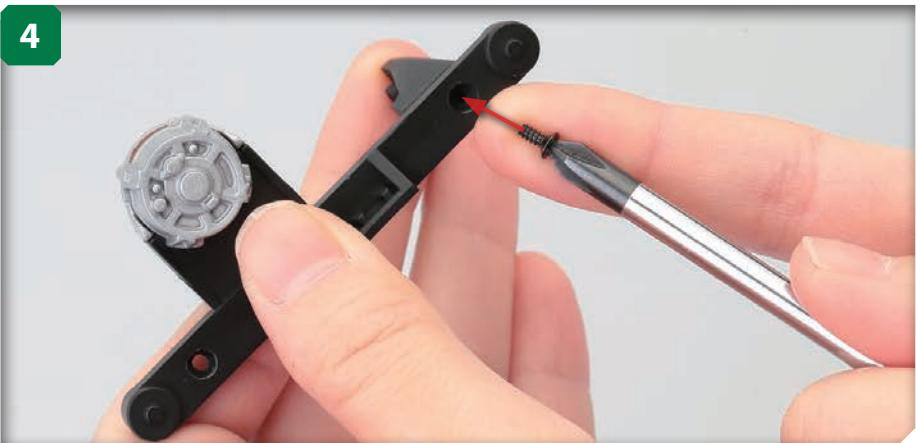
Turn the assembly over and fit an M2 x 5mm countersunk screw into the indicated hole.
