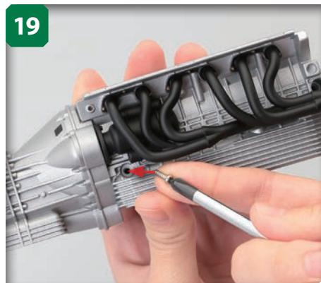
Insert an M2.3 x 6mm self-tapping screw into the indicated hole.
