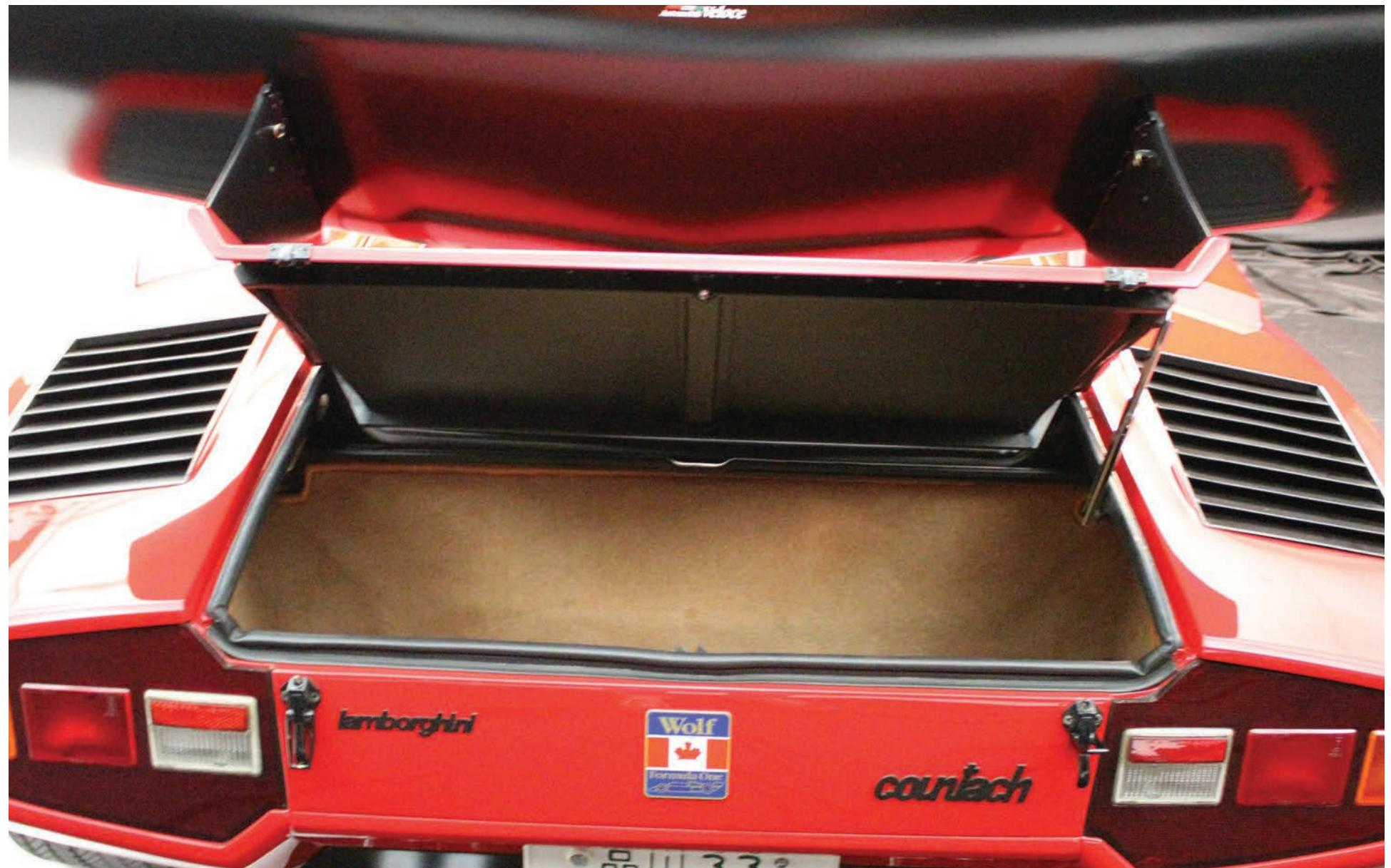
The majority of the space towards the rear of the Lamborghini Countach LP 500S was given over to the car's V12 engine, which was not only sizeable but also positioned longitudinally. As a result, storage space at the rear of the car was very limited.
