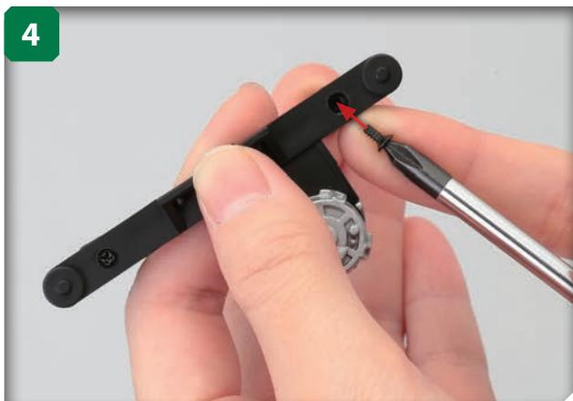
Turn the parts over and insert an M2 x 5mm countersunk screw into the indicated hole.
