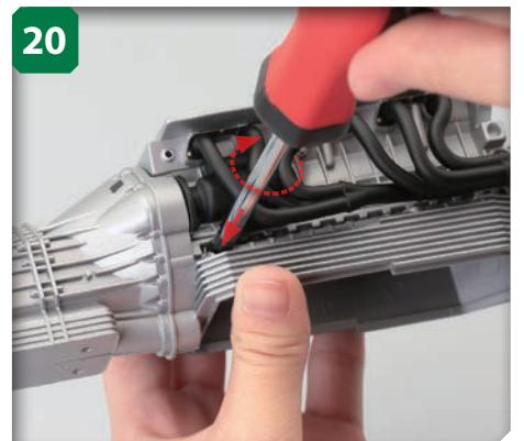
Tighten the screw with the screwdriver until it resists the turn.
