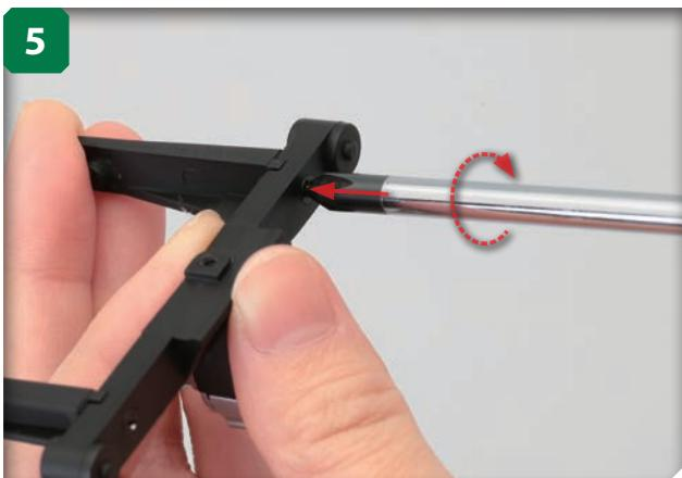
Tighten the screw to secure the bracket.
