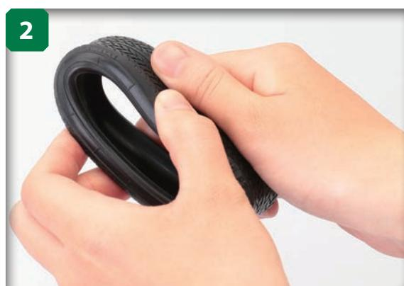
After removing the sponge, squeeze the tyre a few times to make it more pliable.
