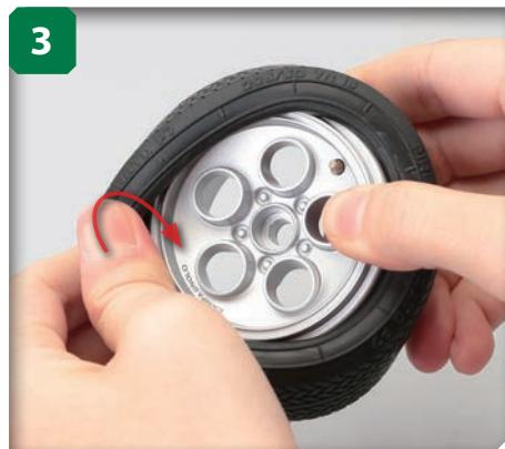
3 Working around gradually, pull the lip of the tyre over the wheel, as shown.
