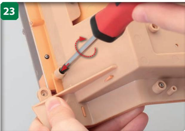
Insert the second M2.6 x 6mm self-tapping screw and, as you have done previously, alternately tighten this and the first screw by half a turn at a time, until any gaps between the parts disappear.
