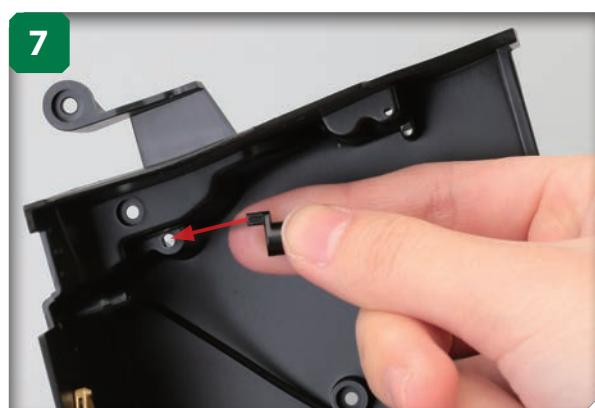
Line up the A/C dryer filter to the hole, as shown.
