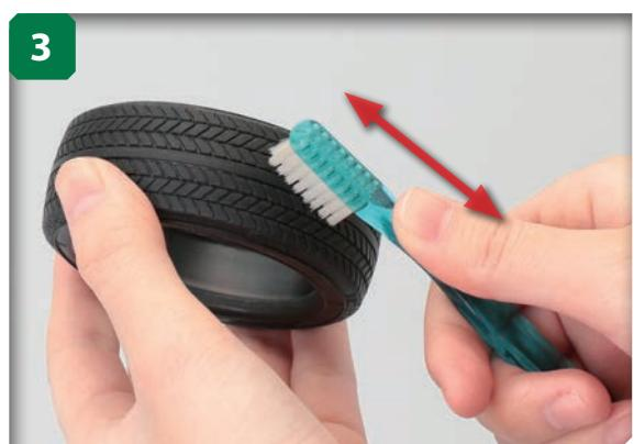
Brush the entire surface of the tyre with an old toothbrush. This will remove any debris left over from the moulding process.
