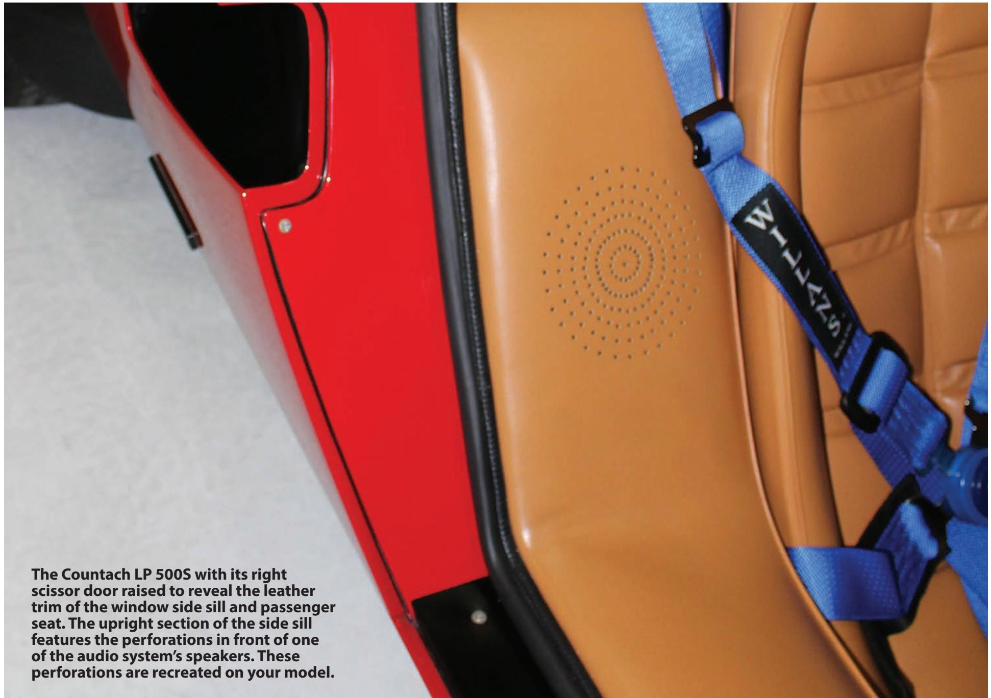
The Countach LP 500S with its right scissor door raised to reveal the leather trim of the window side sill and passenger seat. The upright section of the side sill features the perforations in front of one of the audio system's speakers. These perforations are recreated on your model.
