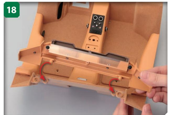
18 Take the rear window assembly, from Stage 19, and line up the mounting posts on each side of the part with the holes on the rear of the cockpit floor (arrowed).
