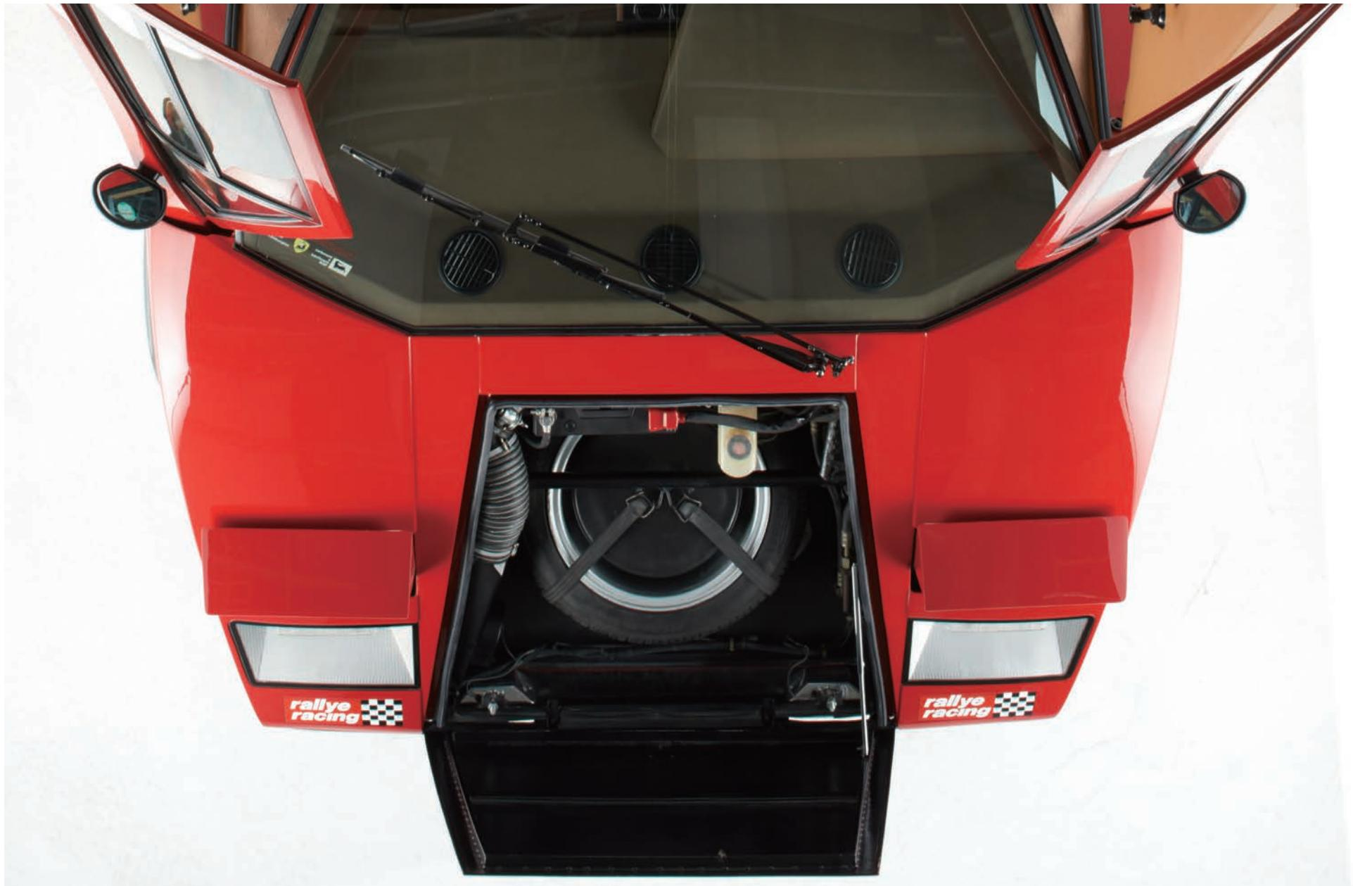
**With the rear section of the Lamborghini Countach LP 500S devoted to its sizeable V12 engine, the spare wheel is stored in the front compartment.**
