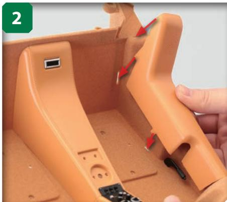
Lower the left side sill into position, rear end first. The arrows show the sill's locating tabs, and the holes in the cockpit floor into which they fit.
