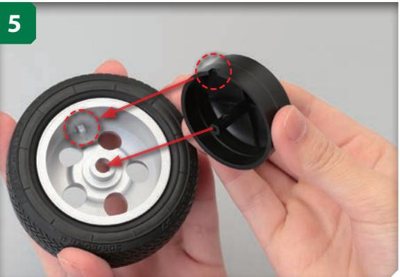
Holding the spare tyre and wheel as shown, line up the spare wheel cover so that its circled notch lines up with the nib on the wheel.
