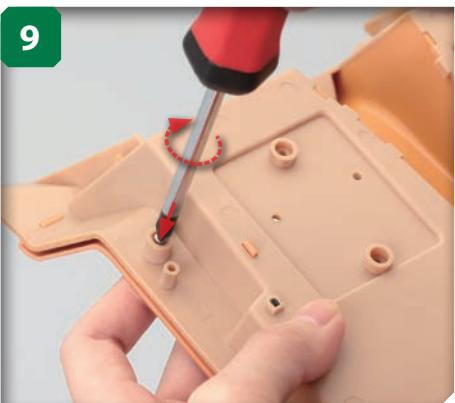
Tighten lightly with a screwdriver.
