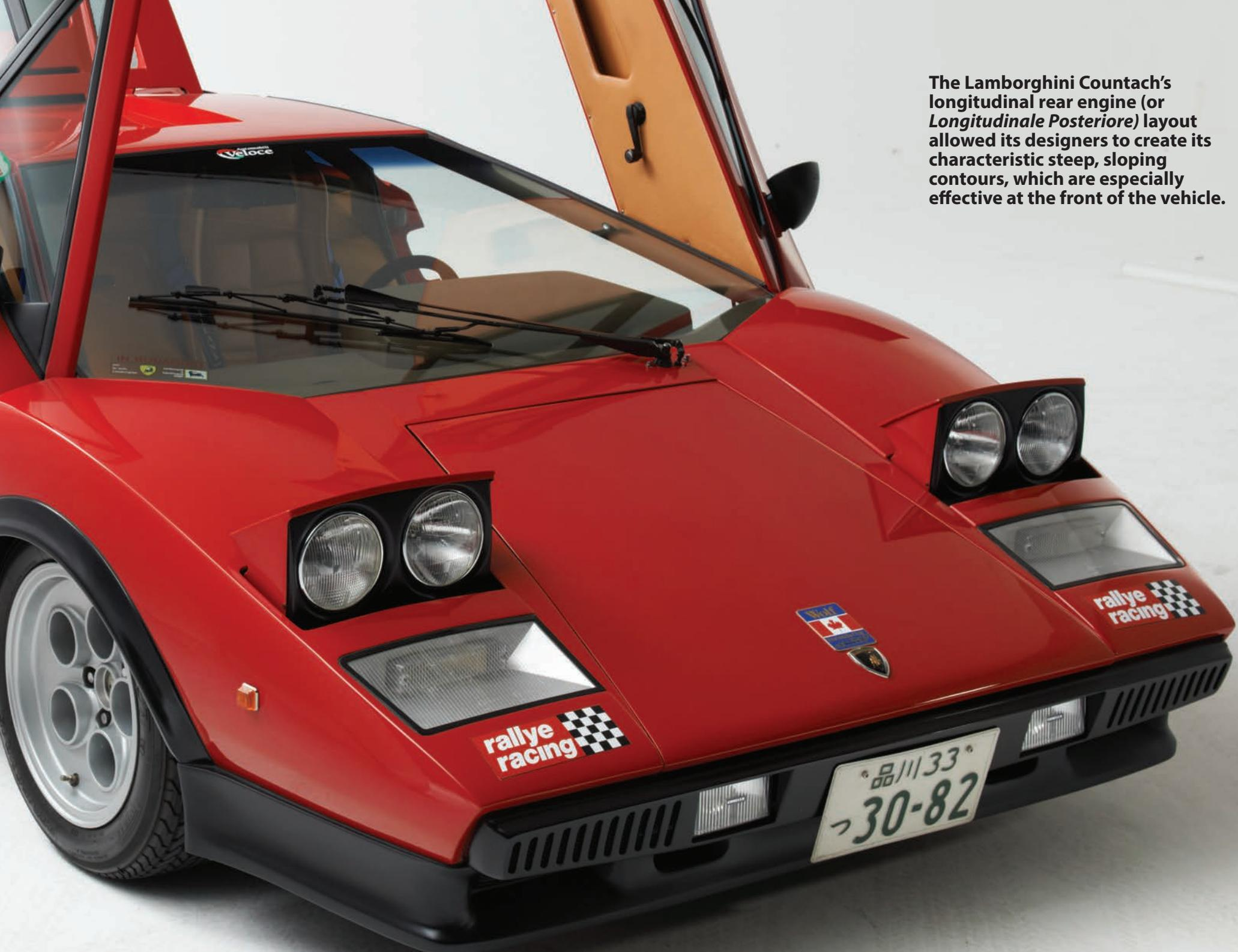
The Lamborghini Countach's longitudinal rear engine (or *Longitudinale Posteriore*) layout allowed its designers to create its characteristic steep, sloping contours, which are especially effective at the front of the vehicle.
