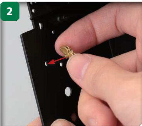
Line up the D-shaped post on the bonnet lock to the correspondingly shaped hole circled in the previous step.
