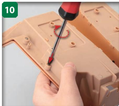
Insert a second M2.3 x 6mm self-tapping screw into the other hole and begin to tighten it. As you did when attaching the cockpit's centre console to its floor, tighten the screws alternately, in increments of a half turn at a time, until the gap between the sill and the cockpit floor is closed.
