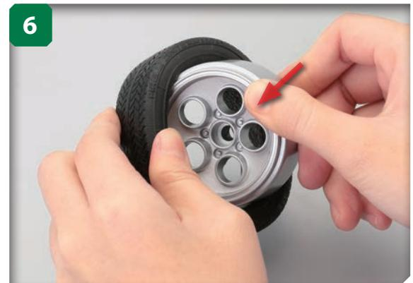
Press the wheel into the tyre, taking care not to scrape off any of the wheel's paint as you do so.
