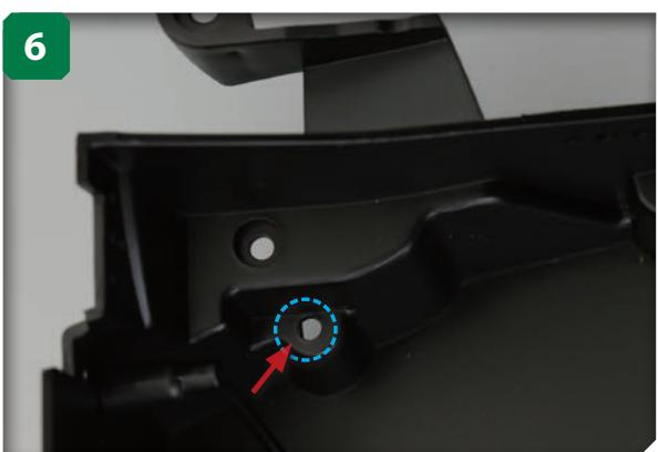
Locate the circled D-shaped hole (again, there are several, so be sure it is the correct one) on the inner edge of the front compartment.
