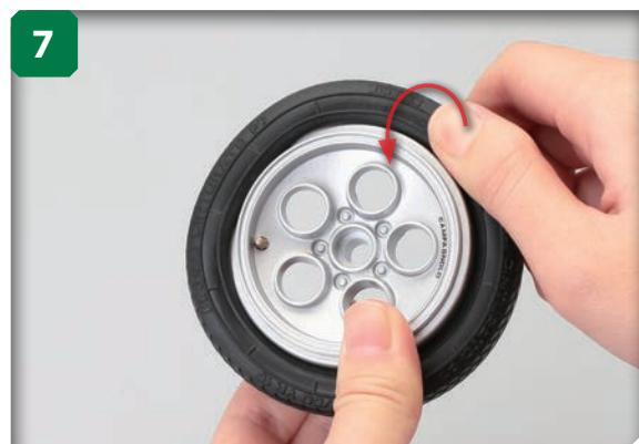
Turn the wheel over and fit the sidewall of the tyre over the inner rim of the wheel.
