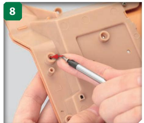
Turn the assembly over and insert an M2.3 x 6mm self-tapping screw (Stage 20) into the indicated hole.
