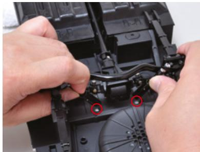
Insert the ends of the rear shock absorbers into the circled holes.
