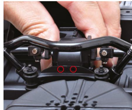
Lift the differential until the screw holes circled in the photo are aligned.
