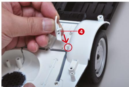
Attach the right hinge mounting bracket to your model's rear right mudguard, positioning the pieces as shown in the photo.
