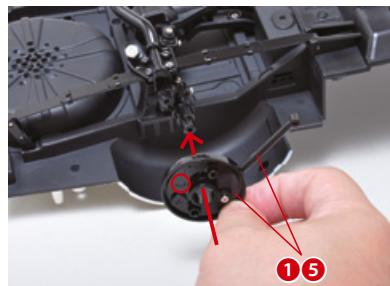
Attach the left disc to the corresponding end of the rear suspension, as shown in the photo.
