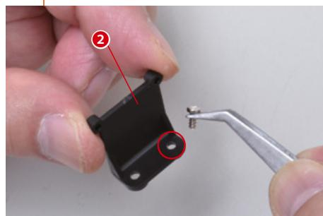
Insert one of the screws received with this stage into the hole in the mount bracket circled in the photo.
