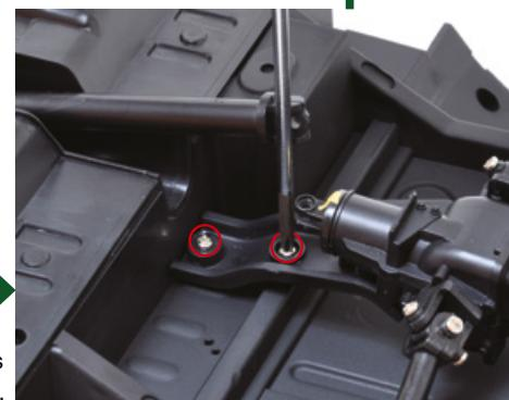
Insert and tighten two type A screws in the circled holes.
