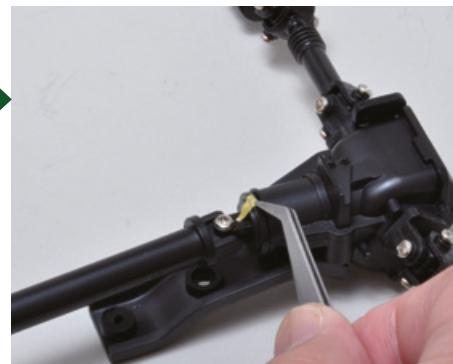
Turn the piece over and apply a strip of adhesive tape to identify the side of the differential shown in the photo.
