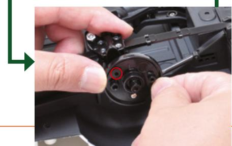
Turn the components to align the screw holes, as shown in the photo.
