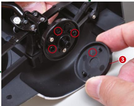
Attach the left drum to its disc, positioning the pieces as shown in the photo.
