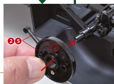
Repeat the previous steps to attach the right disc to the other end of the rear suspension.
