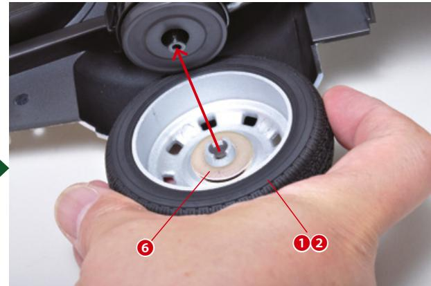
Put a washer on the lynchpin on the inside of the rim. Attach the wheel to the end of the rear axle.
