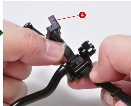
Position the pieces as shown in the photo, then attach the left jounce bumper to the rear left suspension.
