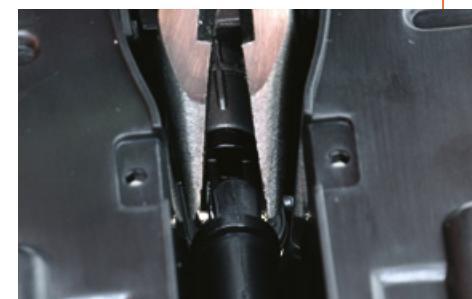
Turn the yoke on the transmission and use the pliers to push the linchpin into place.
