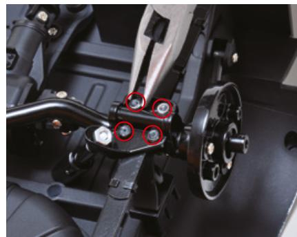
Fully tighten the nuts on both sides of the rear suspension.
