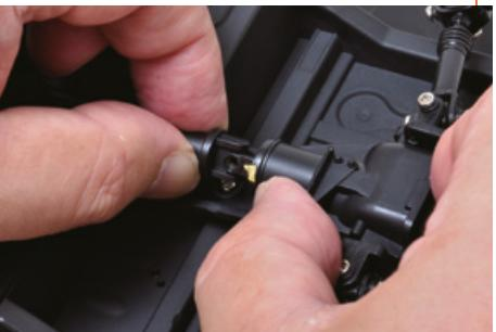
Secure the pieces together with the screw you removed in step 4, then remove the strip of adhesive tape.
