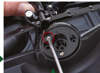
Insert and tighten a type C screw to secure the pieces.
