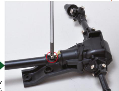
Temporarily remove the screw and the driveshaft.
