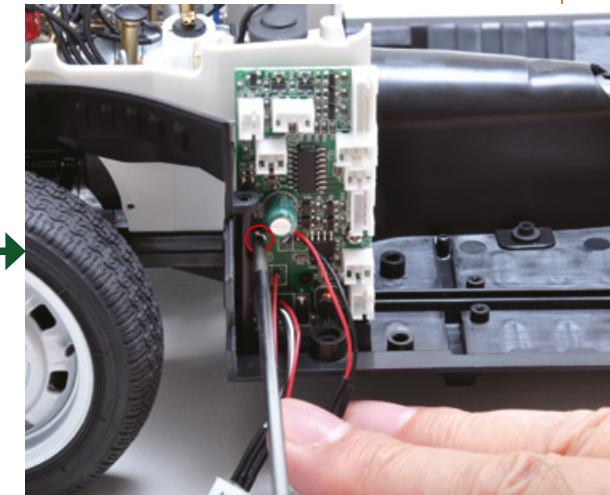
Insert and tighten a second screw in the hole circled in the photo.
