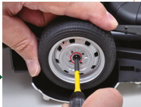
Secure the pieces with one of the screws you received with stage 52.
