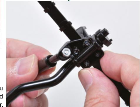
Reattach the nut you removed in this step to the end of the shock absorber.
