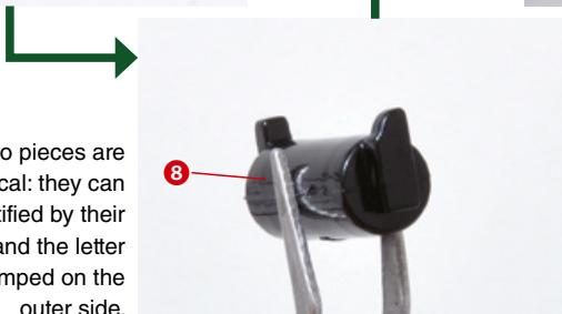
The two pieces are not identical: they can be identified by their shape and the letter stamped on the outer side.
