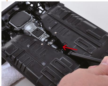
Position the main body of your model as shown in the photo, and insert the driveshaft you removed in step 4 into the transmission.
