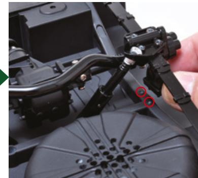
Finally, insert the linchpins on both jounce bumpers into the circled holes.
