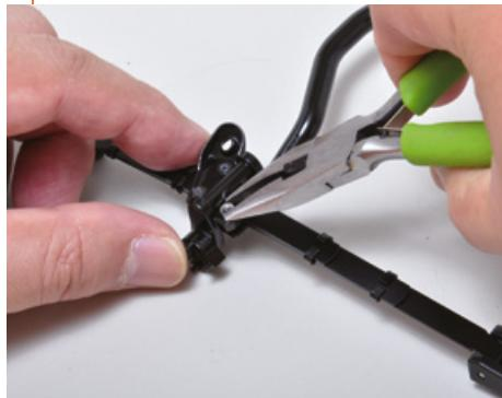
Loosen the four nuts on the rear left suspension.
