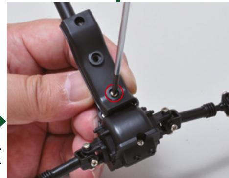
Secure the pieces together with a type A screw, but don't tighten it completely.
