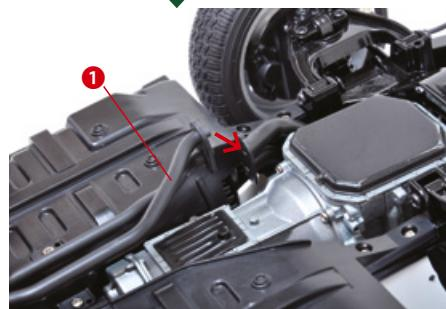
Attach the end of the exhaust pipe to the header, as shown in the photo.
