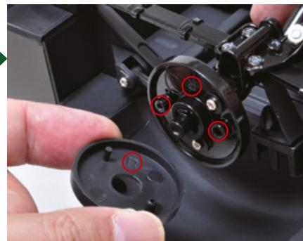
Attach the right drum to its brake disc in the same way.
