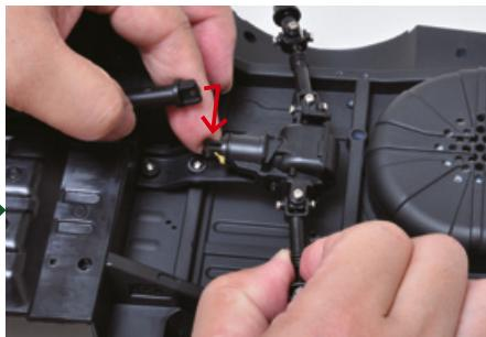
Reattach the driveshaft to the differential.
