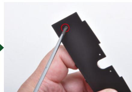
Now insert and tighten another type B screw in the hole on the other side of the panel.
