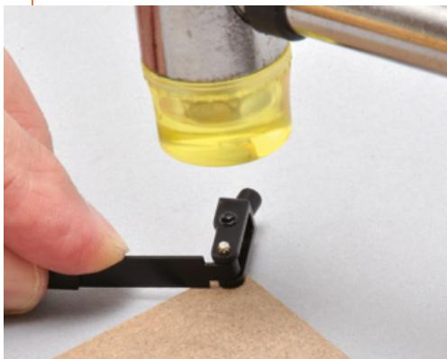
Get the board and hammer you received with stage 17 and hammer the linchpin until it is completely inserted.
