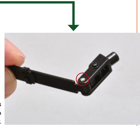
Don't worry if one end of the linchpin is flattened by the hammer; it will have no effect on the rest of the assembly.
