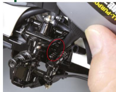
Apply a small amount of oil to the flat part of the tie rod cog, circled in the photo.
