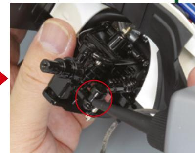
Apply a small amount of oil to the area of the suspension system circled in the photo, where the end of the tie rod goes.
