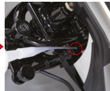
If the screw in the tie rod (circled in the photo) becomes loose, you can apply a drop of instant glue to secure it. Before doing this, fully tighten the screw and then loosen it by about a 1/4 turn, then put some glue in the hole (from the opposite end of the screw head).
