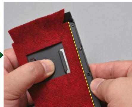
Align the long side and press it down so that it sticks firmly to the corresponding strip of double-sided tape.
