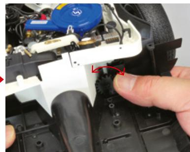
Pick up your model and try to turn the steering column as shown in the photo. Once you have applied the oil, the wheels should turn smoothly.
