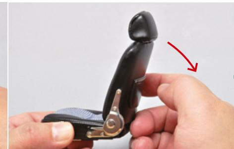
The headrest can also be raised and lowered. Be careful not to separate it completely from the backrest.
