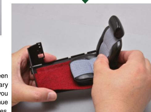
The second seat has now also been installed correctly. This is a temporary assembly; during the following stages you will be removing it to continue assembling the pieces.
