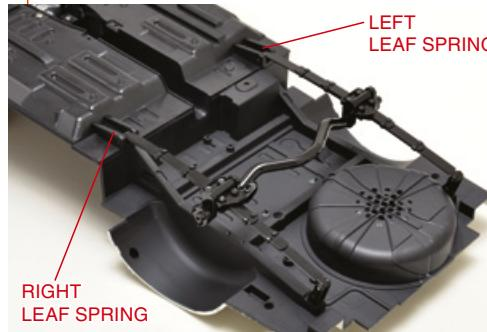
Temporarily install the rear suspension on your model, as shown in the photo. You will secure it permanently in one of the next stages.
