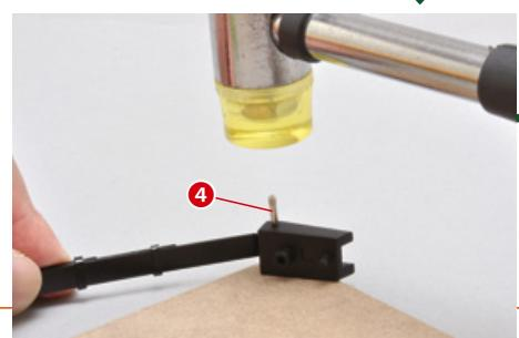
Again, you can use the hammer and board to help you insert the linchpin completely.
