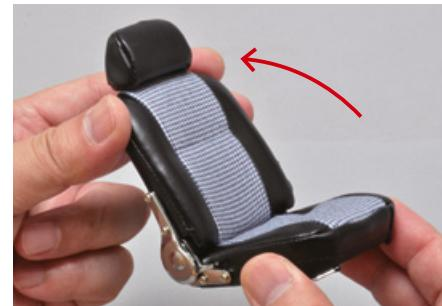
Make sure the seat folds smoothly in both directions. Be careful not to damage the components.
