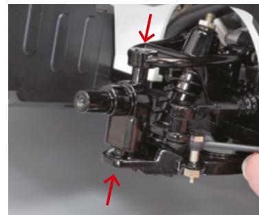
Leave a 2 mm gap between the screws indicated in the photo (where the wheel has been removed) and the surface. If necessary, you can loosen or tighten the screws as required.
