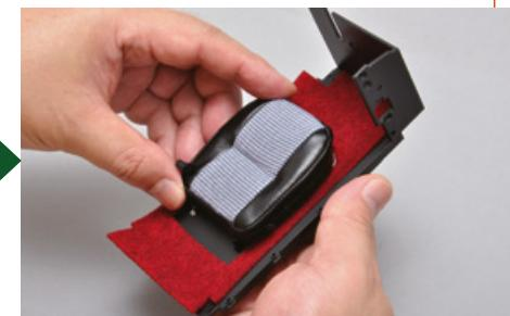
Attach the seat cushion to the platform. Make sure the seat adjustment lever is between the floor mat and the seat cushion.
