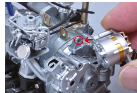
Attach the dynamo using the corresponding interlocking elements indicated in the photo.
