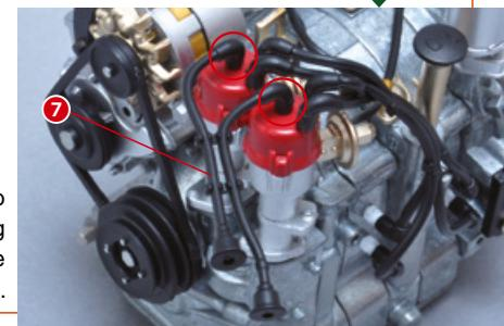
Look carefully at the photo and attach the two spark plug wires A to the remaining distributor caps.
