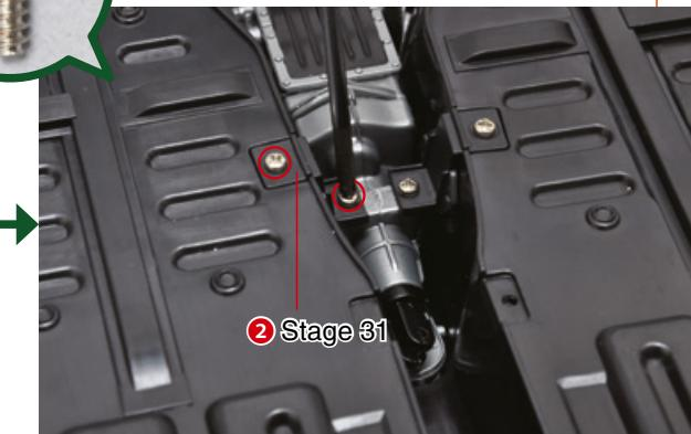
Attach the other mount bracket in the same way and secure the pieces with two type B screws from stage 31.
