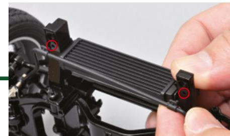
Insert the two lynchpins on the anti-roll bar into the circled holes.
