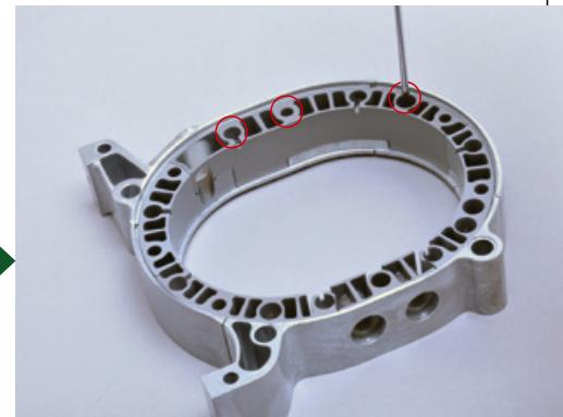
Secure the pieces with three type A screws.
