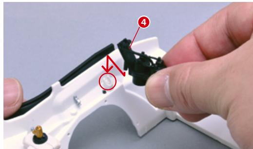
Attach the ignition coil to the body, as shown in the photo.
