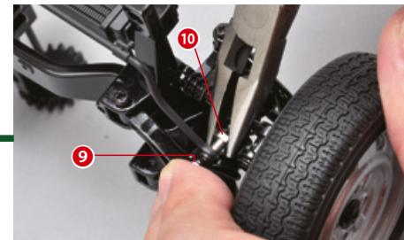
Now insert a bolt into the other end of the anti-roll bar and attach it in the same way; tighten a nut on the end of the bolt.
