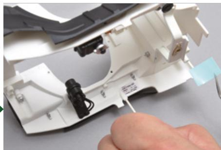
As long as the decal is wet, you can move it around to correct the direction and position. Once satisfied, dry with a cotton bud.
