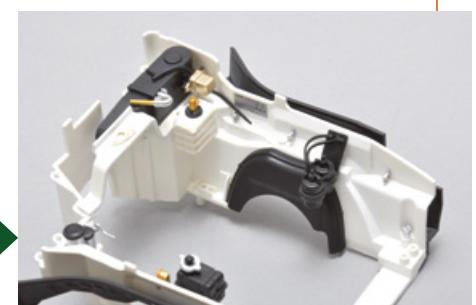
You can now reattach the cooling system, the washer fluid reservoir and the ignition coil. This is a temporary assembly so don't glue the pieces yet.
