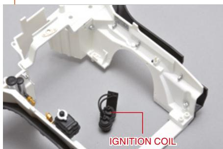
Remove, temporarily, the ignition coil from the body.
