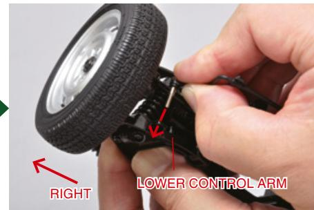
Attach the anti-roll bar to the suspension by inserting the bolt into the hole in the lower control arm in the front suspension. Ensure the pieces face the same way as those in the photos on this page.
