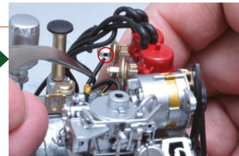
Now insert the shorter end of the other flexible hose into the hole in distributor A, as shown in the photo.
