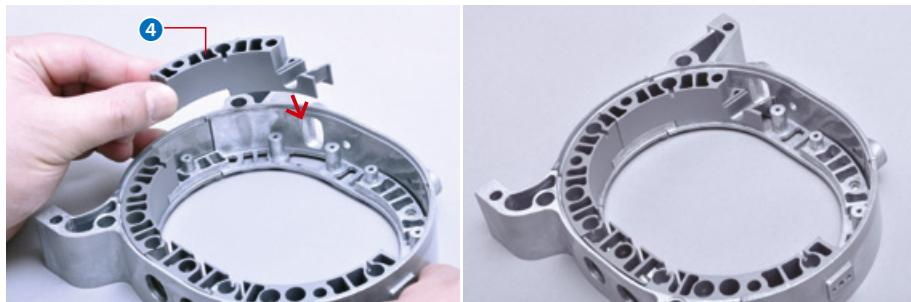
Attach piece S of the rotor housing to the part you assembled in the previous stages.
