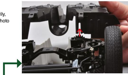
Position the pieces as shown in the photo and attach the front platform to the body.
