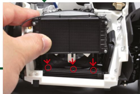
Attach the radiator to the oil cooler, as shown in the photo.
