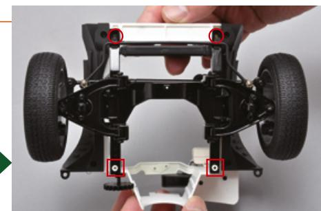
The body and suspension system joined correctly.
