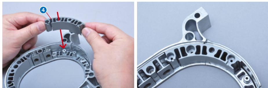
Attach piece R of the rotor housing to the part you assembled in the previous stages.
