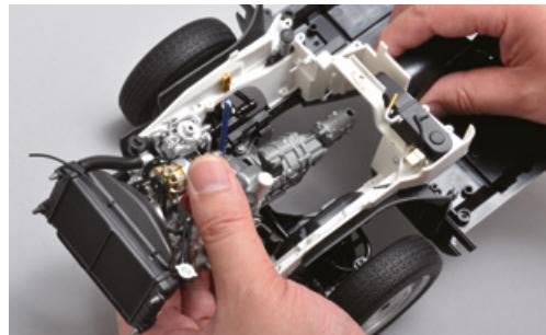
Insert the engine block into the body as shown in the photo.
