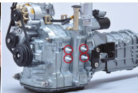
Insert the four spark plugs into the corresponding holes in the left side of the engine block. Look at the photo to see which way they should go.
