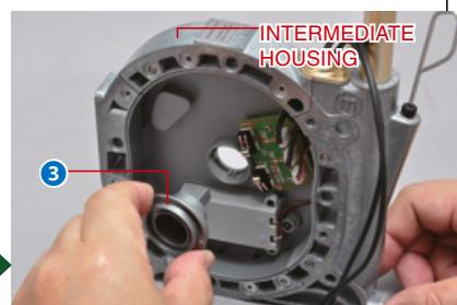
Insert the shift knob adapter into the middle of the intermediate housing, as shown in the photo.
