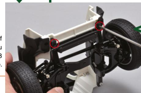
Put the front end of the body on top of the front suspension system. Make sure that the slots and cogs are aligned, as shown in the photo.
