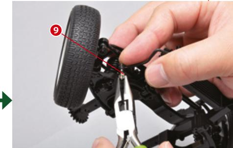
Tighten one of the nuts on the end of the bolt.
