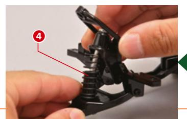
Slide the coil spring onto the shock absorber housing and insert the piston rod into the coil spring.
