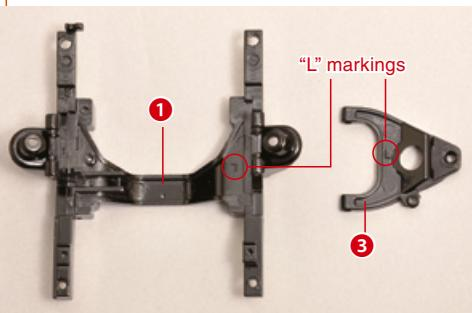
Place the front chassis and the lower left front suspension arm on your work surface.
