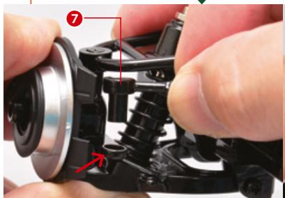
Lift the front suspension arms up and insert the linchpins on the tie rod ends into the holes indicated by the arrows.
