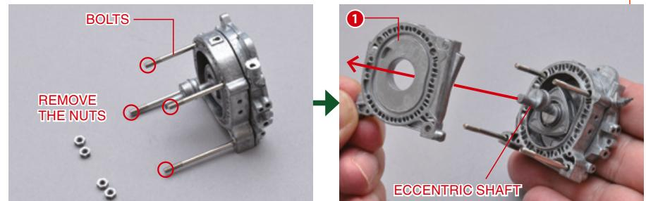
Remove all four nuts from the ends of the bolts.
