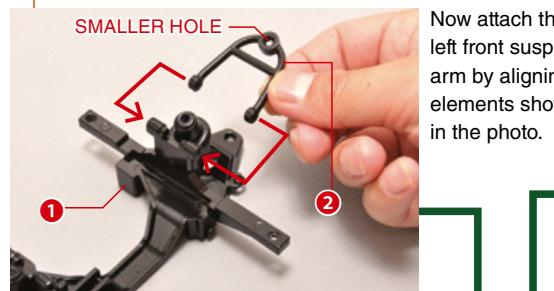
Now attach the upper left front suspension arm by aligning the elements shown in the photo.
