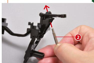
Remove the nut from the end of the piston rod and insert the latter as shown in the photo. Put the nut back on, but don't tighten it completely.
