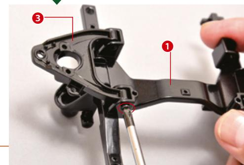
Secure the pieces with one type B screw, using the hole circled in the photo.
