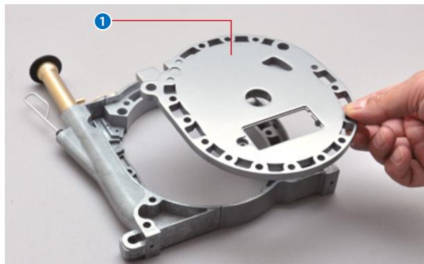
Insert the back plate into the rotor housing, positioning the pieces as shown in the photo. Don't use any screws for now, as this is a temporary assembly.
