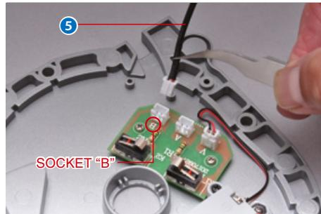
Insert the plug on the electric wire into socket "B" in the control unit.
