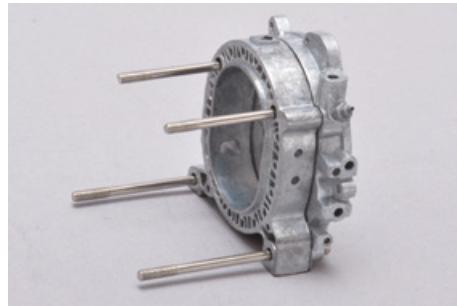
Push the bolts all the way through the back plate of the 1:8 scale rotary engine.
