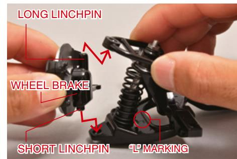
Insert the wheel brake you assembled in Stage 5 into the holes in the left suspension arms. Position the pieces as shown in the photo.
