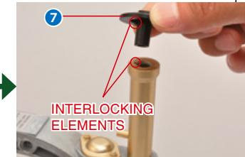
Position the oil filler cap as shown in the photo and insert it into the oil filler tube.
