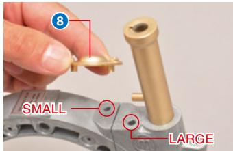
Attach the sealing cap to the rotor housing. Use the photo to help you put it on the right way.
