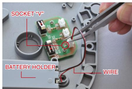
Insert the plug on the wire coming out of the battery holder into socket "V" in the control unit.
