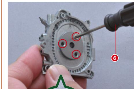
Using the screwdriver provided with this stage, secure the pieces with three type A screws, using the holes circled in the photo.
