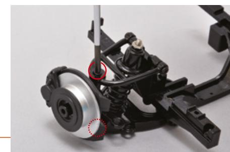
Secure the pieces with two type A screws, using the holes circled in the photo. Don't tighten the screws completely: leave a space of about 2mm for each screw.
