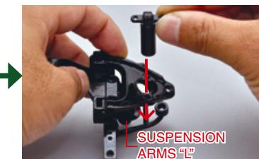
Insert the shock absorber llinchpin into the hole in the housing, as shown in the photo.
