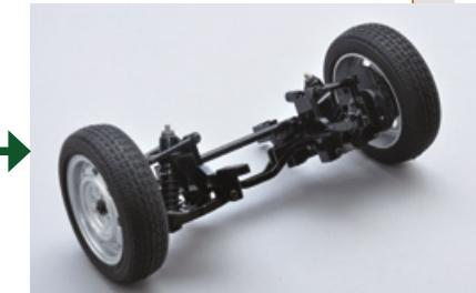
Here are the two wheels mounted on the front suspension. Remember that this is a temporary assembly.
