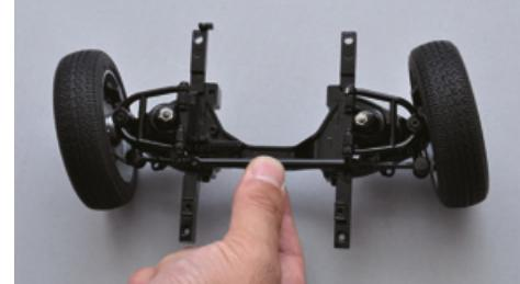
Check that the tie rod works properly by moving it slightly to one side.
