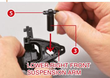
Insert the lynchpin into the shock absorber housing as shown in the photo, and then attach the piece to the lower right front suspension arm.
