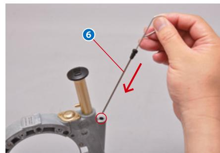
Insert the dipstick into the hole in the rotor housing circled in the photo.
