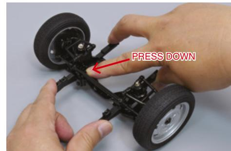
Lightly press down on the chassis to check that the suspension works.
