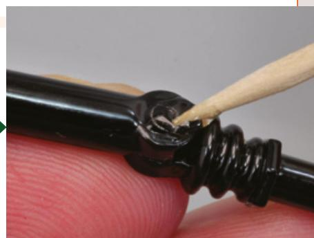
You can apply a small amount of adhesive or glue for screws on one end of the screws in the tie rods to stop them coming out.
