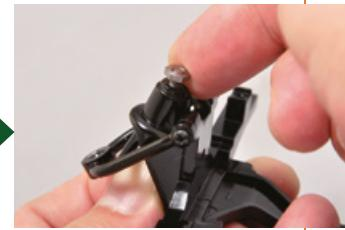
Put the nut back on the end of the piston rod, but don't tighten it completely. You will be adjusting the suspension later on.
