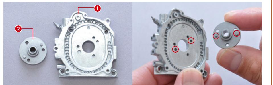
Join the gearwheel R and the rear housing as shown in the photo. The pieces only fit together in one way thanks to the interlocking elements circled in the photo.
