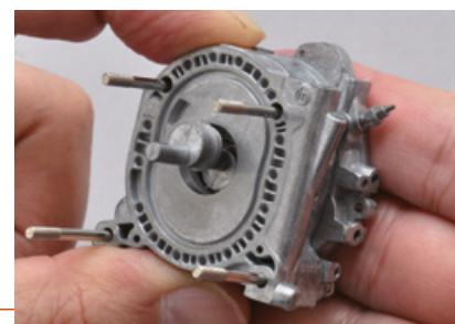
Use the photo to help you position the intermediate housing correctly.
