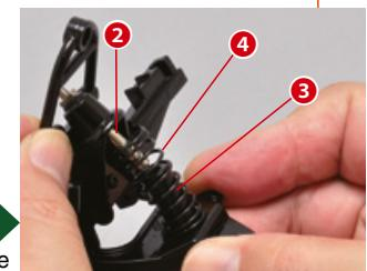
Slide on the coil spring and insert the piston rod as shown in the photo.
