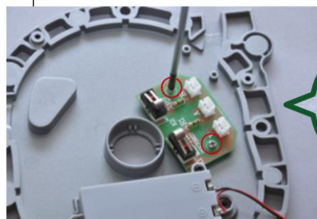
Position the control unit as shown in the photo, aligning the circled holes.
