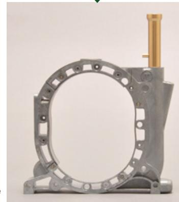
Press the oil filler tube all the way down.
