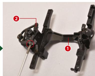
Insert and tighten another type A screw in the other end, as shown in the photo.
