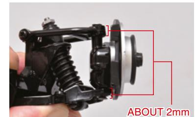
You will be adjusting the suspension later on; the space left will allow the pieces to move sufficiently for the moment.
