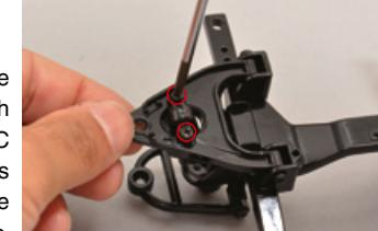
Secure the pieces with two type C screws, as shown in the photo.
