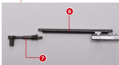
Attach one of the tie rod ends to the tie rod, as shown in the photo.
