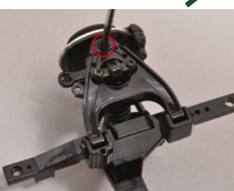
Use two type D screws to secure the pieces. Don't tighten the screws completely: leave a space of about 2mm.
