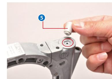
Get the rotor housing you assembled previously and attach the connection of the oil filler tube as shown in the photo.
