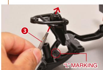
Remove the nut from the end of the shock absorber piston rod and insert the latter as shown in the photo.
