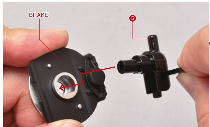
Position the pieces as shown in the photo and insert the hose joint into the brake unit.
