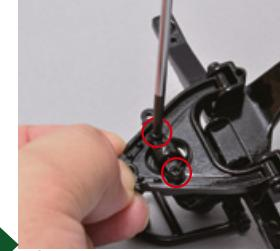
Secure the pieces with two type B screws.
