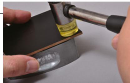
Use the board and hammer to insert it completely.
