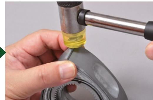
Lightly hammer the three apex seals until they are in the correct position.
