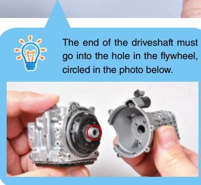
Push it right in. The driveshaft must be in the same position as the one in the photo.
