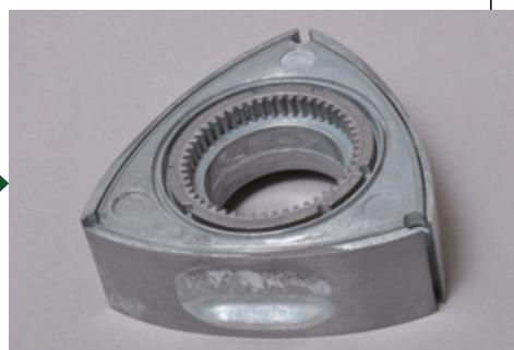
Make sure the edges of the gearwheel and the rotor are flush.
