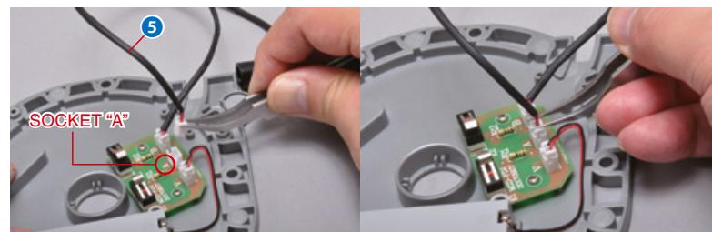
Insert the plug on the electric wire into socket "A" in the control unit.
