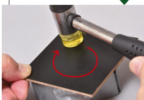
Put the board on top of the rotor and hammer it a few times to insert the gearwheel completely.
