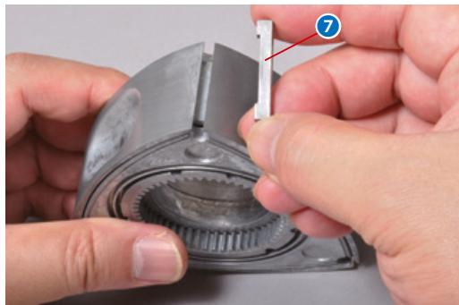
Insert the apex seals into the respective slots in the corners of the rotor.
