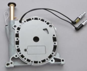
Put the back plate on the rotor housing, ensuring it faces the same way as shown in the photo. The electric wires must come out of the notch indicated in the photo.
