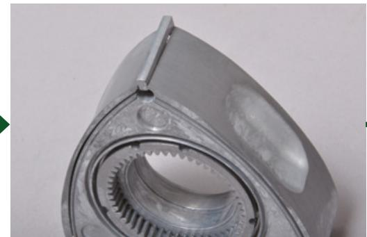
Press all the apex seals into the slots so that no edges stick out of the rotor.
