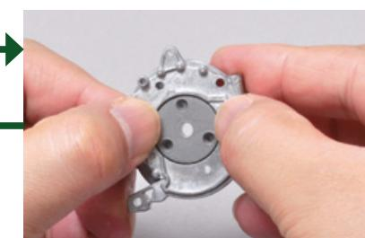
Press the gearwheel all the way down.
