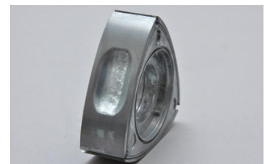
Make sure the edges of rotor A and B are flush.
