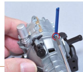
Now attach the air filter mount using the hole you previously removed the screw from.
