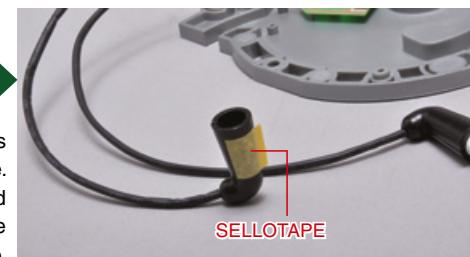
Once your 1:2 scale model of the rotary engine is completed, the control unit will no longer be visible. To distinguish the two electric wires, we recommend you stick a piece of coloured sellotape on the wire you received with this stage.
