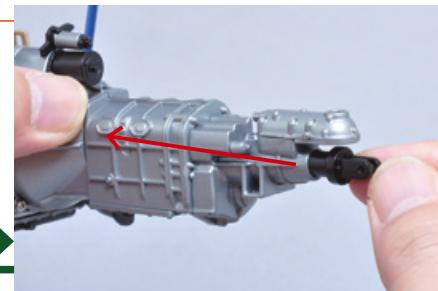
Insert it at the angle shown in the photo. The driveshaft must go into the hole in the flywheel.
