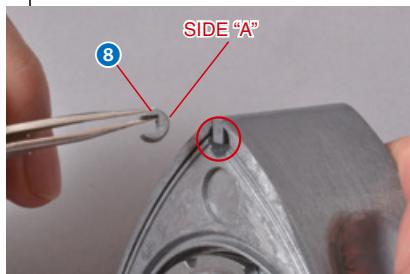
It's time to insert the corner seals. Side "A" must be facing the rotor.
