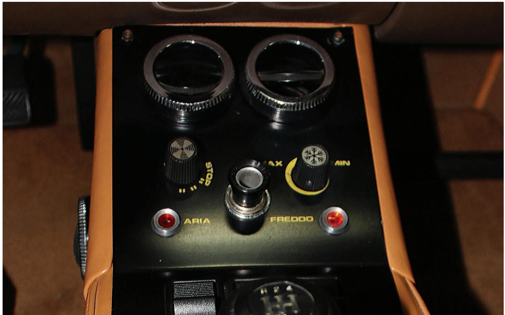
Though later models would feature more sophisticated climate-control systems, complete with digitised temperature displays, Walter Wolf's 1978 Countach used a more basic set-up, with warm or cool air being supplied to the cockpit via a number of circular vents, such as those seen above on the central console panel.
