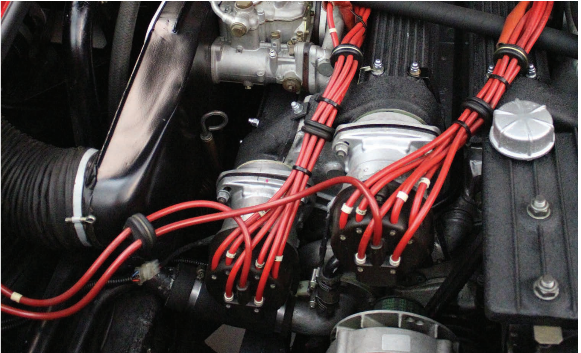
A close-up view of the two distributors on a Countach. The two leads coming in from the left of the picture are the HT leads from the ignition coils, and each distributor serves one bank of cylinders, supplying high voltage to each spark plug in turn in the correct sequence.
