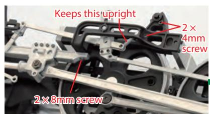
Secure the motion bar to the plate with a 2 x 8mm screw. Secure the motion plate to the motion frame with two 2 x 4mm screws.
