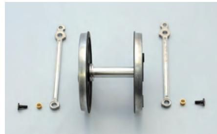
Disassemble the first wheels from Stage 3.
