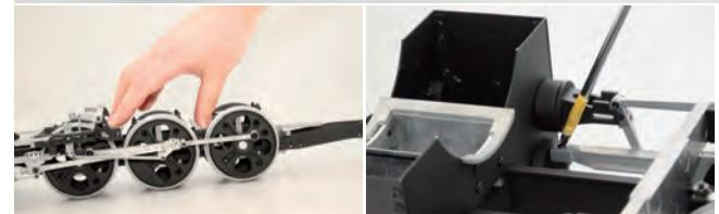
Move the assembly back and forth on a flat surface to test the movement of the wheels. If they get stuck at all, try to identify the cause of the problem. Inspect each part, in particular the screws in the motion bar, as they may be loose. Tighten them if they are.
