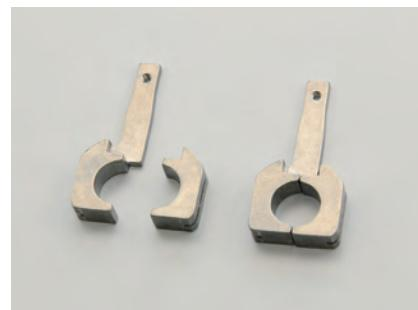
Assemble axle boxes A and B as shown above. Complete the four sets.
