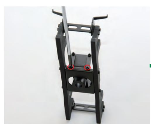
Tighten a 2 x 3.8mm stepped screw into the aligned holes.
