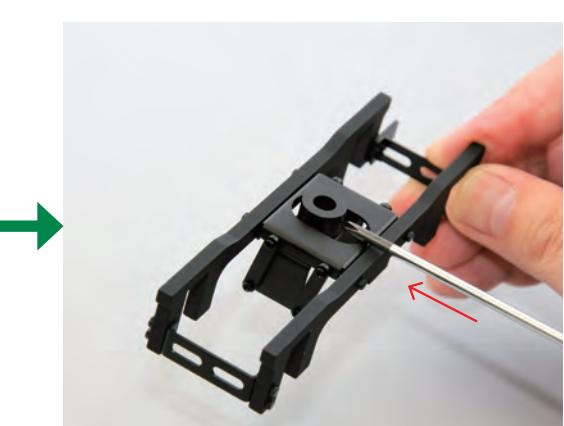
Push the cylindrical part of the mount towards one side of the truck frame to test the movement of the links.
