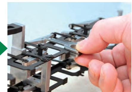
Take one of the axle boxes and slide it up into the gap in the underframe, positioning the frame in the grooves at the side of the axle box.
