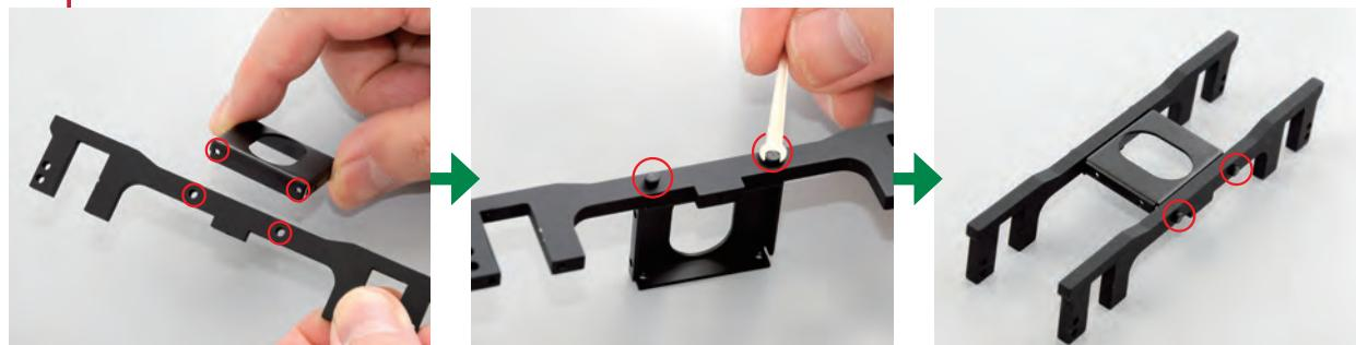
Align the holes in the centre beam with those in the truck frame.
