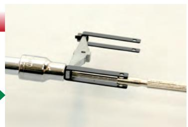
Place the links over the ends of the springs and pass a screw up through the aligned holes. Tighten a nut onto the end of the screw. Repeat this process, following the photo in the previous step to assemble all the leaf springs.
