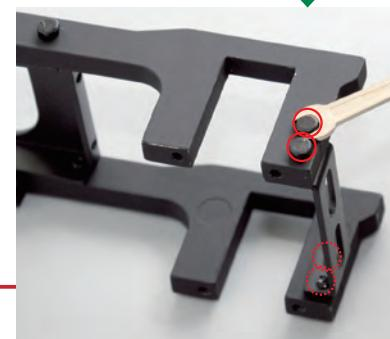
Place the bracket between the frames, align the holes and half-tighten a  $2 \times 6\text{mm}$  hex screw into them.
