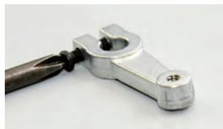
Tighten a 2 x 7mm screw into an eccentric arm, as shown.
