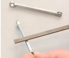
Check the connecting rods for any flash. Remove any you find with a file.
