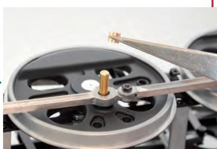
Place the hole at the rear of the coupling rod over the pin projecting from the second wheel, then place the bush (Stage 22) between them. Repeat this step for the other side of the model.
