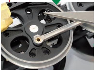
Align the hole in the coupling rod with the hole off-centre of the first wheel. Insert a bush into the hole in the rod and then place the rod pin into the bush, then tighten it into the wheel. Do this for the third wheel as well.
