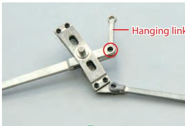
Fit a hanging link at the end of the left radius rod and secure with a  $2 \times 3.6\text{mm}$  set screw (circled).
