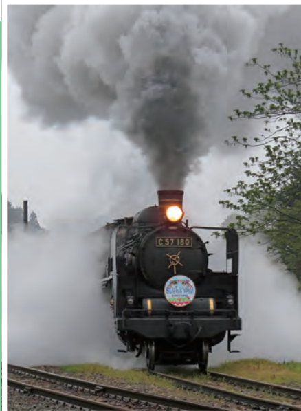
Here you can see a C57 underway with its drainage pipes fully opened, discharging the water from the cylinders.
