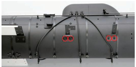
Now fit the other two supports, again tightening the screws lightly to allow for adjustment.
