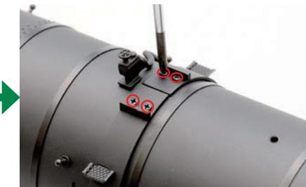
Repeat for the right step seat, then secure both with two 2 x 3mm screws in the four circled holes.
