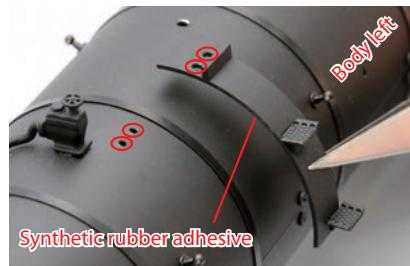
Brush the reverse of the left step seat with SRA and press to the left side of the boiler, lining up the circled holes.
