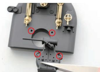
Align the holes in the firebox door with those in the backhead, as shown.
