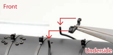
Take one of the tube receivers and fit it onto the tips of tubes A and D, as shown.
