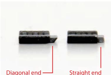
Note the differences between the left and right boiler side steps.
