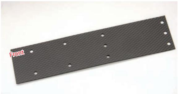
Familiarise yourself with the front left running board, noting the positions of its holes and which are the top and bottom sides (the top has raised, criss-crossing ridges on it, creating diamond-shaped recesses, while the bottom is the reverse of this).
