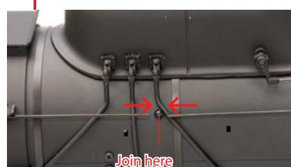
The two handrails will meet inside the bracket shown here.
