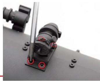
Tighten a  $2 \times 3\text{mm}$  screw into the four circled holes.
