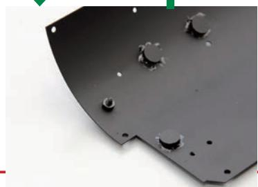
Fit the second handrail bracket in the same way. Before the glue dries, make sure the holes of the brackets are aligned.
