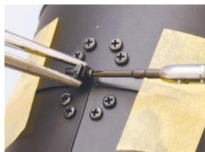
To secure the bands, hold in place with masking tape and fasten with a 1.4 x 6mm screw and a M1.4 nut, which you can hold in place with pliers.
