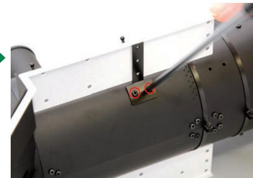
Tighten two 2 x 3mm screws into the circled holes. Do this lightly at first, to allow for adjustment later.
