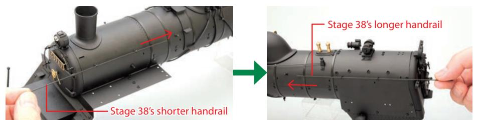
Take one of the shorter handrails from Stage 38 and feed it through the handrail brackets from the front.
