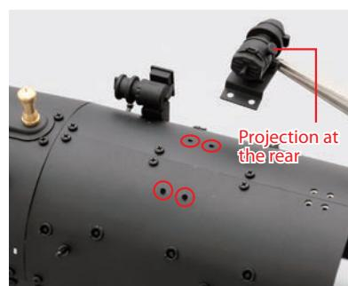
Align the holes in the generator with those in the top of the firebox.
