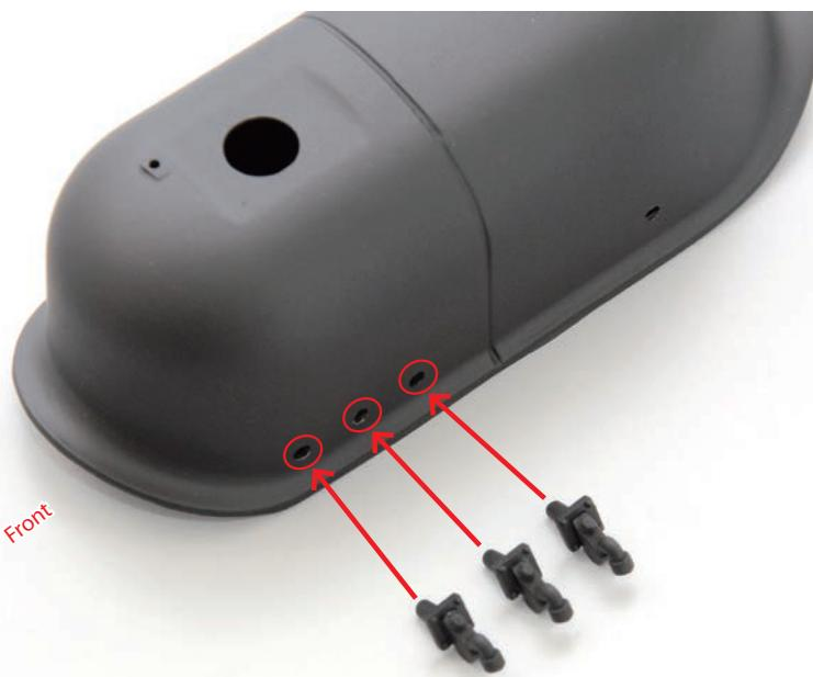
Test-fit the six sand spreader pipe main cocks into the holes indicated (there are three more on the other side).
