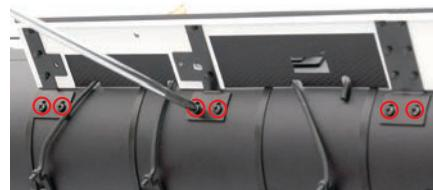
Return and tighten the supports' screws fully.
