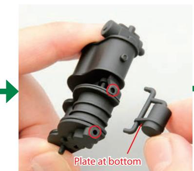
Now line up the regulator as shown (note the location of the lower plate) and use SRA to fit it into the circled holes.
