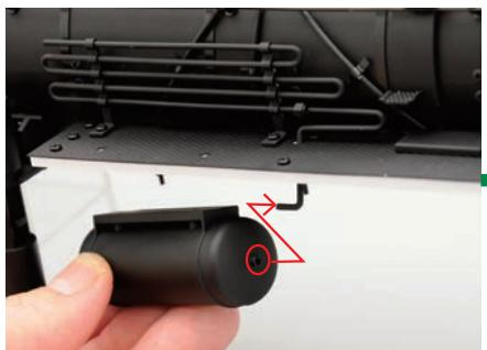
Line up the right air reservoir to the underside of the running board. The hole in its front should accommodate the tip of the cooling tube.
