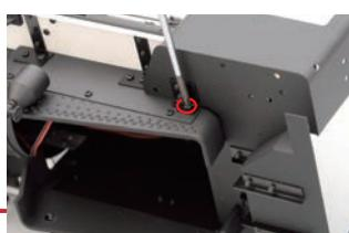
Also tighten a 2 x 3mm screw into the side hole.
