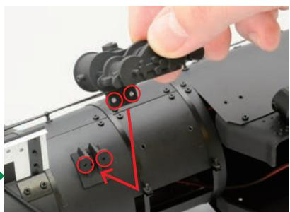
Line up the compressor assembly to support A. Support B will fit to the underside of support A.
