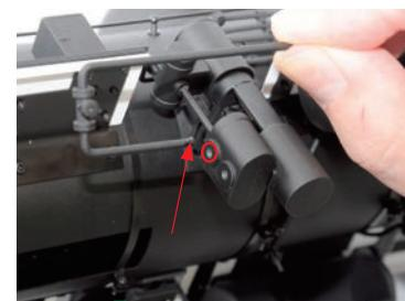
Dab some SRA to the indicated tip of the pipe, and fit to the circled hole on the water supply pump assembly.
