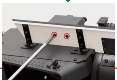
Secure with two 2 x 4mm screws.
