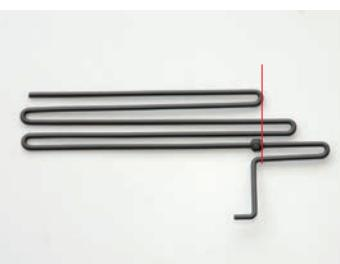
The joint should be level with the upper bend in the tube, as shown.
