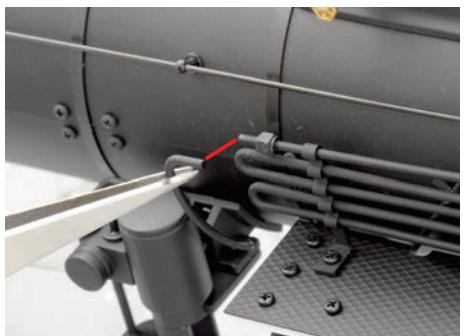
Now dab the other tip with SRA, and line up to the free end of the air cooling tube A.
