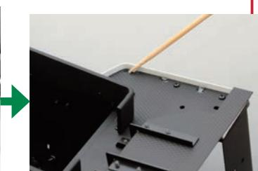
Reinforce the join along the underside of the cab floors with a few spaced dabs of SRA.
