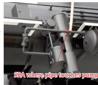
Now dab a very little SRA to the inside of the indicated length of pipe and set to the pump's side.
