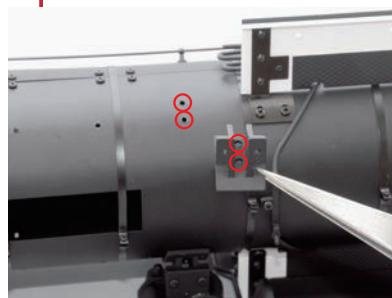
Line up the pump support, as shown, to the holes on the right underside of the body.
