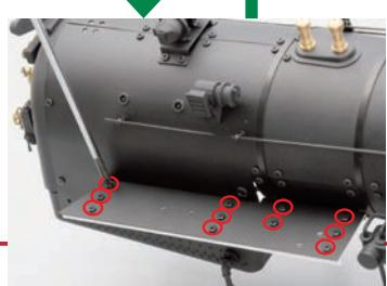
Join the parts and secure to the supports using 2 x 3mm screws.
