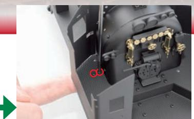
Hold the stay in place and secure with 2 x 3mm screws, from the top.
