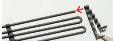
Now take the air cooling tube supports and slide them onto the tube as shown.
