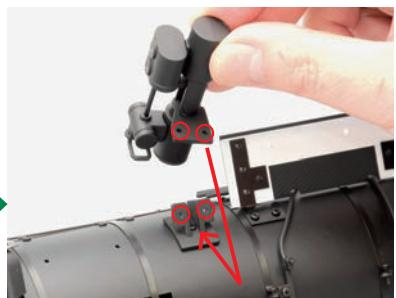
Fit the water pump assembly under the support.
