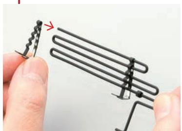
Slide the two air cooling tube supports over the tube, then press them together with your fingers to clamp it to the tube.
