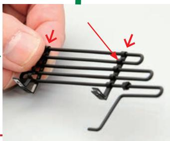
Make sure each coil of the tube is held in one of the supports' rings.
