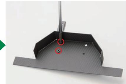
Secure with two 2 x 3mm screws – but only lightly at this stage to allow for adjustment later.
