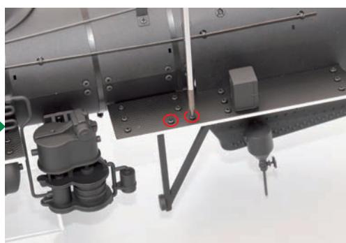
Secure (from the top) using two 2 x 4mm screws.
