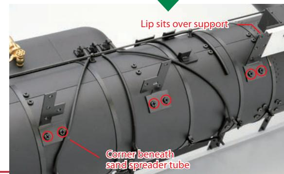
Line up running board supports A, B and C as shown, noting their differing shapes.
