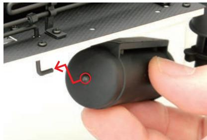
Next, line up the left air reservoir to the underside of the left running board. Fit the tip of the air cooling tube into the recess in its front section.
