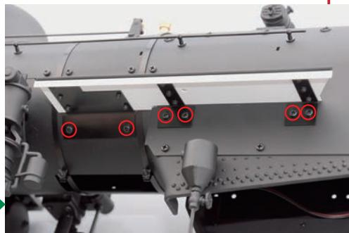
Once in place, return to fully tighten the supports' screws.
