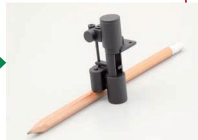
Use a pencil (or similar) to rest the assembly vertically, then leave to dry.
