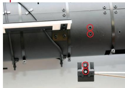
Now line up compressor support A to the circled holes on the left side of the body.
