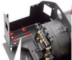
Place this on the inside-left side of the cab, matching the circled holes.
