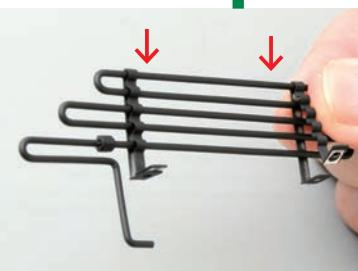
Slide the tube end shown into the indicated hole in the left running board.
