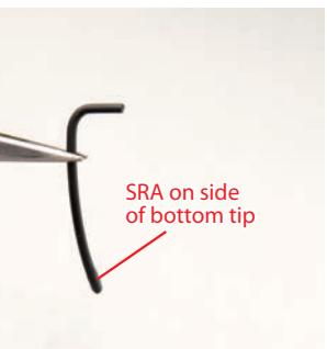
Now take the air cooling tube (right B) and dab the **side** of the marked tip with SRA.
