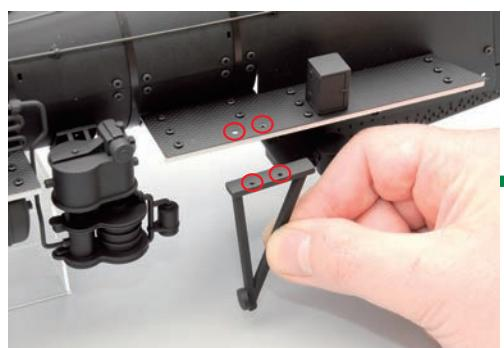
Now join the coupling gear to the underside of the running board.
