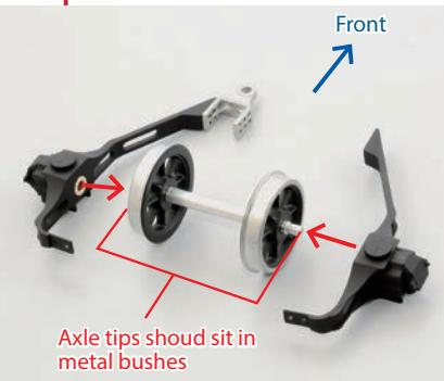
Now join the trailing truck end beams together, pushing the bushes onto the ends of the trailing wheels' axles.
