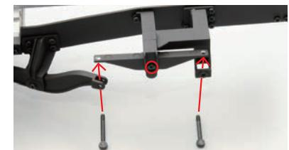
Turn the underframe back over, and line up the parts shown: a long link joining the equaliser and a medium link on the far side to that.
