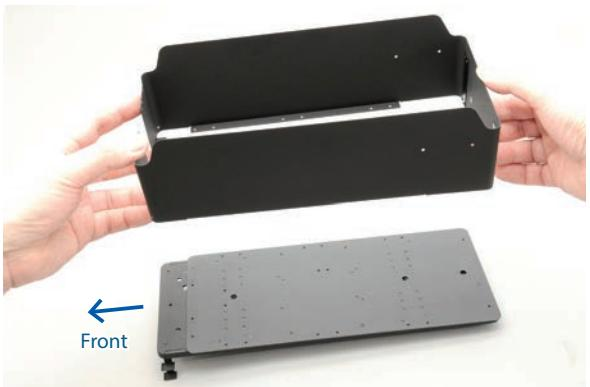
Now line up the tender wall assembly with the top of the tender base.
