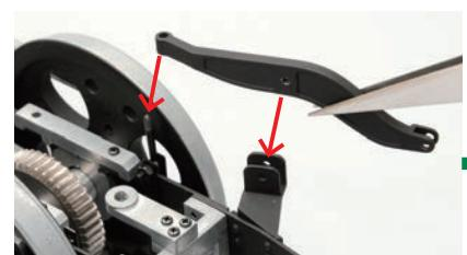
Now take the left equaliser and, orienting the part exactly as shown, lower it into place.
