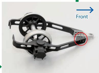
Use six more 2 x 3mm screws from Stage 65 to secure the parts. Do this lightly at this stage.
