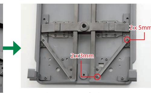
Repeat the process to fit the medium member B, again noting the corresponding sizes of screw to use.
