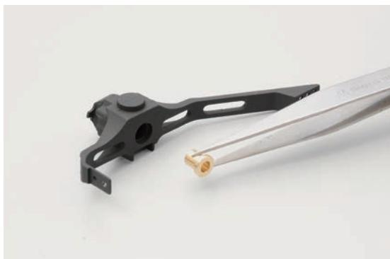
Use SRA to fit one of the wheel bushes into the hole on the inside centre of the left trailing truck beam, positioning the part as shown.
