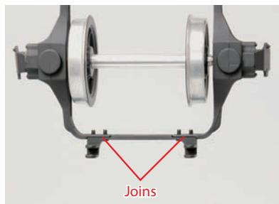
Ensure the indicated joins are flush when tightening.
