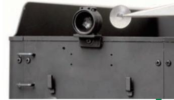
The rear headlamp's lens will fit to its housing with the inlaid pattern running vertically. Use PVA glue (which dries clear) to fit this.
