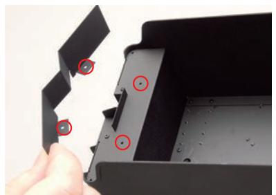
Now add the front tender wall B to the top of part A, aligning the circled holes.
