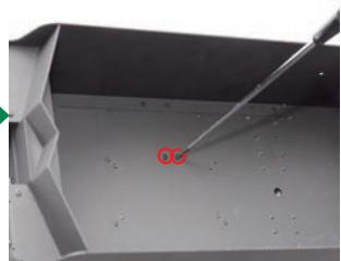
Use 2 x 4mm screws to secure the part, from the inside of the tender.
