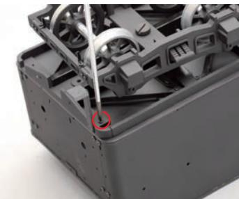
Turn the tender upside down and fit one of the rear step sub-assemblies to its bottom corner using a 2 x 7mm screw, as shown.
