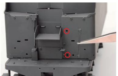
Use SRA to fit the water level gauge to the circled holes. It does not matter which way round the part goes.
