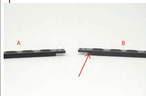
Differentiate between the traverse beams A and B by locating the holes on the side of the single beam B.
