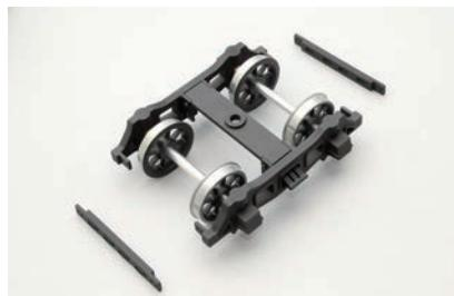
Repeat the work of Step 3 to fit the remaining two traverse beams A to the other tender truck.
