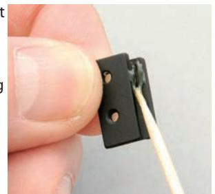
Remove the bracket and dab SRA onto the tab on the part's left/inside edge.
