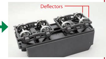
Now repeat for the rear truck – making sure the end with the deflectors is facing the rear.
