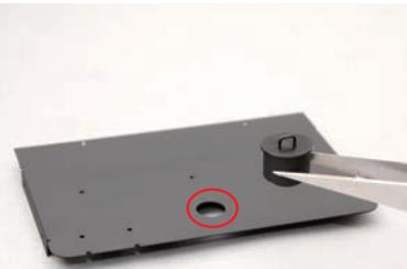
Position the rear upper tender plate on your work surface as shown, then use SRA to affix the water inlet to the circled hole.
