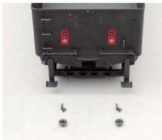
Now use SRA to fit the four handles to the pairs of circled holes. If those on the left are tight, you can loosen the arrowed screws. The handles should sit at a distance of 2mm from the rear tender wall.
