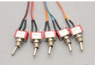
Turn the nuts onto the threaded part of the switches to about two thirds of the way in.
