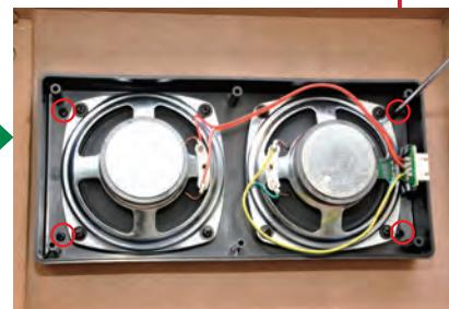
Use four of the speaker screws to secure it.
