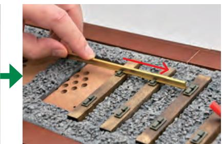
The rails will be fitted by sliding them through the fasteners, one by one.
