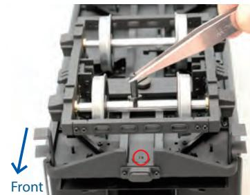
Turn the tender upside down and fit the drawbar pin into the circled hole using tweezers. You can remove the front truck to make this easier.
