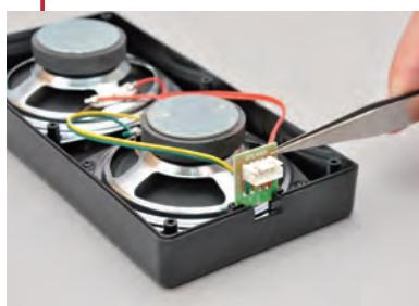
Use tweezers to slot the speaker's circuit board into the mount at the end of the speaker housing.
