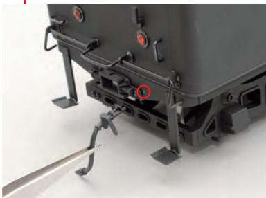
Fit the brake hose, positioned as shown on the rear of the tender, into the circled hole and secure with SRA.
