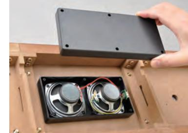
Lower the speaker cover onto the speaker. It does not matter which way round it goes, but be careful not to trap any wiring.
