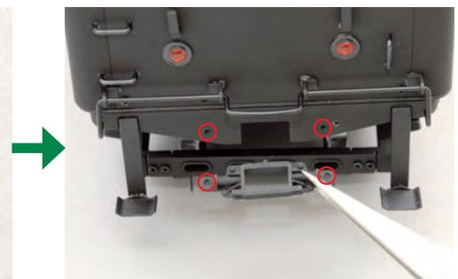
Line the part up to the circled holes at the rear of the tender.
