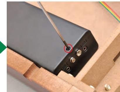
Now use the smaller-headed 2.3 x 8mm) screws from Stage 89 to secure the lid.
