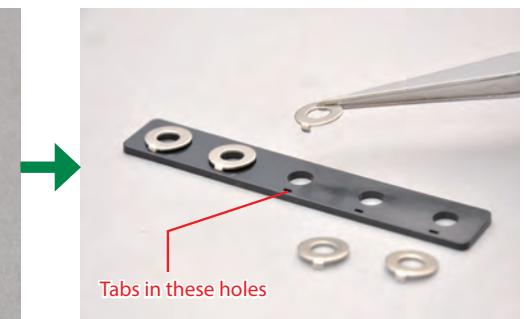
Lay the switchboard with its flat face down, then fit the washers to it as shown above.
