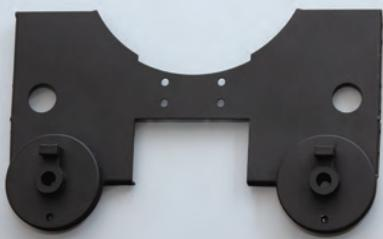
Fit the second cylinder cover to the cylinder rear plate in the same way as the first. Remove any excess glue from around the covers before they dry.
