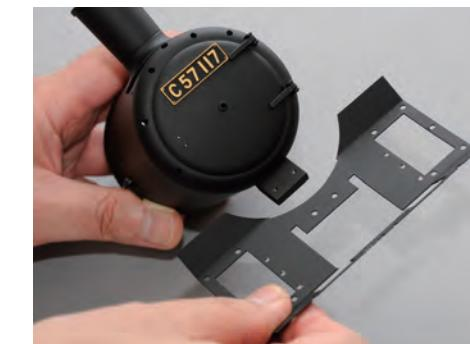
The front deck base fits onto the projecting tab at the bottom of the smokebox.
