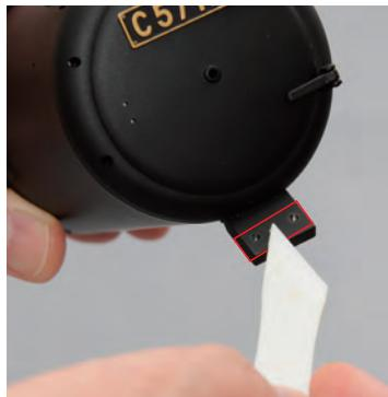
Remove the deck base and apply some multi-purpose adhesive to the tab.
