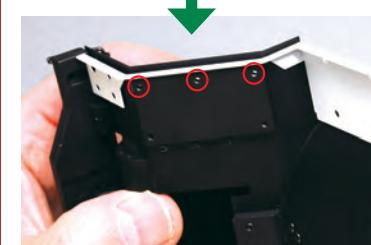
Align the three holes of the deck side with those in the front deck and inspection lid.
