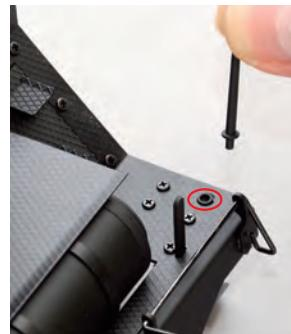
Glue the second grab bar into the hole on the right-hand side of the front deck.
