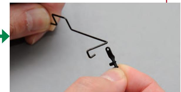
Place the four release levers onto the release lever bar, alternating their order, as shown below.
