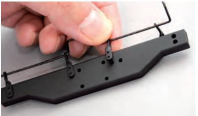
Insert the pins of the lever into the corresponding holes in the front end beam. Then repeat for the other three levers.
