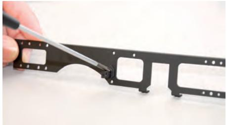
Fit the brake supports to the underframes with  $2 \times 3\text{mm}$  screws.
