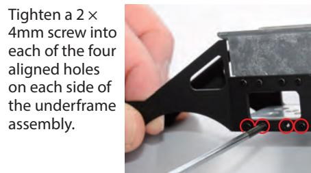
Tighten a  $2 \times 4$ mm screw into each of the four aligned holes on each side of the underframe assembly.
