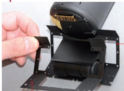
Place the front deck upper plate (Stage 5) onto the front deck.
