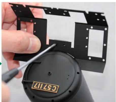
Align the holes of the deck with those in the tab. Half-tighten a 2 x 4mm screw into each hole.
