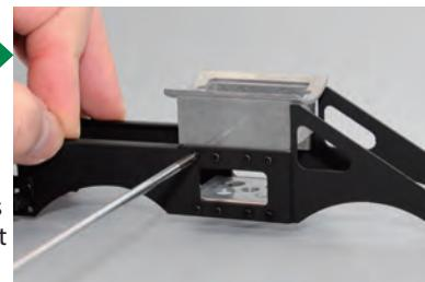
Check all the screws and tighten any that are loose.
