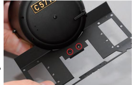
Test-fit the front deck base onto the tab, aligning the circled holes of both.
