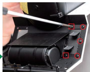
Tighten three  $2 \times 3\text{mm}$  screws into the holes at the side of the deck (circled) and then fully tighten the screws in the two inner holes (marked here with squares). Repeat this for the front right deck side.
