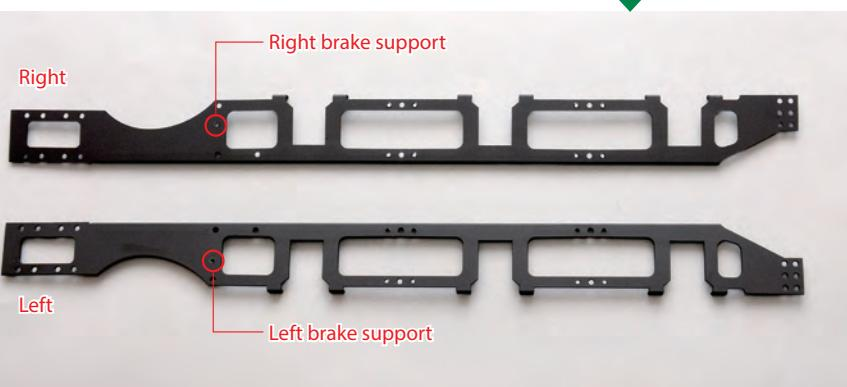
The right brake support fits to the right main underframe at the circled point, and the left brake support fits to the left main underframe at the circled point.
