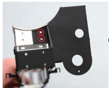
Align the holes of the left cylinder front plate with those in the smokebox support.
