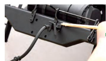
Place the air hose into position and remove any excess adhesive.
