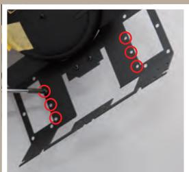
To avoid the screwdriver damaging any of the adjacent surfaces, you can cover the shank with masking tape, as shown.
