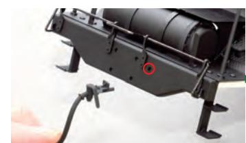
Test-fit the air hose into the circled hole in the front beam.
