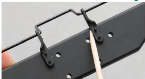
If any excess adhesive is visible on the front end beam around the levers, use something pointed – such as a toothpick – to remove it before it dries.
