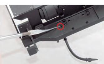
Apply a small amount of instant adhesive to the air hose from the back of the front beam.
