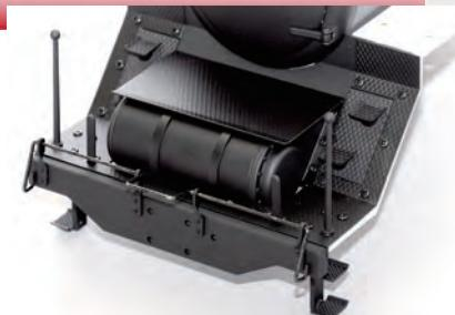
Glue one of the grab bars into the circled hole on the left-hand side of the front deck with multi-purpose adhesive.
