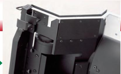
Push the projection in and then align the holes.
