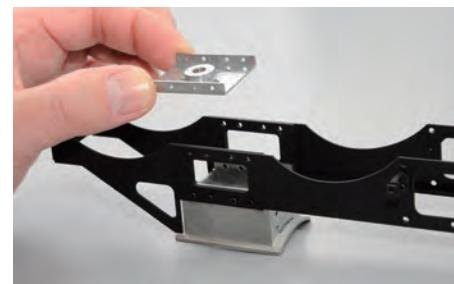
Turn the underframe assembly over and place the truck support between the sides, below the smoke chamber support.
