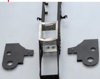
The cylinder front plate is divided into two parts. The front faces of the plates are flat.
