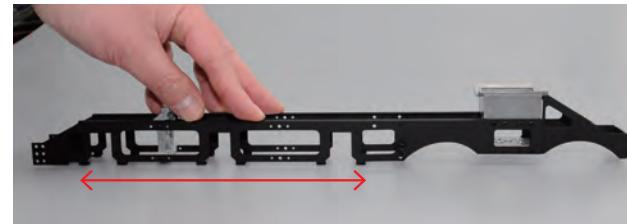
Place the underframe on a flat surface, as shown, and lightly press down on the top. Check that the bottom is resting flat in the area between the arrowheads.
