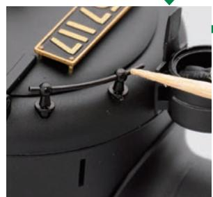
Fit handrail A and the three brackets in the same way as B. Remove any excess adhesive from the rails and brackets.
