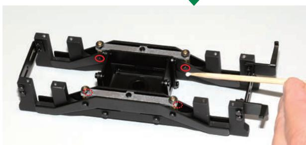
Loosen the hex head screws slightly and then apply some PVA glue to the ends of them.
