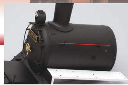
Align the holes of the handrail brackets before the adhesive dries.
