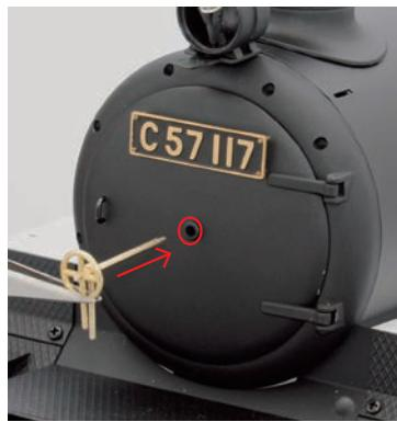
Pass the end of the handle into the hole in the centre of the smokebox door.
