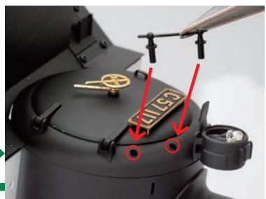
Apply synthetic rubber adhesive to the ends of the two brackets holding handrail B, and insert them into the two holes (circled).
