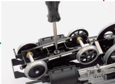
Tighten the centre pin into place.
