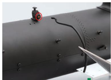
Apply a small amount of synthetic rubber adhesive to the end of the water supply pipe and insert it into the hole in the valve.
