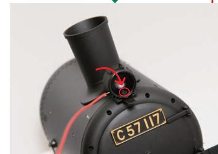
Align the end of the cable with the hole in the headlamp.
