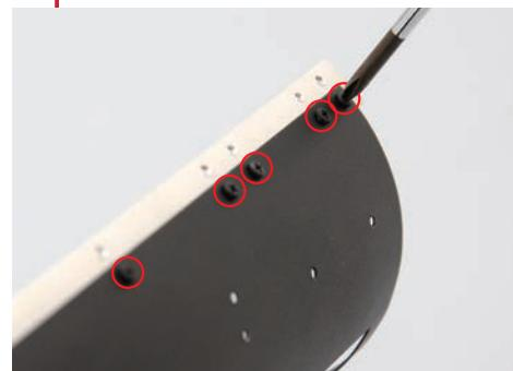
Fix the second boiler joint to the other side of the lower boiler half with seven 2 x 3mm screws.
