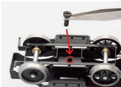
Pass the centre pin (Stage 28) down through the aligned holes.
