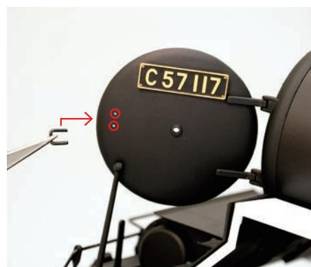
Insert the handle into the two holes on the smokebox door.
