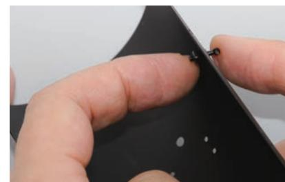
Apply some synthetic rubber adhesive to the inside of the boiler half at the base of the bracket, and tighten a nut onto the end of it.
