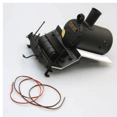
Prepare the LED cable by removing the cable tie. Straighten the end of the cable that does not have the LED on it.
