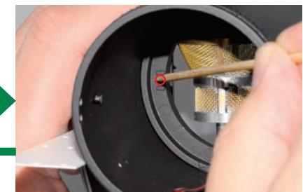
Apply some epoxy adhesive to the space between the ridges.
