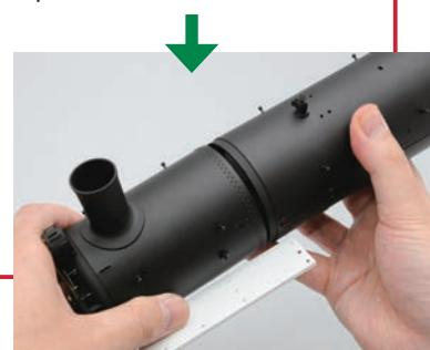
Insert the boiler joint into the rear of the smokebox.
