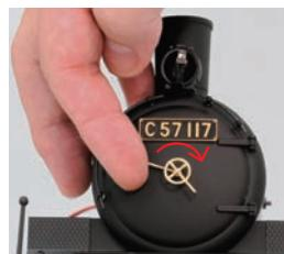
When the lever is rotated the lock on the inside of the smokebox turns in the hole in the centre of the lock bar, holding the door shut.
