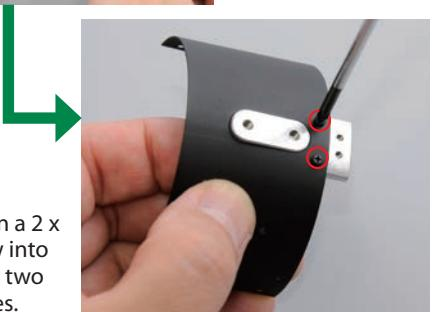
Half-tighten a 2 x 3mm screw into each of the two circled holes.
