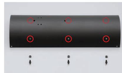
Locate the six holes on the left and right of the boiler upper half. Prepare six handrail brackets and six nuts.
