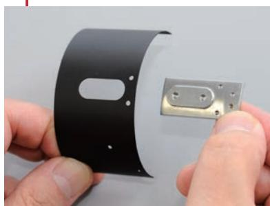
Place the safety valve base on the inside of the boiler section, aligning the circled holes.
