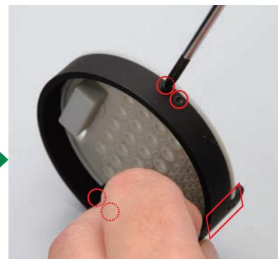
Tap the four holes in the sides of the joint (circles) with 2 x 3mm screws.
