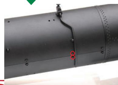
Adjust the position of the water supply pipe so that it is in front of the two circled screws.
