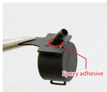
Apply a small amount of epoxy adhesive to the base of the headlamp (circled, above).
