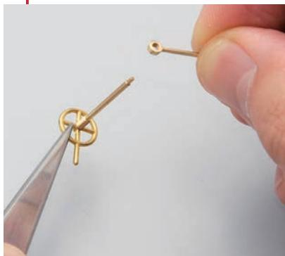
Insert the end of the smokebox handle into the hole in the lever.
