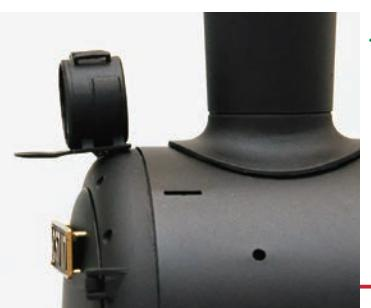
Adjust the position of the headlamp to match the one shown here. Make sure it's aligned centrally with the smokebox.
