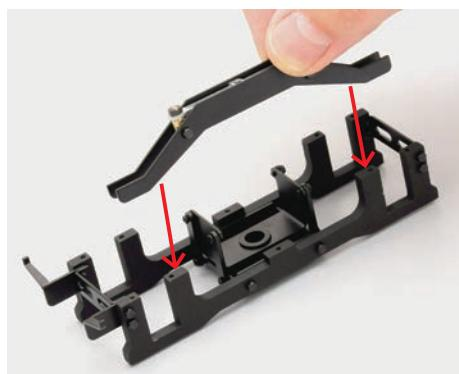
Place the assembly over the side frame of the leading truck, with the equalisers either side of the frame.
