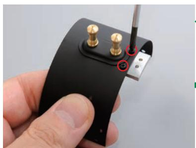
Screw the two safety valves into the holes in the cover and base.
