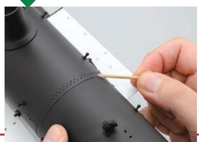
If any synthetic rubber adhesive comes through the seam between the smokebox and boiler, remove it with a toothpick.
