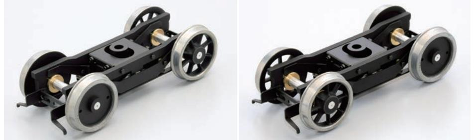
Make sure that when you are fitting the wheels of the leading truck that you have the spoked wheels at the rear (above left).
