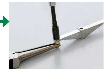
Pass the threaded part of the link through the hole in the leaf spring, and tighten a nut onto it.
