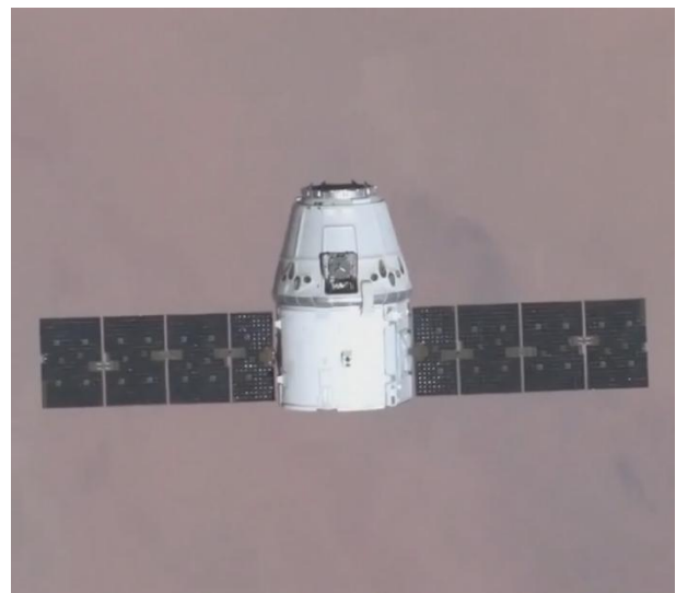
Figure 5: Both of Dragon's Solar Arrays Fully Deployed as seen from the ISS
