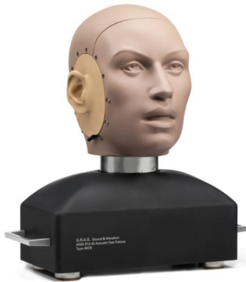
Figure A-1. G.R.A.S. 45CB acoustic test fixture.
