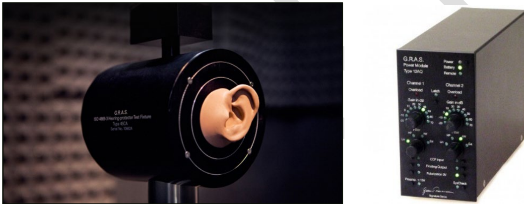
Figure B-1. Left: The G.R.A.S. 45CA ATF with pinna suitable for self-noise testing of electronic hearing protection devices; Right: A G.R.A.S. 12AQ preamplifier with variable gain
