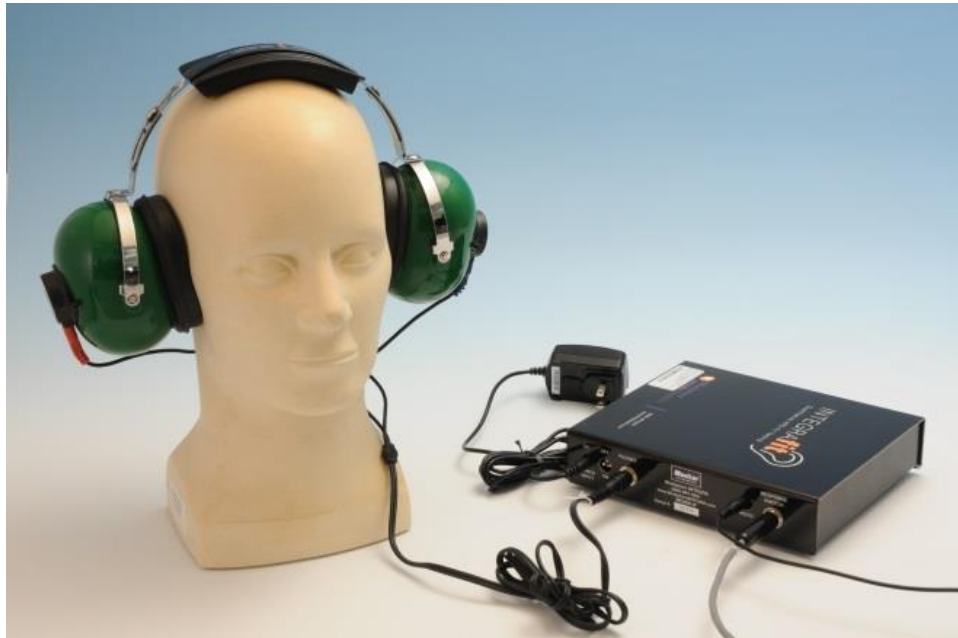
Figure 6. INTEGRAfit ® control box and circumaural noise-isolation headphones.
