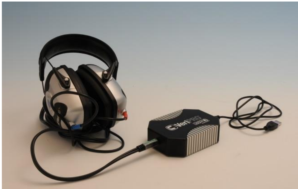
Figure 7. VeriPRO® control box and circumaural noise-isolation headphones.
