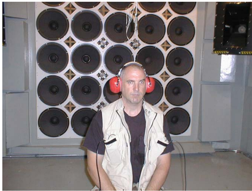
Figure 6: AFRL’s high intensity reverberation chamber – 142 dB max overall sound pressure level capability
