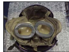
Figure 13: Hard, Creased Earcup Cushions and Missing Earcup Foam Inserts
