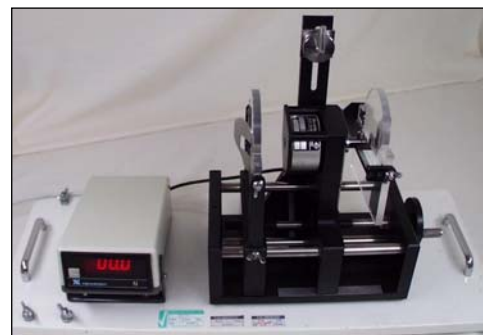
Figure 8: Inspec Laboratories Ltd Tension Rig to Measure Earmuff Headband Clamping Force
