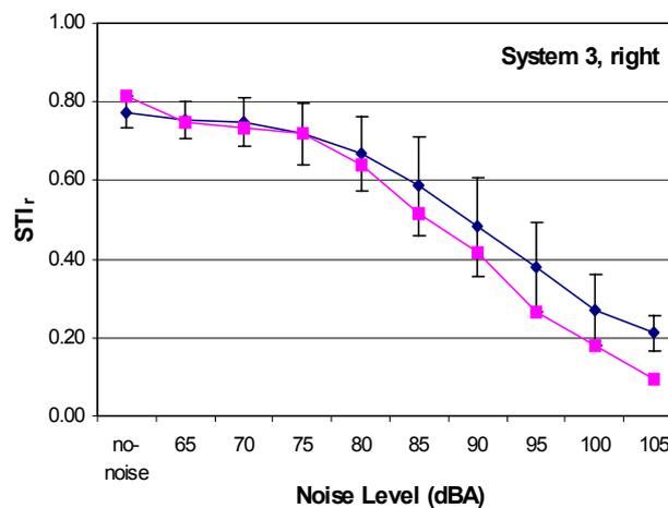
Figure 19. STI<sub>r</sub> as a function of the background noise level for system 3 (right earcup).
