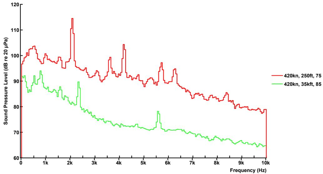
Figure 5 Cockpit noise in Harrier illustrating the compressor fan tone.
