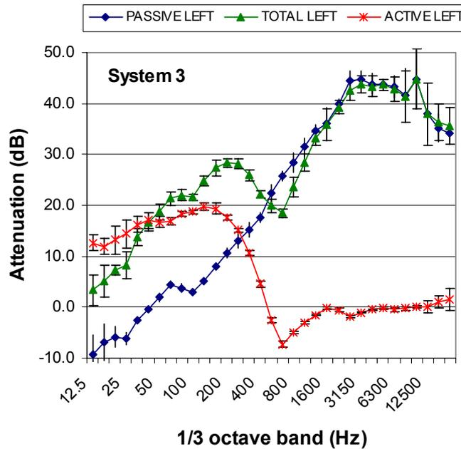
Figure 13. Example of the total, passive and active attenuation of headset 3 as a function of frequency. The curves present the mean attenuation obtained for 5 replica's of the same subject and the left earcup. The vertical bars indicate the standard deviation.
