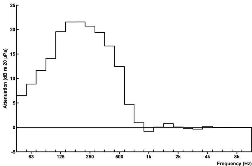
*Figure 10 The active attenuation performance afforded by a helmet mounted ANR system*
