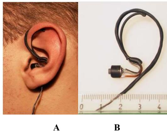
Figure 5. Microphone configuration used for the MIRE-method.
