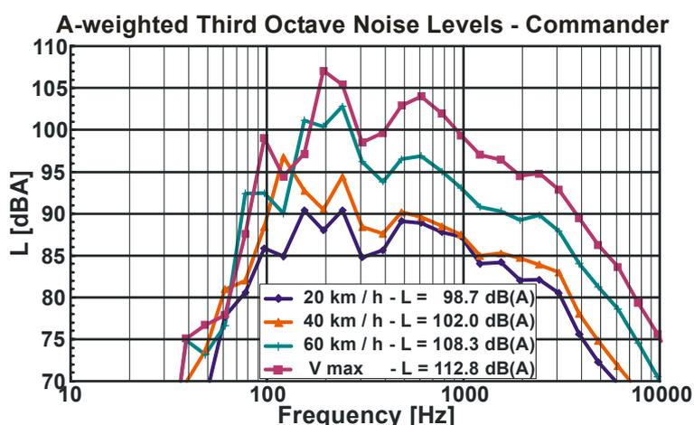
Figure 2: Typical A-weighted noise inside an armoured vehicle
