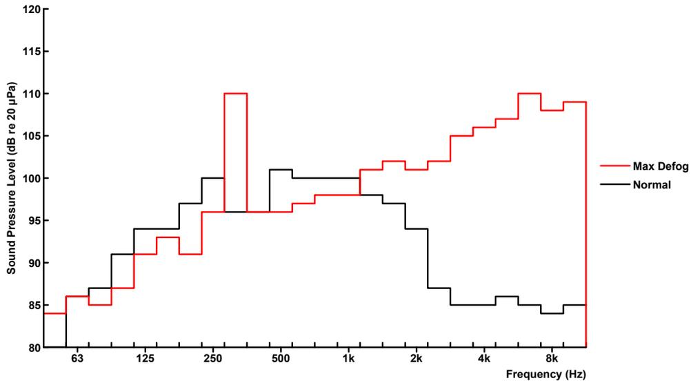
Figure 3 A comparison of cockpit noise in the F-16A with ECS switched on and off
