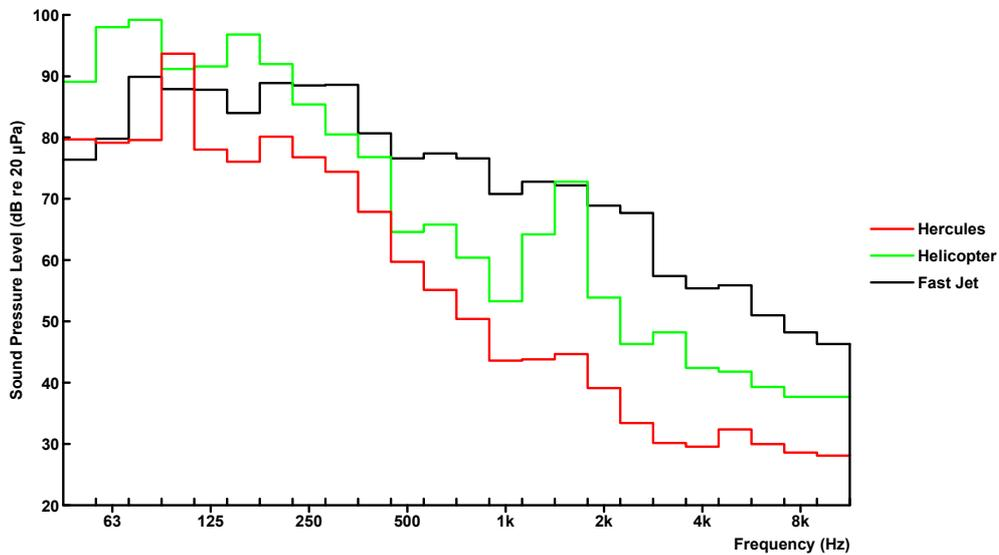
*Figure 9 Typical noise levels at the ear experienced in fast jets, helicopters and Hercules*
