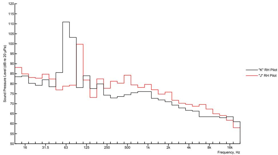
Figure 7 Cockpit noise in the C130K and C130J variants of the Hercules
