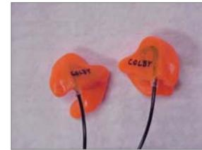
The substantial increase in attenuation (see Figure 10) was achieved by taking deep impressions of individual earcanals and molding the plug to the second bend in the earcanal. This approach required special methods and training for taking the impressions. The ear dam had an integrated silicone pressure relief tube. This tube helped the pressure equalize behind the impression and the ear dam, and substantially reduced the number of hematomas which occasionally occur with deep impressions.
