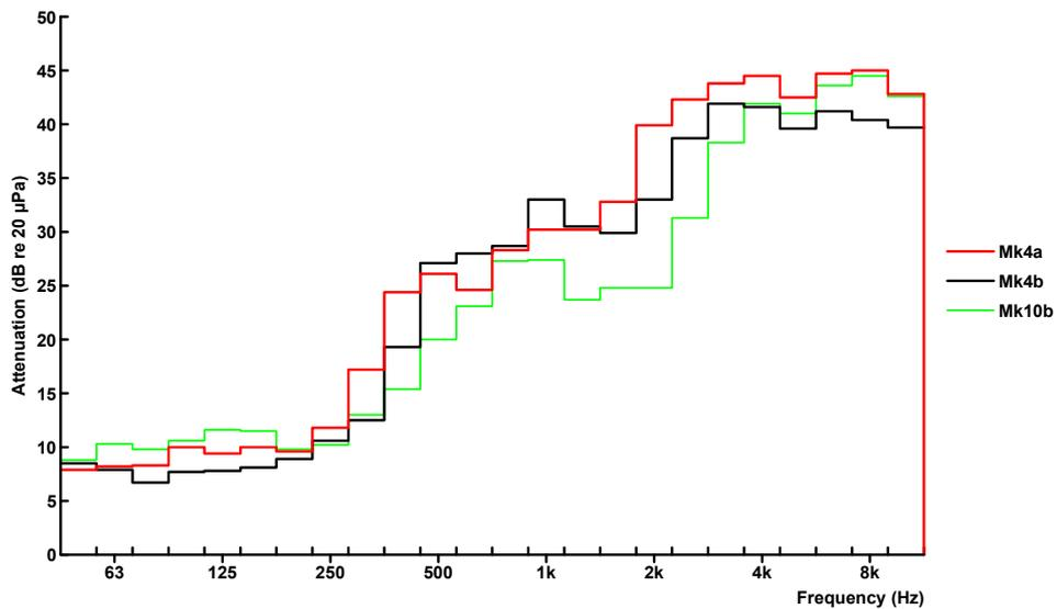
Figure 8 The attenuation characteristics of the Mk4 and Mk10 flight helmets
