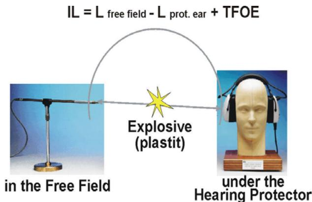
Figure 9. Measuring set-up for the attenuation measurement by using explosive charges.
