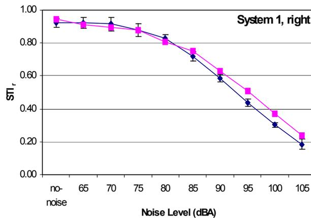
Figure 18. STI<sub>r</sub> as a function of the background noise level for system 1 (right earcup).
