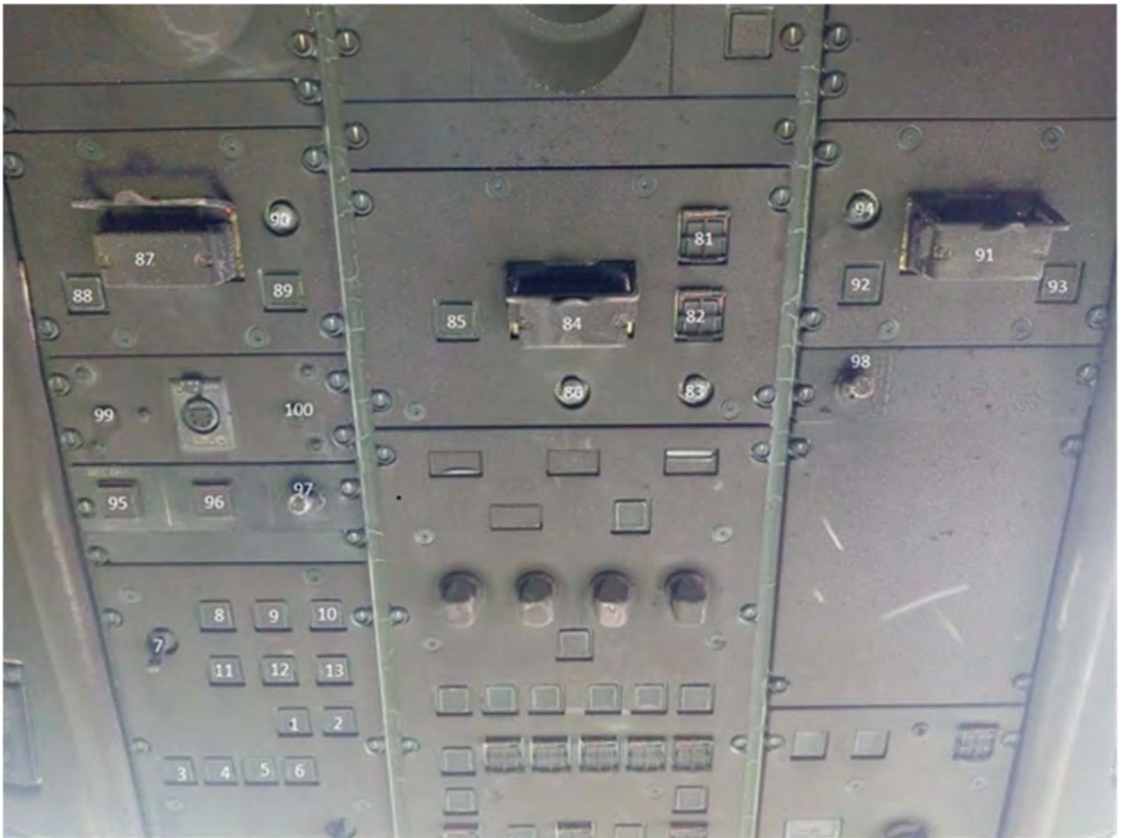
Fig. 21. Engines and APU fire extinguish systems switch condition after the accident
