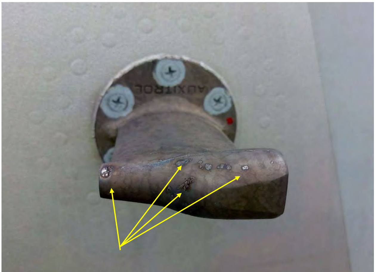
Fig. 24. Lightning strike traces on the right temperature probe
