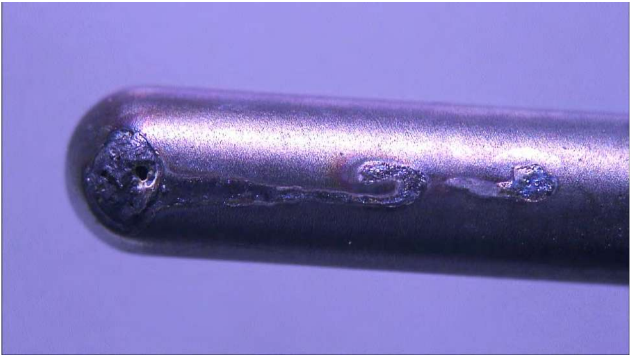
Fig. 25. Lightning strike traces on the right ice detector
