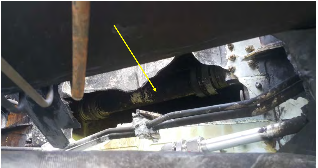
Fig. 16. The hole in the right-side wing spar web (pointed with an arrow)
