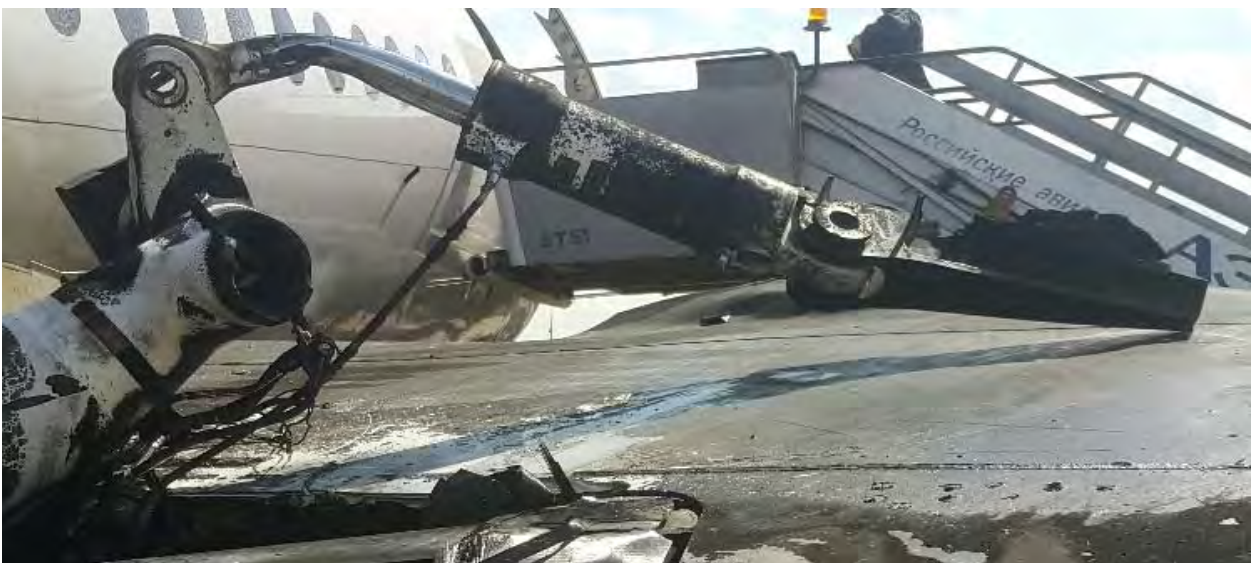
Fig. 15. External view of the cylinder of the right main landing gear
