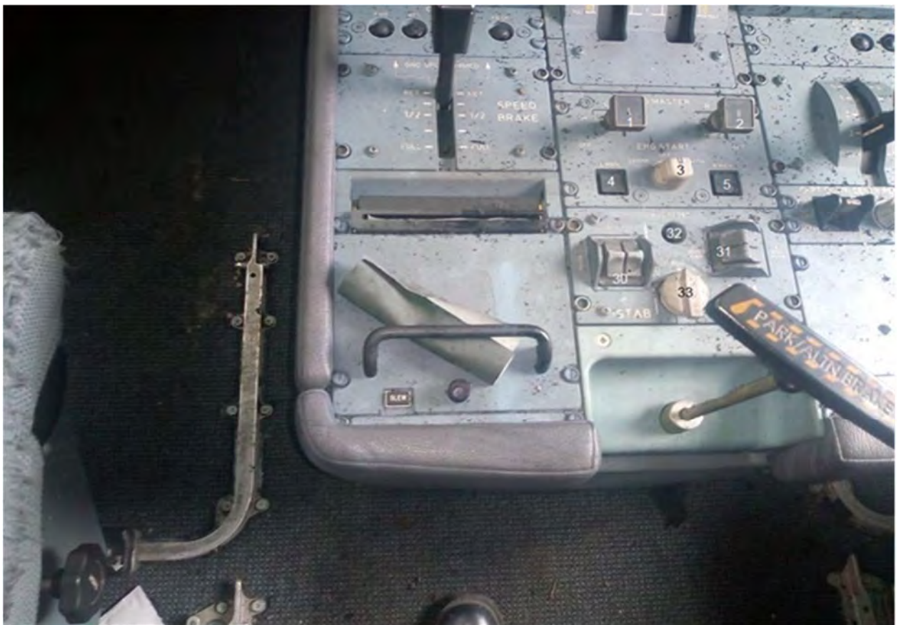
Fig. 20. Engine control switch after the accident
