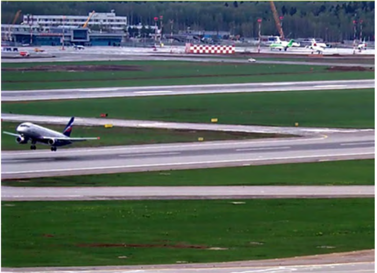
Fig. 36. The aircraft bounce after the second touchdown
