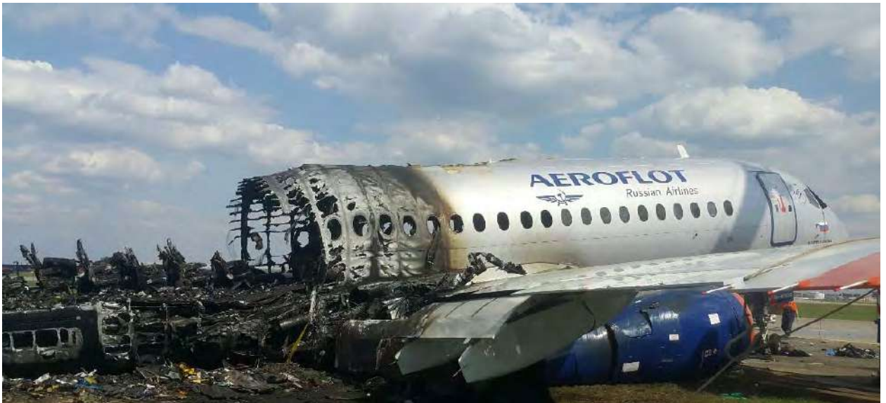
Fig. 10. External view of the fuselage front part after the accident
