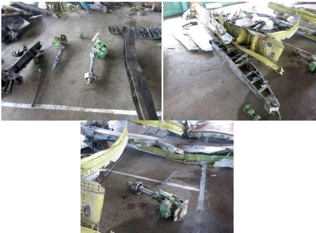
**Fig. 6. Jackscrews and single unit tracks**
