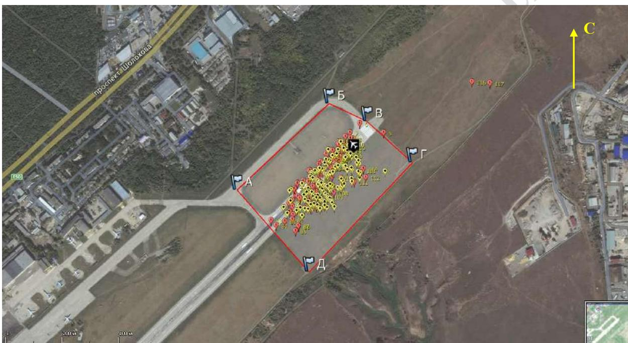
**Fig. 39. The pattern of the wreckage scatter on the accident site**
