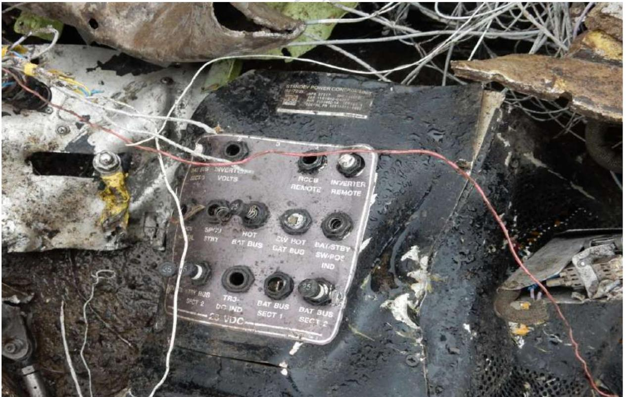
**Fig. 19. The standby power control unit**
