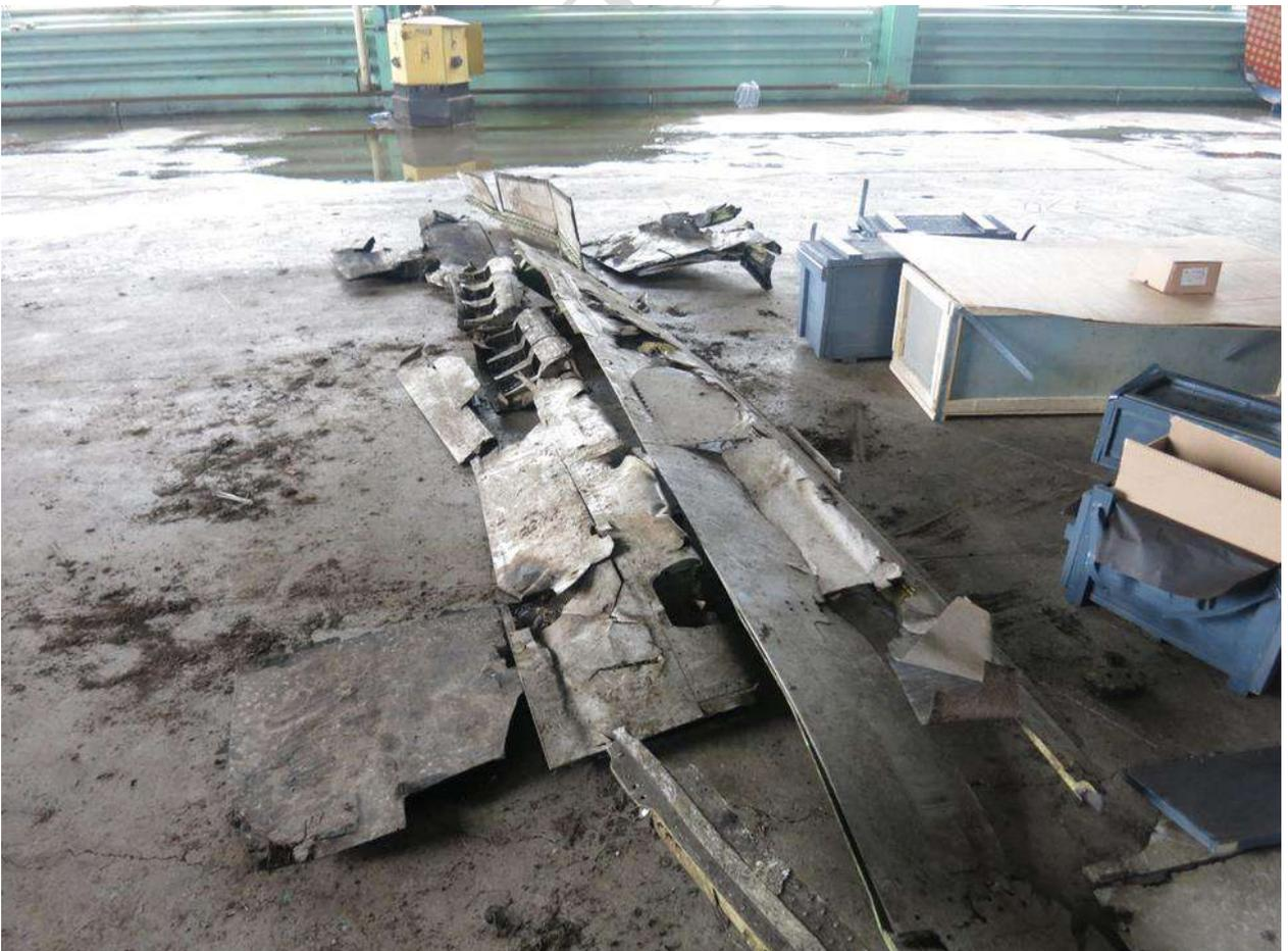
**Fig. 5. The fragments of the LH wing panel**
