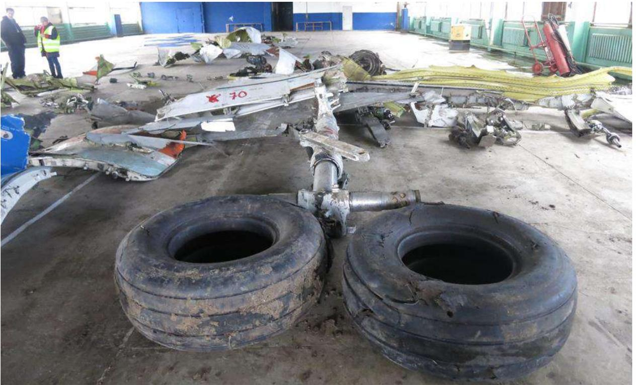
**Fig. 9. The elements of the right main landing gear leg**
