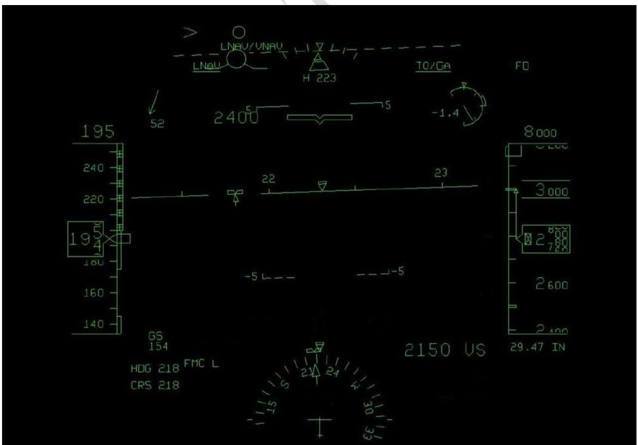
Fig. 68. The HUD reconstructed image at the point of time of 00:41:19 (the pitch command bar local maximum  $\approx 13^\circ$ )
