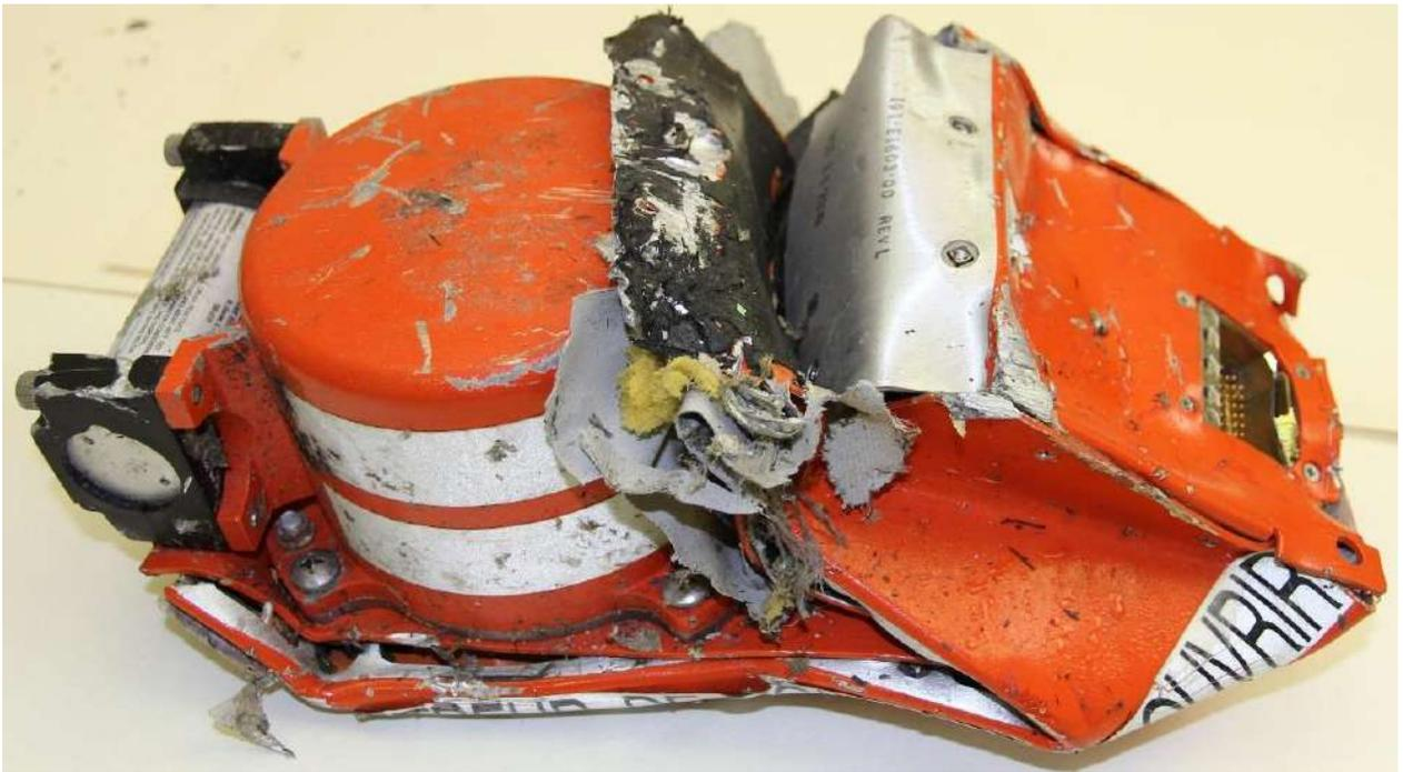
**Fig. 36. The external view of the CVR**
