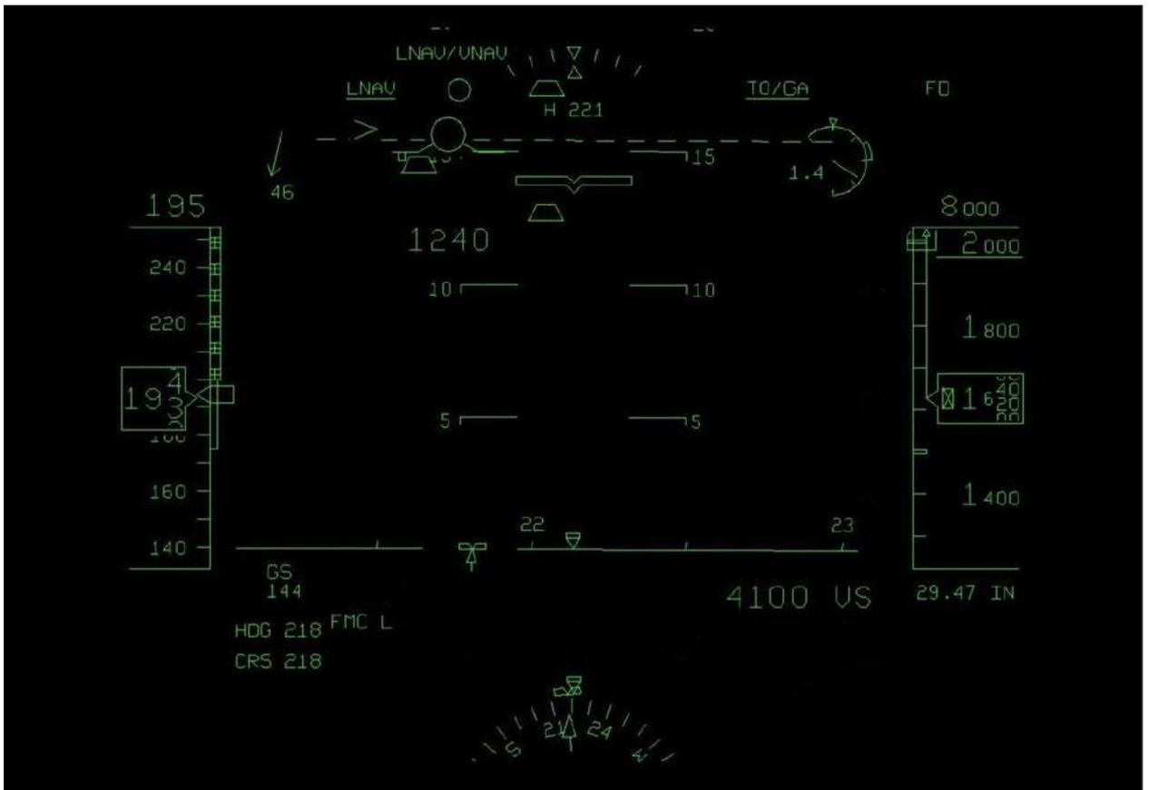
Fig. 65. The HUD reconstructed image at the point of time of 00:41:03 (the pitch local maximum  $\approx 14^\circ$ )
