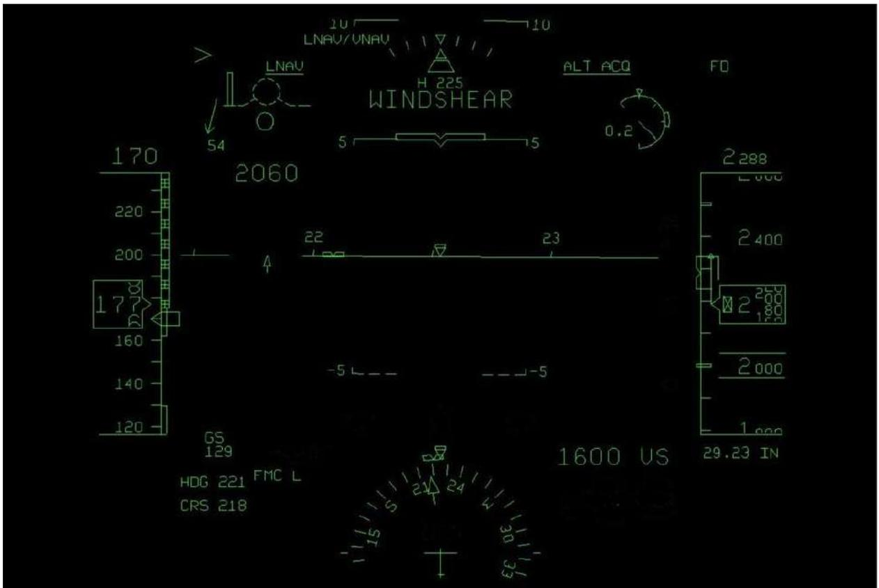
**Fig. 60.** The HUD reconstructed image at the point of time of 22:42:31.5 (the last press on the stabilizer trim switches)
