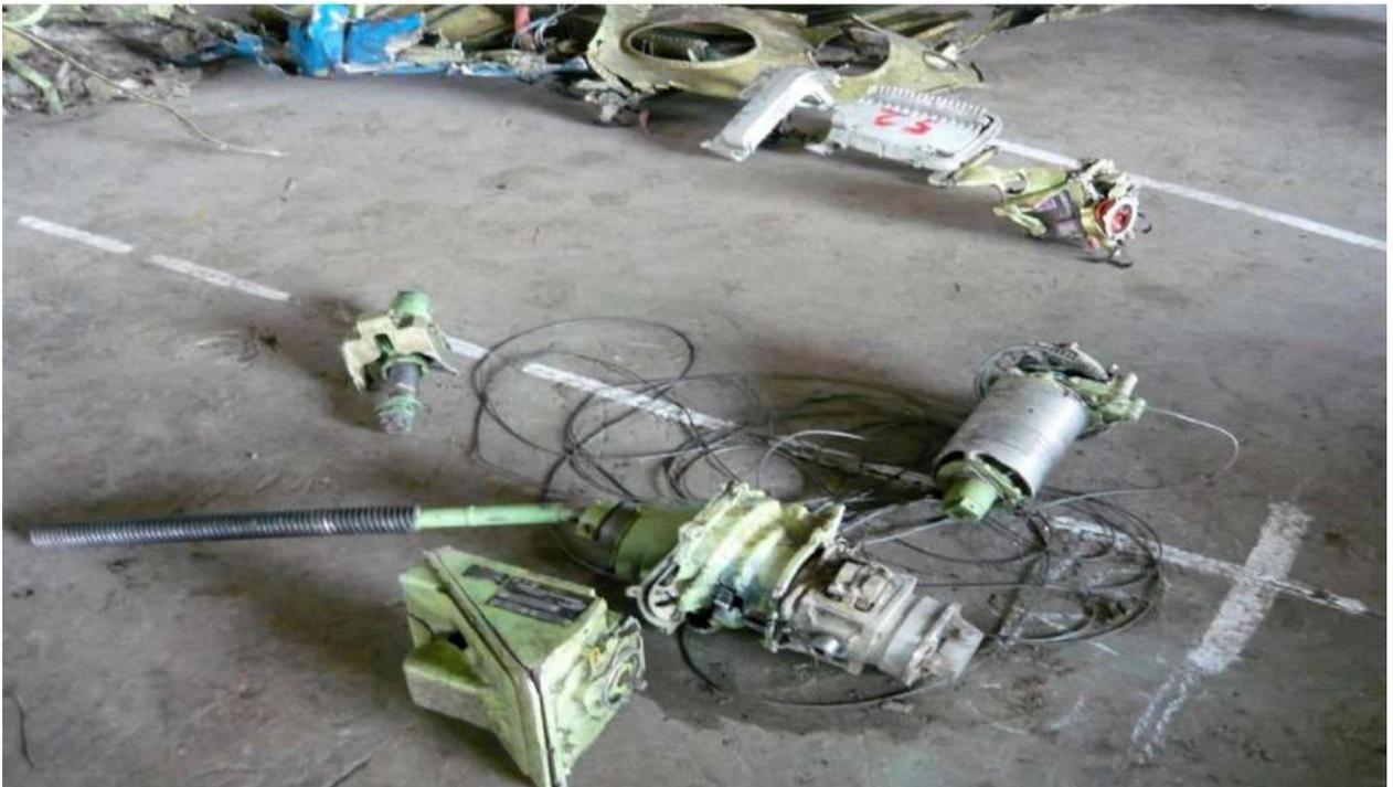
**Fig. 12. The recovered elements of the stab trim actuator**
