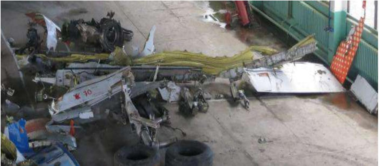
**Fig. 4. The fragments of the RH wing panel**
