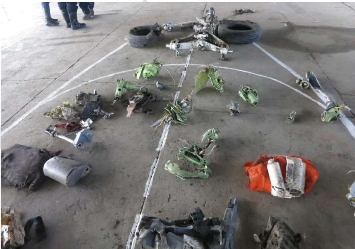
**Fig. 3. The elements of the elevator, ailerons and rudder control systems, mounted in the cockpit underfloor compartment**
