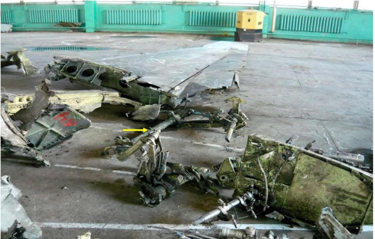
**Fig. 11. The elevator control system output shaft (pointed with arrow)**
