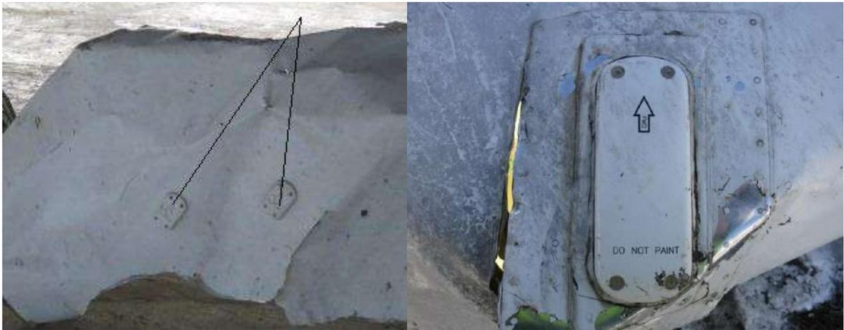
**Fig. 26. The GPS and TCAS antennas**
