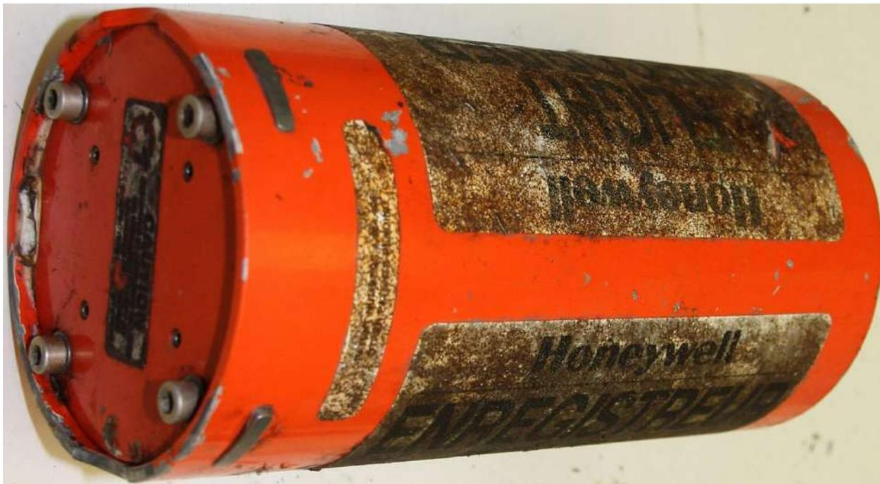
Fig. 35. The FDR secure memory unit
