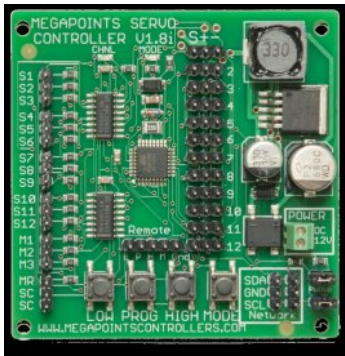
4c. The Megapoints Servo Controller 12 drives up to a dozen servos ($8.80 per servo). See: megapointscontrollers.co.uk/product/servo-controller-12
