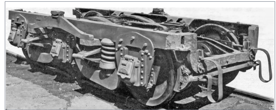
9. This Pullman six-wheel truck from the early heavyweight period utilized a one-piece cast frame with separate bolted-on pedestals. The looped strap-springs mounted on the dropped end sill support the floating brake beam.
