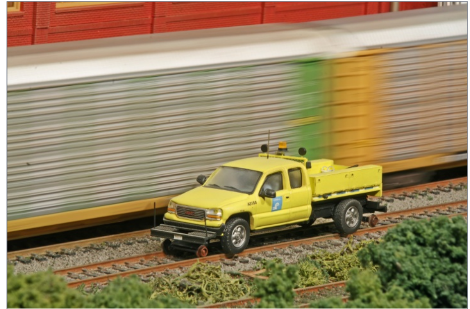
20. A hi-rail inspection truck drives along the rails at Cranford as eastbound auto rack 18N rushes past at track speed. Once the domain of speeder cars, track inspection is now performed in special trucks equipped with hi-rail wheels that enable them to operate on both rail and road.
