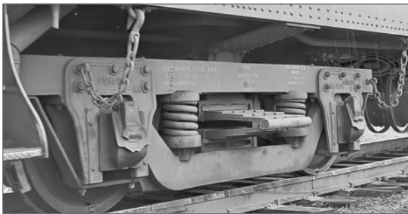
13. A heavy tie bar from the corner of the truck frame to the bottom of the pedestal helped stabilize bolt-on pedestals.
