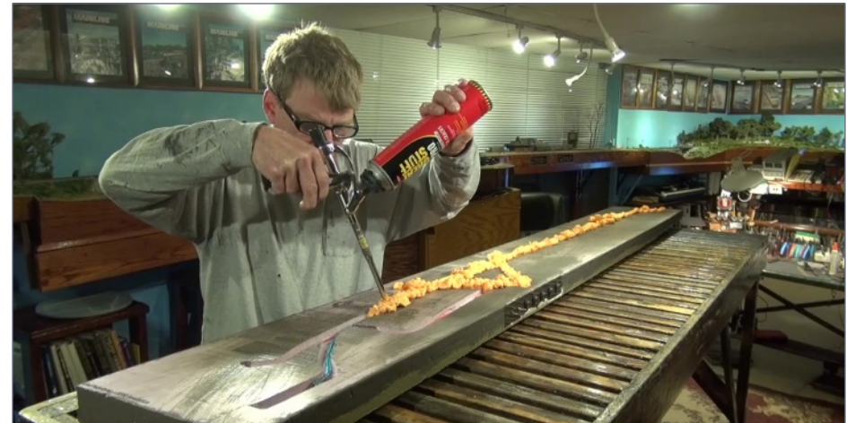
15. Ken uses Great Stuff Pro foam to fill in the wire tracks on the bottom of the layout. This keeps the wires out of the way and ensures that they won't catch on anything when the layout is moved.
