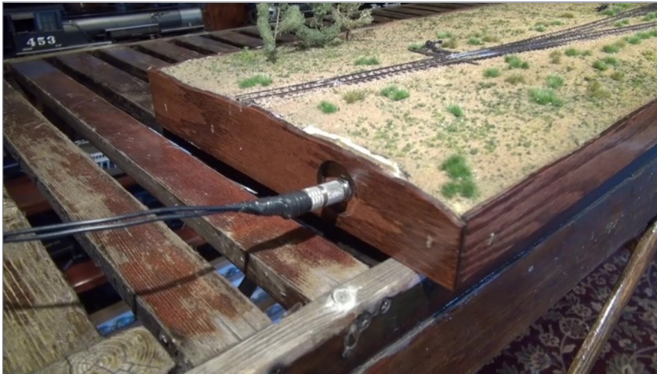
13. External power comes from a 1/4" microphone jack installed in the end of the layout.
