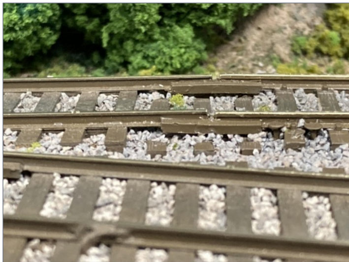
2. This vertical kink caused longer-wheelbase locomotives to derail.
