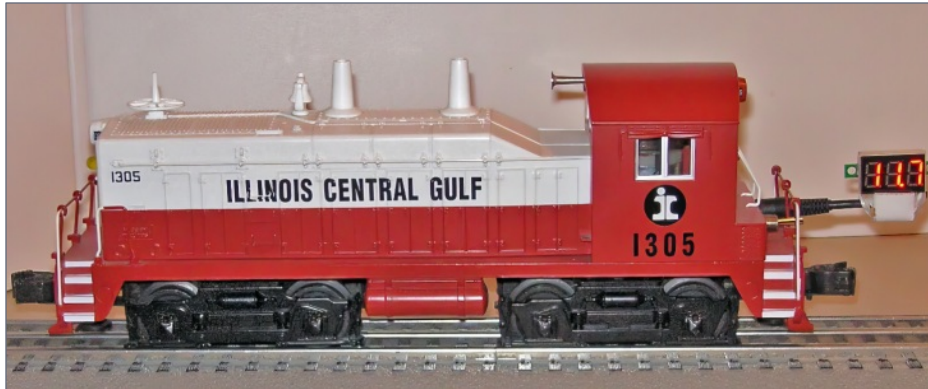
4. Our NW2 test unit with the voltage monitor at far right.
