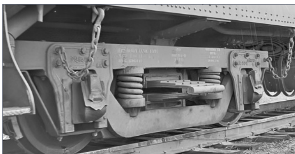
12. This six-wheel truck features individual cast pedestals bolted to the steel-clasped wood frame. Details include slender drop equalizers with coil springs, pedestal stabilizing bars below the equalizers, and car side-bearings. This truck was produced by Barney & Smith in the 1880s.
