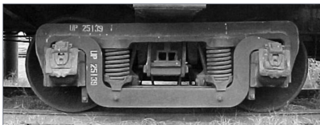
17. Outside drop equalizer on a heavyweight Union Pacific truck with plain journal bearings.
