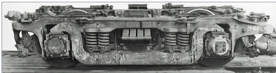
19. Pennsylvania Railroad class 2D-P7 four-wheel truck with outside drop equalizers was used on the Fleet of Modernism cars built in 1938. Due to clearance issues, some air brake cylinders were mounted on the end sill rather than on the side of the truck.
