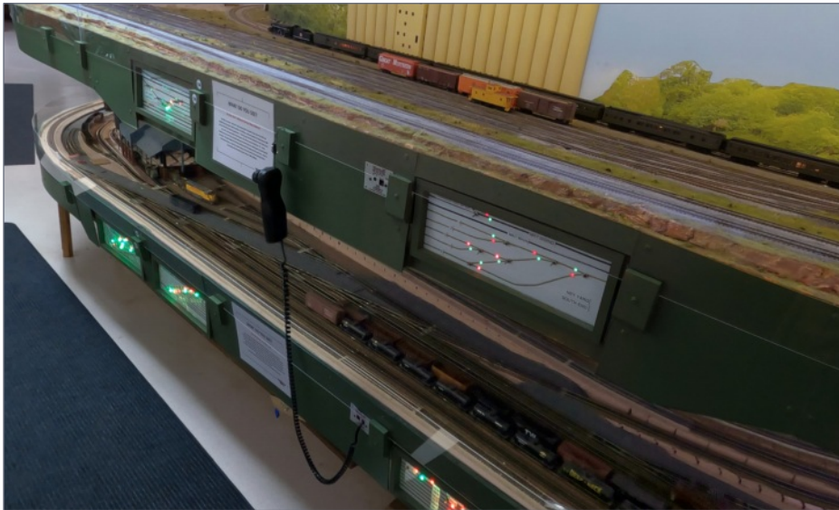
10. The club spent multiple years installing Tortoises and adding panels to control the turnouts across the layout, as seen in this view.
