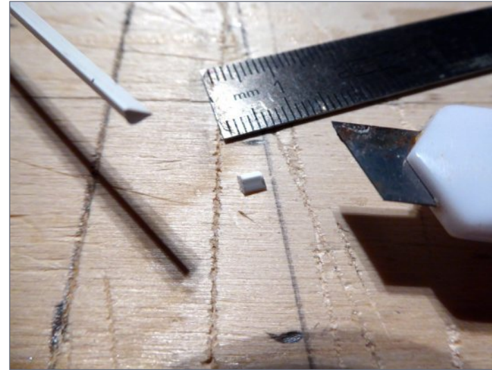
13. I cut triangular pieces from 3/32" square styrene by splitting it down the middle.
