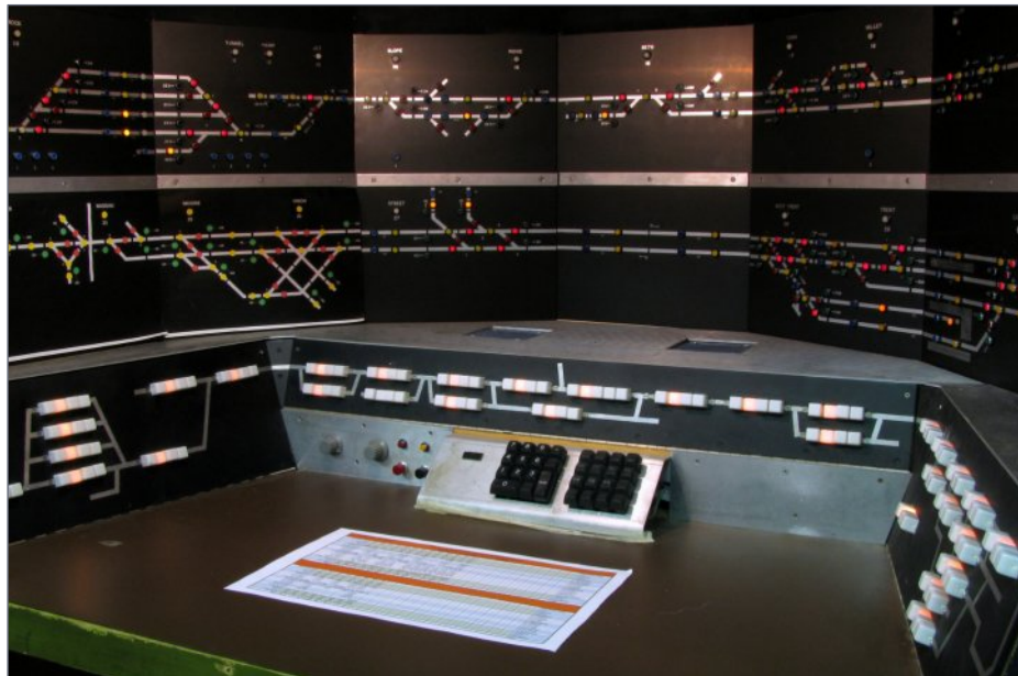
6. The Trenton Northern's Dispatcher's panel. The wrap-around design makes all the displays easy to see and the controls easily accessible.
