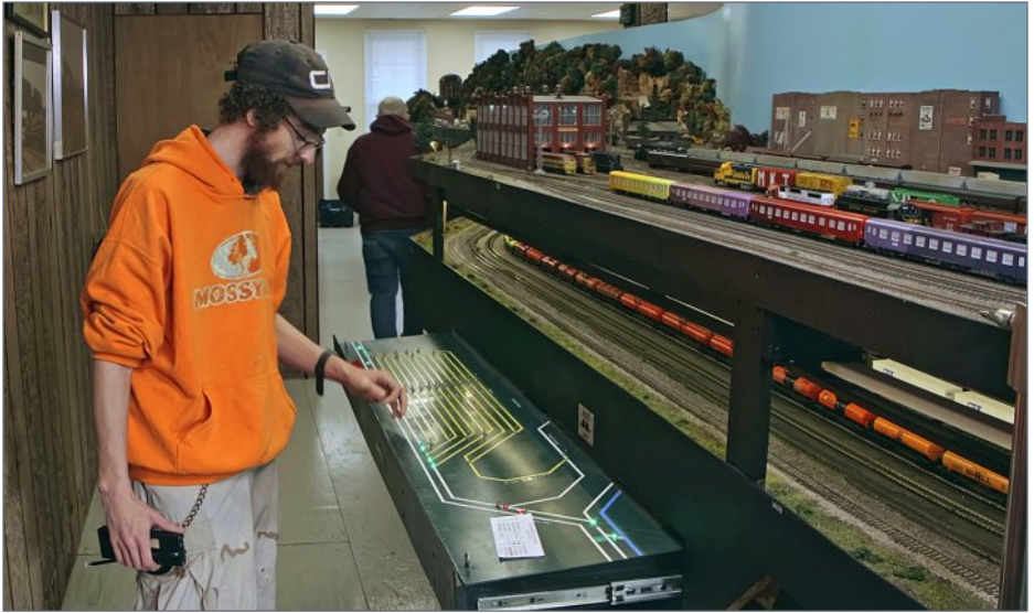
20. Club member Jake Dillam demonstrates one of the club's "hidden panels" pullout drawer-slide control panels for controlling the staging track turnouts and track power.
