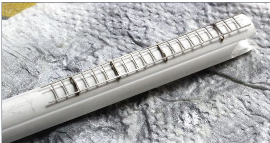
25. I drilled #75 holes into the half-inch tube and mounted the two pieces of ladder.
