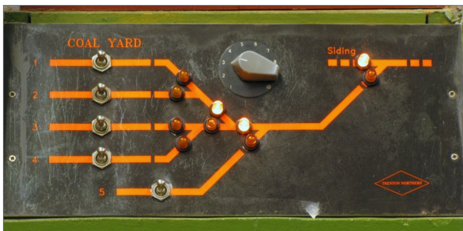
3. This TN panel controls access to the coal yard.
