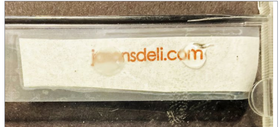
12. RapidFuse Ultra Clear dries clear (right drop), when compared to regular CA (left drop). Yes, I was eating a Jason's Deli Meatball Sub at the time of this test.
