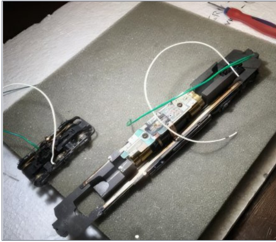
6. Green wire leads from right rail pickups and white wire leads from left rail pickups.
