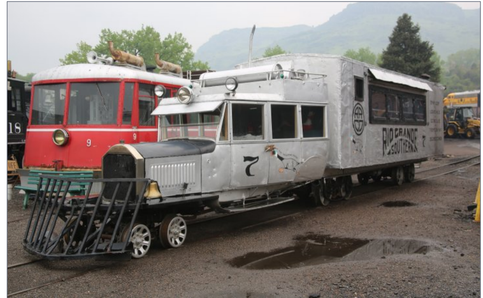
3. RGS motor car no. 7, one of the famed Galloping Geese, at rest on one of the roundhouse tracks. Originally built for mail and light passenger duty, the car featured a Pierce-Arrow limousine chassis mated with a boxcar. As mail duty gave way to tourist duty, the railroad cut windows into the box.
