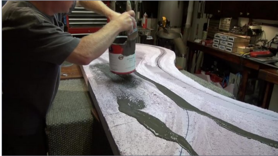
4. To seal the foam, Ken paints the entire layout with brown house paint.
