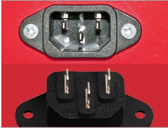
11. Front, outside view (top) and back, inside view (bottom) of the IEC C14 chassis mount connector (item 11, parts list). From the inside view, the black wire from the power strip connects to the left post (live),
