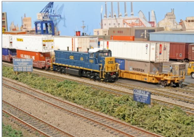
16. CSX 1301, a brand new genset locomotive, works Portside yard job YPPN-06, pulling a cut of westbound cars from the intermodal terminal. Genset locomotives use multiple self-contained diesel gensets on a
