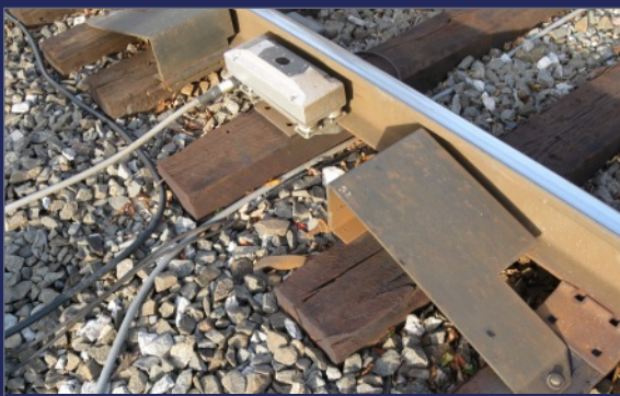
7. Closeup of an axle heat sensor.
