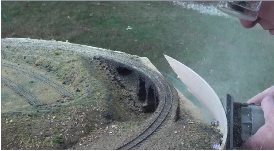
8. Ken uses a laminate trimmer to sculpt the edges of the fascia to match the dips and rises of the layout scenery. He'll finish it off with a sander to smooth the edges.
