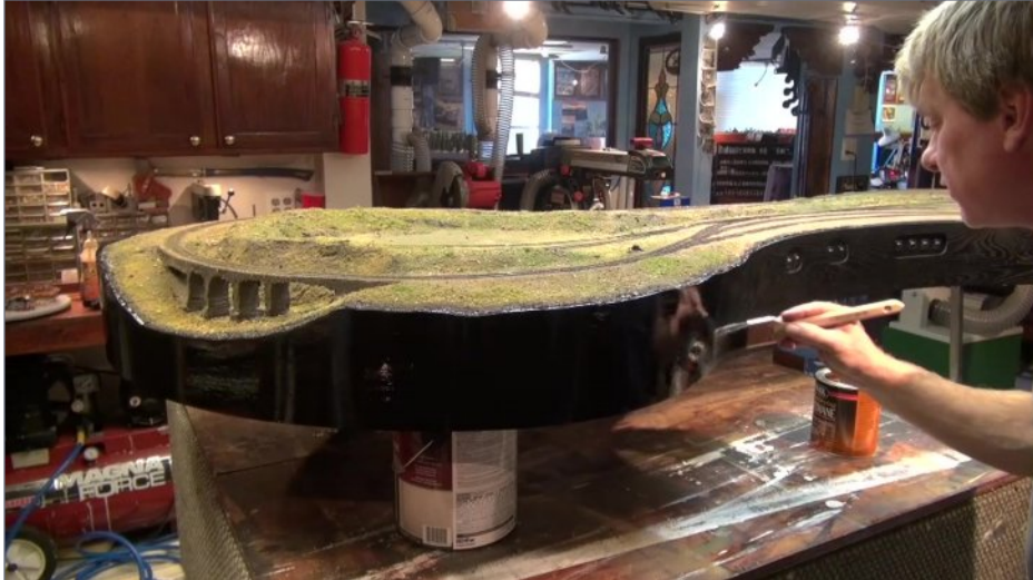
9. Ken applies two layers of a Floquil and Minwax stain mixture, and then finishes off the fascia with three layers of polyurethane gloss.
